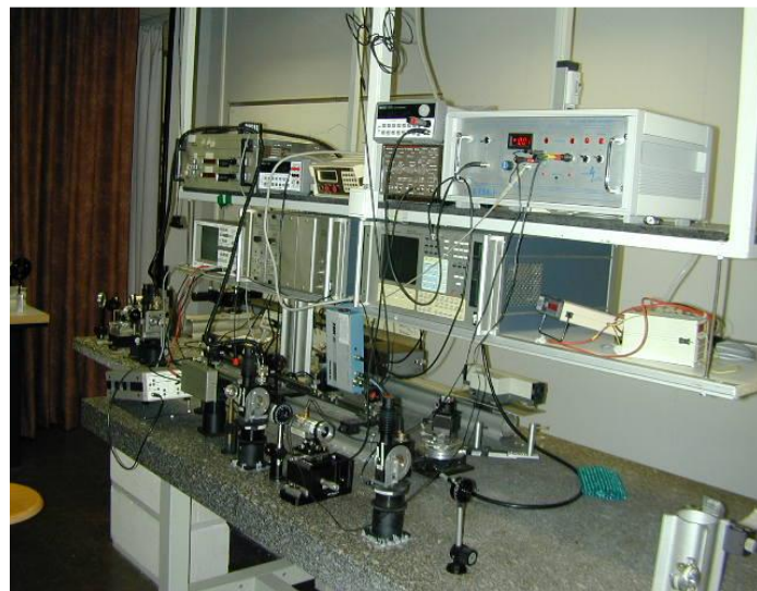
Figure 3.1.1.1.2: The Senarmont compensation one-beam ellipsometric setup (LMOPS laboratory).
