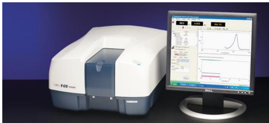
Figure 2.3.1.1: Scheme of the Jasco V670 spectrophotometer used for optical absorption measurements. It is a double beam spectrophotometer operating in a wide range of wavelengths from 200 to 3200 nm. It is equipped with two lamps (deuterium lamp from 190 to 350 nm, halogen lamp from 330 to 3200 nm), a dual-grating monochromator, two detectors (a photomultiplier tube and a Peltier-cooled PbS detector). It is equipped also with an optional rotating sample holder, and an optional polarizing window made of a Glan-Taylor calcite prism.
