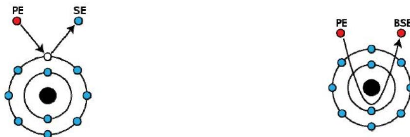
**Fig.21:** Interactions between primary electrons (PE) and the atoms of specimens leading to the formation of secondary electrons (SE) and backscattered electrons (BSE) [175]
