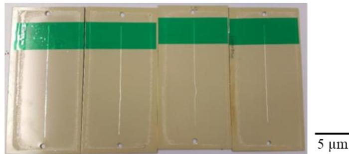
**Fig.115:** Appearance of the pulse Zn-Mn deposits (100 x 200 mm samples) after application of the phosphate conversion layer and the electrophoretic coating (E-coat); samples as prepared for the cyclic corrosion test (VDA 233-102) with scribe
