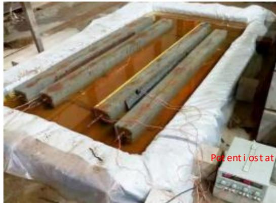
**Fig. 3.2. Accelerated corrosion device**
