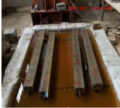
**Fig. 4.7. Accelerated corrosion device**
