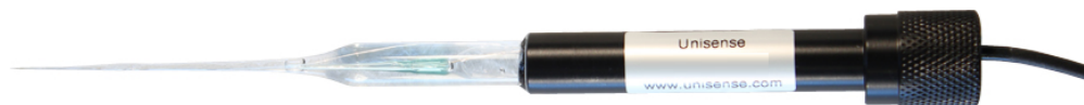
Figure 3.16 – Unisense oxygen microsensor employed to collect the oxygen concentration data. Picture taken from Unisense website .
