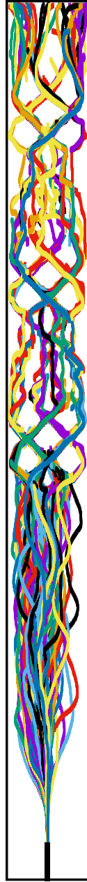
Figure 7.15 – Trajectories of bubbles registered in the bubbles column with the 5 elements SMX fed by d_n = 1 mm. Gas flow-rate Q_G = 11/h . Coloured according to bubble ID.
