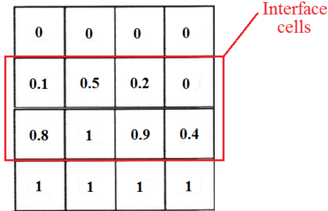
Figure 5.3 – Tracking of the interface in the VoF model.
