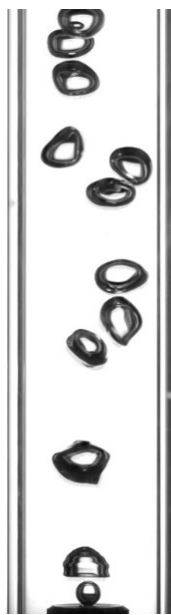
Figure 3.4 – Detailed view of the bubbles' generation with a flat orifice (diameter = 1 mm). Nitrogen/water system. Gas flow rate : 2.5 l/h.
