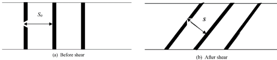
Figure 2.17 – Striation thickness under simple shear. Taken from Thakur et al. (2003) [2].
