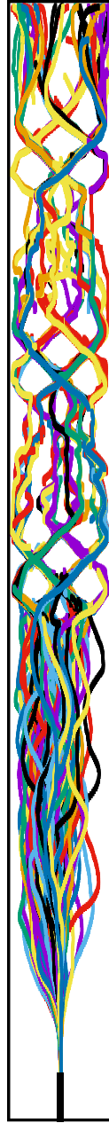
Figure 7.15 – Trajectories of bubbles registered in the bubbles column with the 5 elements SMX fed by d_n = 1 mm. Gas flow-rate Q_G = 11 /h. Coloured according to bubble ID.
