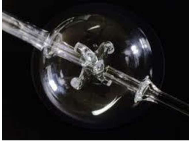
Figure 34. Picture of a jet-stirred reactor. The cross shaped nozzle can be seen in the center of the reactor.
