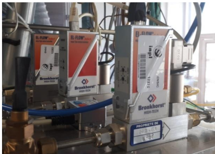
Figure 33. Picture of the three mass flow controllers installed on the set-up.
