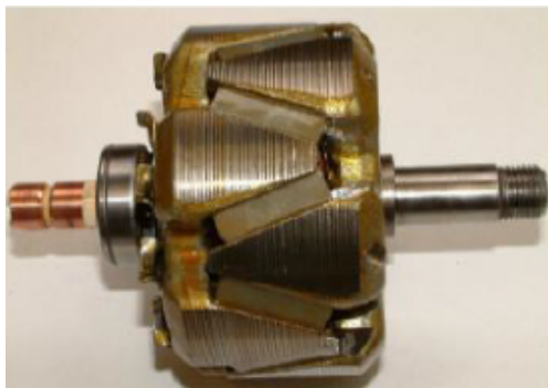
Figure 1.22. Photo of an example of a claw pole rotor.
