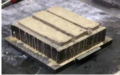
Fig. VIII.5. Prismatic mortar test (4*4*16) manufactured to test the characteristics of the considered formulation of manufactured mortar.
