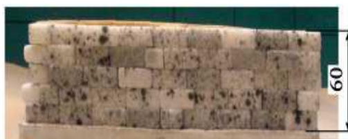
Fig. II.29 Model combining silicone foundation and sugar block structural element.
