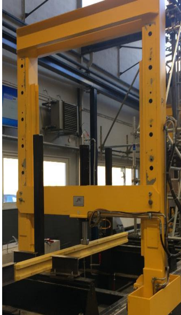
Fig. VIII.12. Bending test for the wooden beam.
