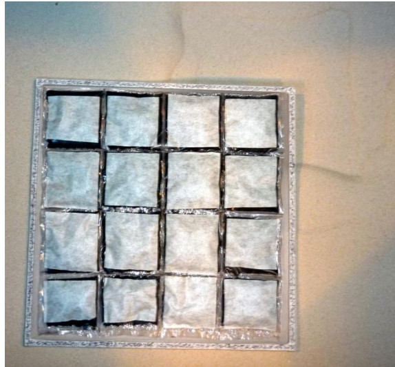
Fig. II.28 The model polycarbonate tray type with overloading of lead balls placed in small bags to ensure good load distribution during testing.
