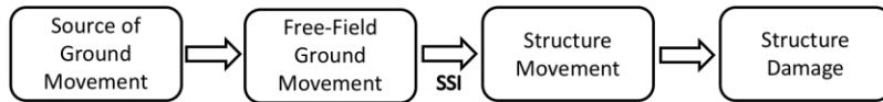
Fig. VIII.1. Diagram representing the ground movement transmission to the structures due to Soil-Structure Interaction (SSI).
