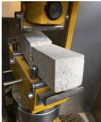
Fig. VIII.6. Bending and compression tests of mortar specimen.
