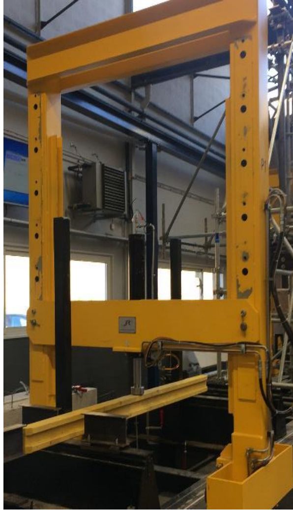
Fig. VIII.12. Bending test for the wooden beam.
