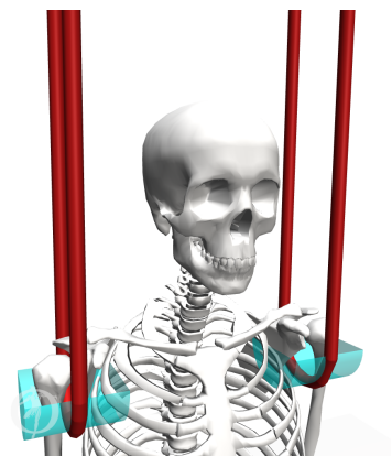
Figure 3.6: Connection of the elastic harness.
