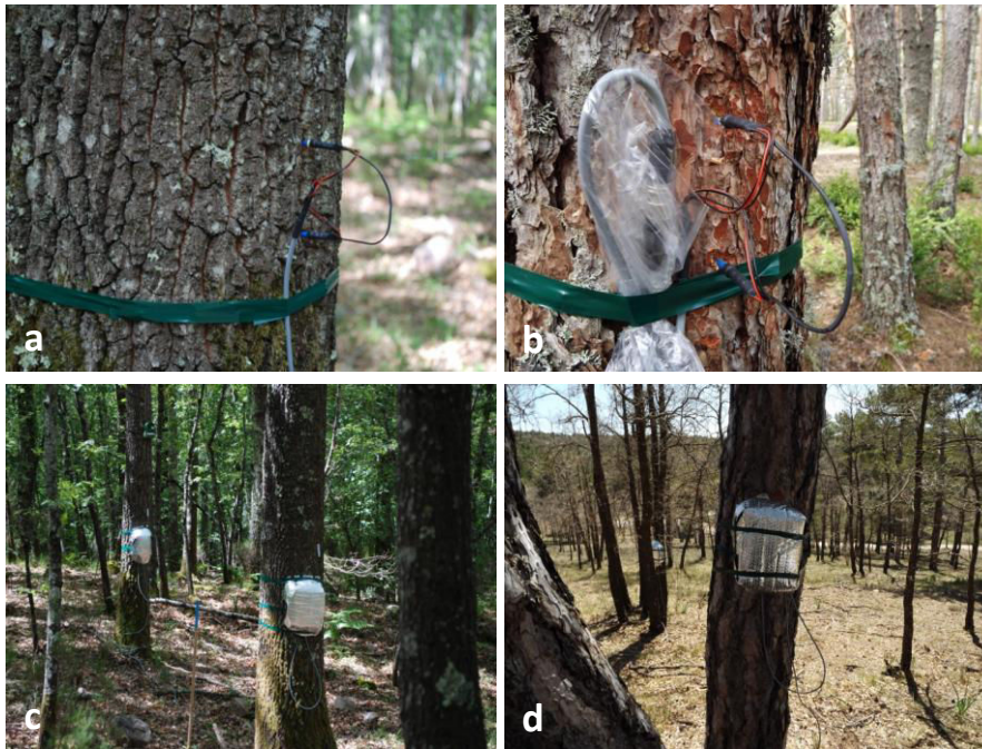
Figure 5: (a) Sap flux sensor insertion into the trunk of a Quercus cerris tree in the thermophilous deciduous forest in Italy (June 2012) and (b) into a Pinus sylvestris tree in the Mediterranean broadleaved-coniferous forest in Spain (May 2013). (c) Two Quercus cerris trees in the thermophilous deciduous forest in Italy (June 2012) and (d) two Pinus nigra
