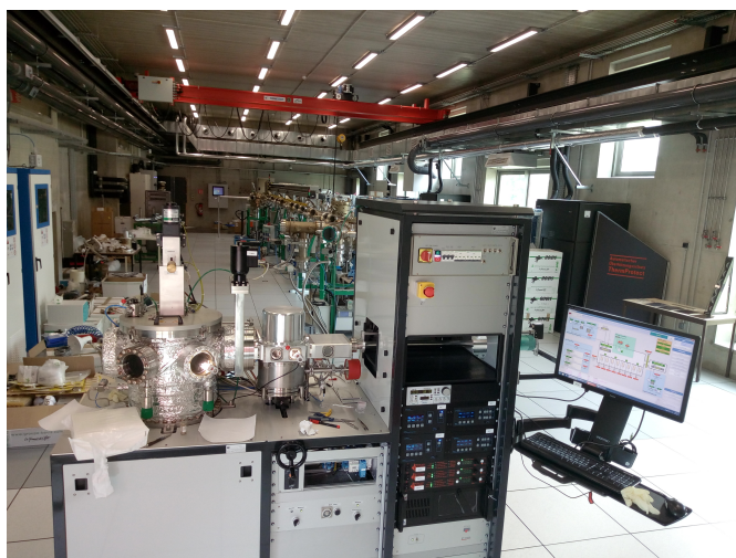
Figure II.2: Sputtering system developed by Vinci Technologies for the Institut Jean Lamour.
