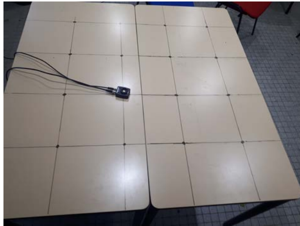
Figure 6.25: Photodetector receiver in the testing grid for CPP VLP method validation
