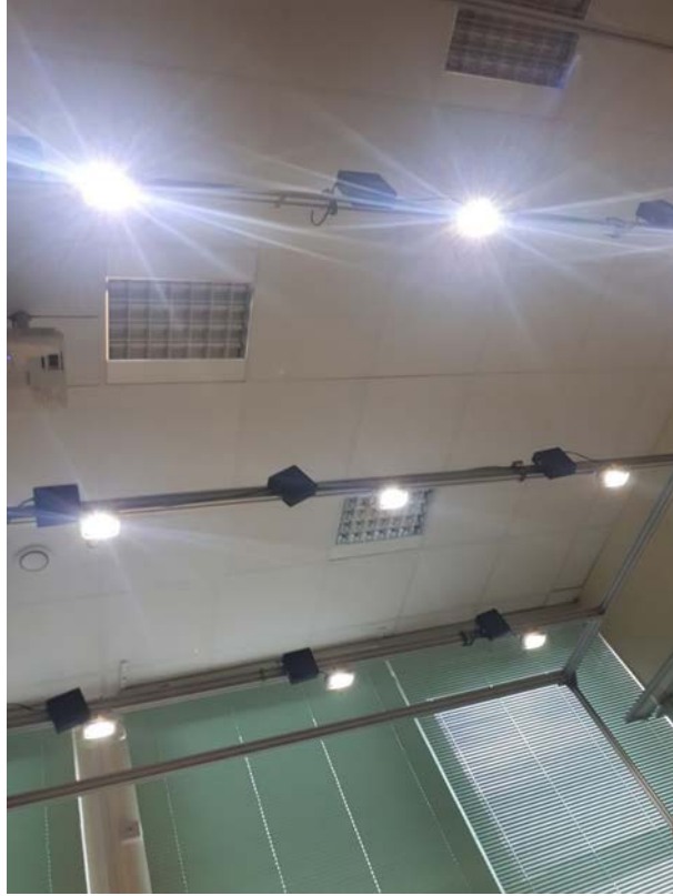
Figure 6.24: Real square room VLC platform for VLP testing
