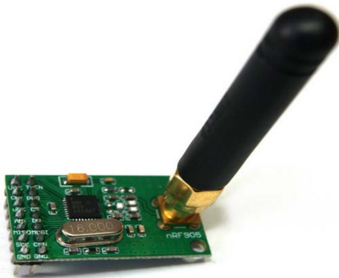
Figure 5.1: Single chip transceiver nRF905
