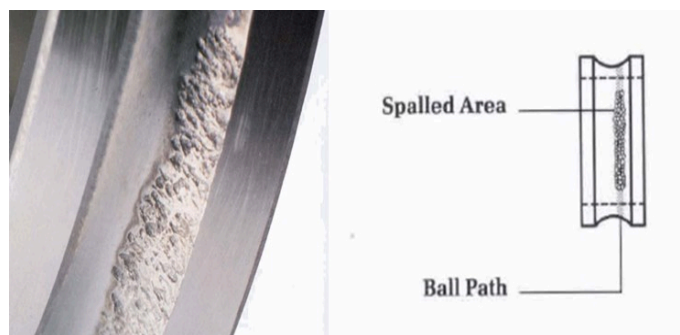
Figure 1.3 Severe spalling and its location of ball bearing [10].
