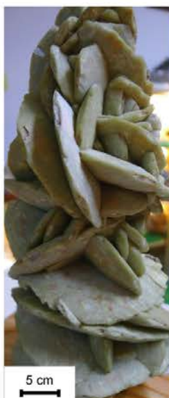
Fig. 3.13: Siderite stage is at the origin of the formation of euhedral large siderite crystals in cavities, the crystallization of xenomorph isolated crystals in the quartz veins, and some crystals at the boundary between host-rock and earliest veins in the cavities created by the muscovite-arsenopyrite stage. Siderite crystallizes onto quartz IV euhedral crystals, and is then covered by chalcopyrite crystals in geodes.
