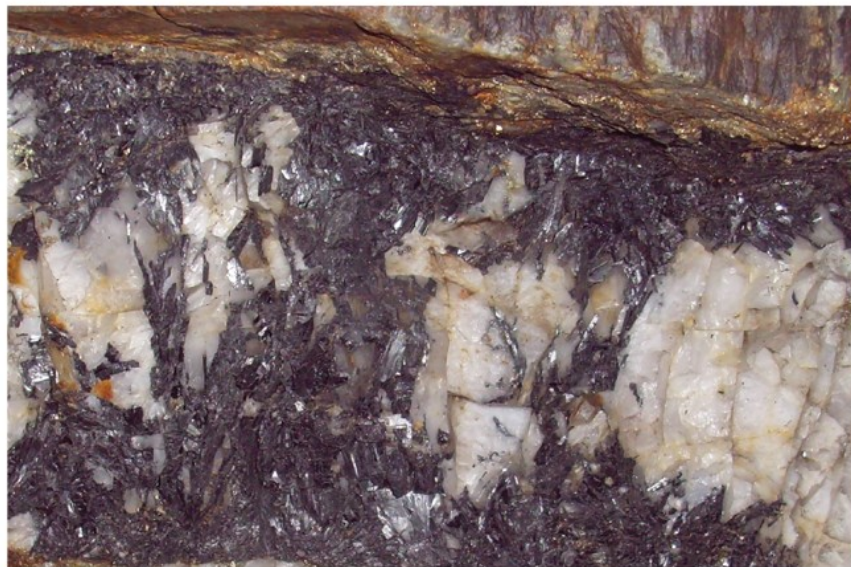
Fig 3.3: The earliest vein infilling: wolframite followed by quartz QI, which represent more than 90 % of the vein infillings observed in galleries.
