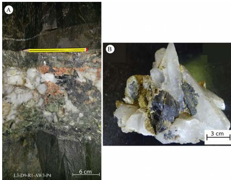
Fig. i-8: A- Quartz vein at the pillar scale showing the stage IV of the paragenetic sequence. B- Larger crystal size concentrated in the vugs
