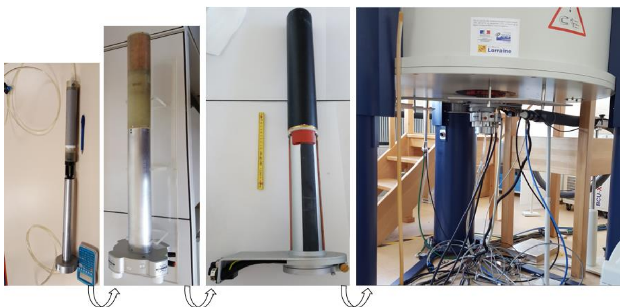
Figure A.2. MRI probe in combination with the Gradient System and the holder with PVC tube sample
