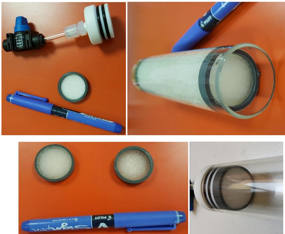
Figure A.5. Sample components, filters and caps.
