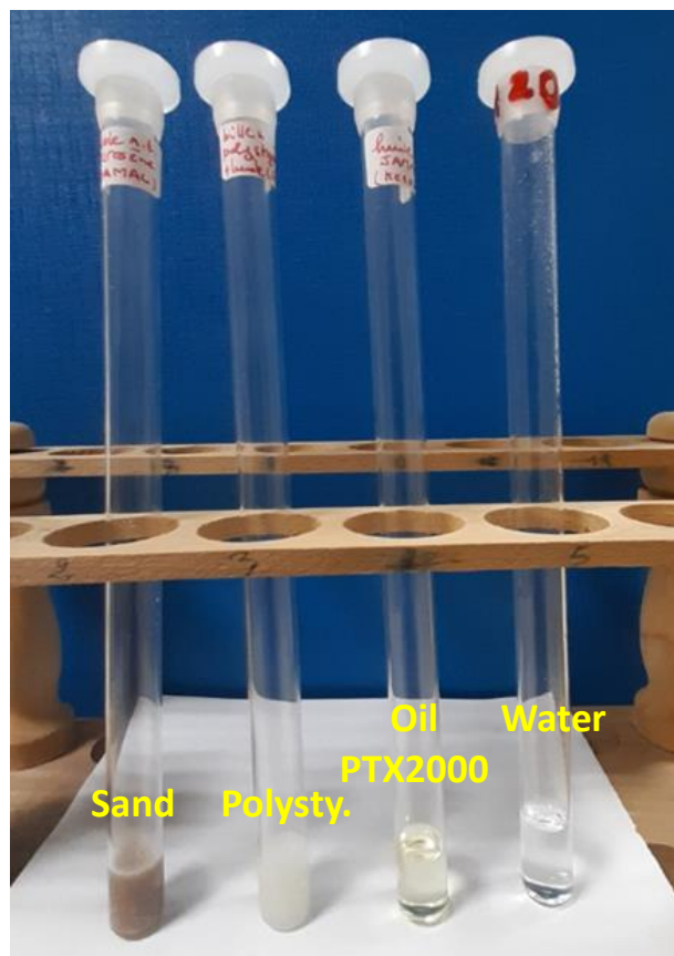
Figure A.13. Samples used to measure T2 relaxation time; pure water, pure oil (PTX2000/Kerosene), sand with water/oil and polystyrene with water/oil. The sample tube internal diameter is 0.878 cm and the height of substances is around 12 mm, the total tube height is 12 cm.
