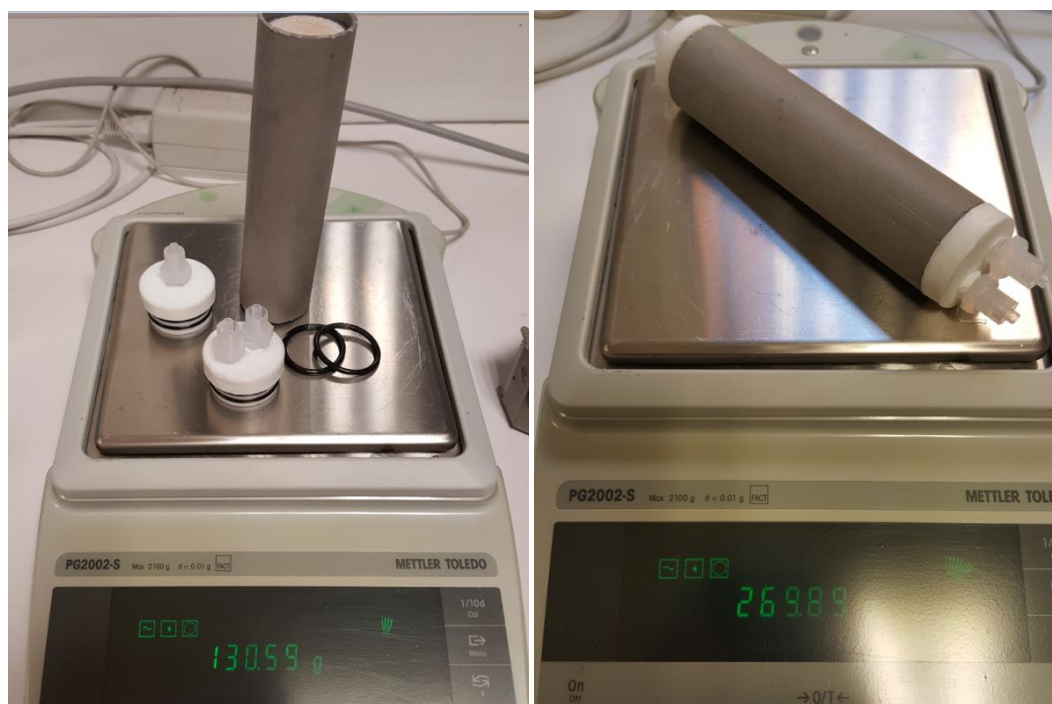
Figure A.6. PVC sample and its components (10 cm of the final net length), the weight with and without sand.
