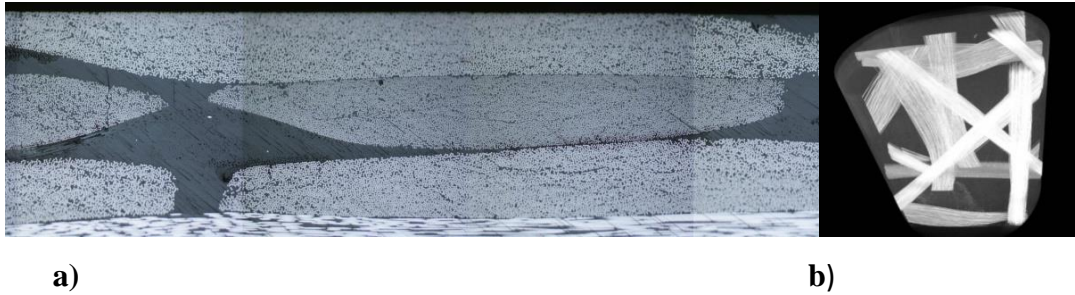
Figure 2: Upper part of the [-45/90/45/0]_s quasi-isotropic laminate: a) optical micrograph of the edge view; b) spatial distribution of stitch yarns obtained from micro computed tomography.
