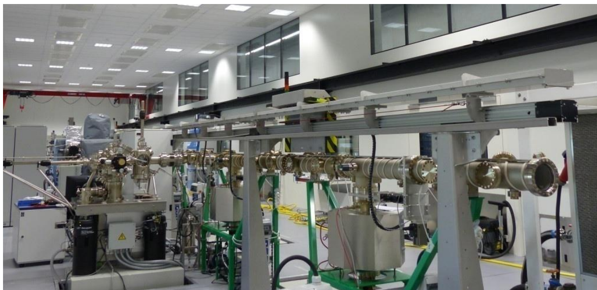
Figure 62 : Tube DAUM ultravide
