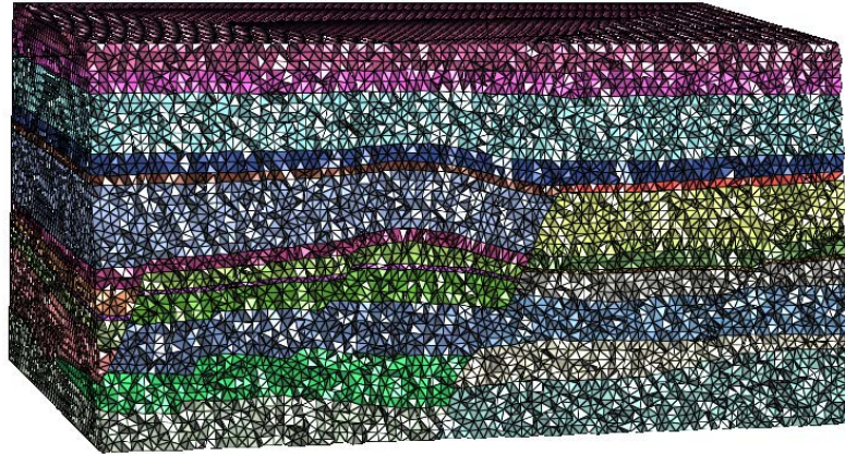
Figure III.9 – Cross-section view of the volumetric model with a resolution of 50 m. The different geological entities, which are the blocks delimited by the faults and horizons, are underlined with different colors.
