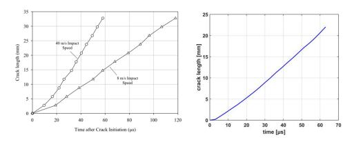
Figure 2.23: Crack length evolution with time: (a) experimental results [17] vs (b) numerical results.
