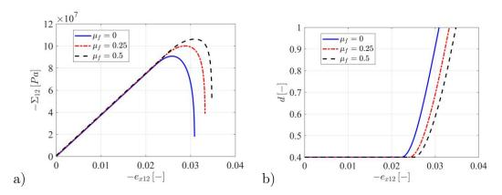
Figure 3.6: Stress  $-\Sigma_{12}$  and damage d vs strain  $-e_{x12}$  for three values of the friction coefficient:  $\mu_f = 0$ ,  $\mu_f = 0.25$  and  $\mu_f = 0.5$ .
