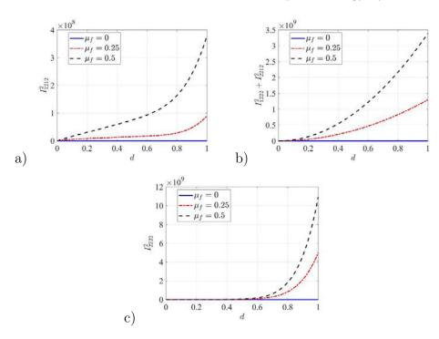
Figure 4.6: Components  $I_{1212}^2$  (a),  $I_{1222}^2 + I_{2212}^2$  (b),  $I_{2222}^2$  (c) of  $I_{mnpq}^2$  vs damage variable d, for  $\mu_f = 0$ , 0.25, 0.5.
