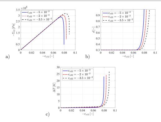
Figure 4.10: Effective stress  $\Sigma_{12}$ , damage variable d and temperature variation  $\Delta T$  vs. the strain  $e_{x12}$ , for different compressive strains:  $e_{x22} = -5 \times 10^{-3}$ ,  $e_{x22} = -2 \times 10^{-2}$ ,  $e_{x22} = -3.5 \times 10^{-2}$ .
