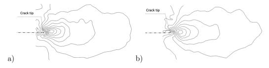
Figure 3.14: Lines of constant shear stress  $\Sigma_{12}$  at: a)  $40 \,\mu s$  and b)  $60 \,\mu s$ . The absolute values of  $\Sigma_{12}$  are increasing when approaching the tip of the damage band.
