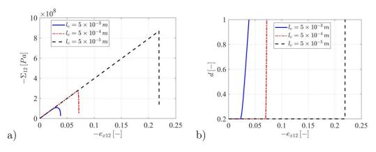
Figure 3.9: Stress  $-\Sigma_{12}$  and damage d vs strain  $-e_{x12}$  for micro-structural lengths:  $l_c = 5 \times 10^{-3} \, m$ ,  $l_c = 5 \times 10^{-4} \, m$  and  $l_c = 5 \times 10^{-5} \, m$ .
