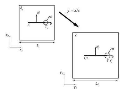
Figure 4.2: Scaling of the microscopic period  $B_{\varepsilon}$  with a crack C into the reference cell Y with the crack CY. The unit vectors  $\mathbf{n}$  and  $\mathbf{e}$  indicate the normal to the crack-tip contours  $\Gamma_r$  and  $\Gamma Y_r$  and, respectively, the propagation direction.
