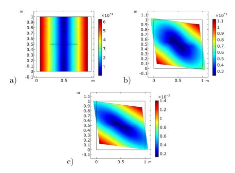
Figure B.1: Displacements  $\mathbf{v}^{11}$  (a),  $\mathbf{v}^{12}$  (b) and  $\mathbf{v}^{22}$  (c) obtained from FE unit cell computations.
