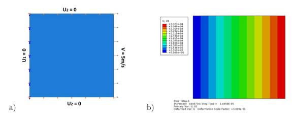
Figure 2.15: One-element test: a) boundary conditions and b) displacement  $u_1$ .
