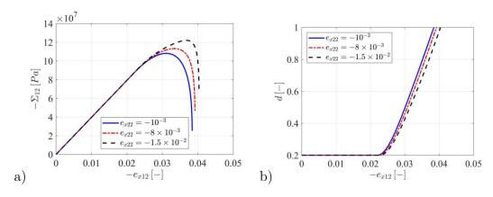
Figure 3.7: Stress  $-\Sigma_{12}$  and damage d responses for three values of the compressive strain.
