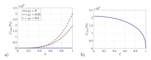
Figure 3.4: Effective moduli  $C_{1222}(d)$  and  $C_{1212}(d)$  for three values of the friction coefficient:  $\mu_f = 0$ ,  $\mu_f = 0.25$  and  $\mu_f = 0.5$ .
