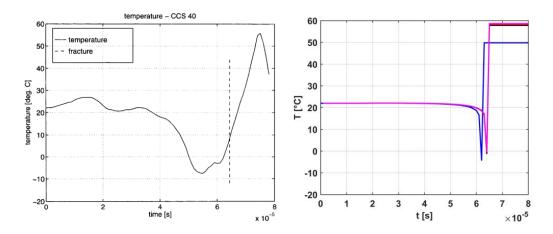
Figure 2.14: Temperature variation at 1 mm from the tip of the notch: measured values (left) from [115] and computed values (right) in 4 neighbor elements in the area of the thermocouple location.
