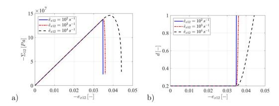
Figure 3.8: Stress  $-\Sigma_{12}$  and damage d response for three values of the strain rate:  $\dot{e}_{x12} = -100 \ /s$ ,  $\dot{e}_{x12} = -1000 \ /s$ ,  $\dot{e}_{x12} = -10000 \ /s$ .
