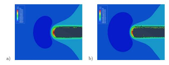
Figure 2.20: Temperature contours during the crack propagation regime: simulations with (a) and without (b) heat conduction.
