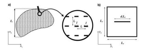
Figure 2.1: a) Micro-fissured medium with locally periodic microstructure with  $l_c$  the size of a period, l the local micro-crack length and  $L_c$  the characteristic length of the macro-structure. b) Reference cell of size  $L_c$  with rescaled crack length  $d.L_c$ .
