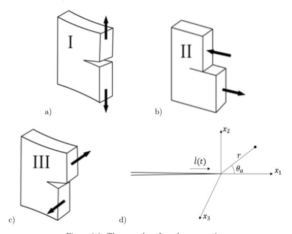
Figure 1.1: Three modes of crack propagation
