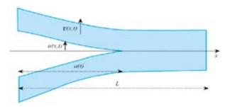
Figure 1.5: One dimensional thermoelastic fracture problem [132].
