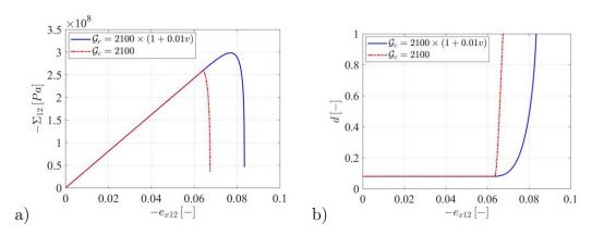
Figure 3.10: Stress  $-\Sigma_{12}$  and damage d vs strain  $-e_{x12}$ , for constant and crack-velocity dependent fracture energy.
