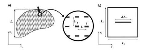
Figure 4.1: a) Solid body with locally periodic microstructure with  $l_c$  the size of a period, l the micro-crack length and  $L_c$  the characteristic length of the macro-structure. b) Reference cell of size  $L_c$  with rescaled crack length  $d.L_c$ .
