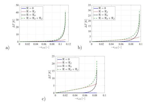
Figure 4.12: Temperature variations for different expressions of the heat source  $\mathcal{R}$  in the temperature equation (4.94), with  $\mathcal{R}_d$  and  $\mathcal{R}_f$  respectively the damage and frictional heating terms. Results are presented for a)  $d_0 = 0.3$ , b)  $d_0 = 0.5$  and c)  $d_0 = 0.7$ .
