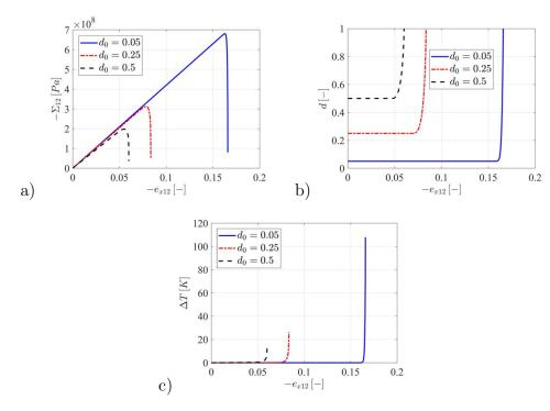
Figure 4.9: Effective stress  $\Sigma_{12}$ , damage variable d and temperature variation  $\Delta T$  vs. the strain  $e_{x12}$ , for initial values of damage  $d_0 = 0.05$ ,  $d_0 = 0.25$ ,  $d_0 = 0.5$ .
