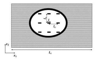
Figure 1.7: Micro-fissured medium with locally periodic distributed microcracks
