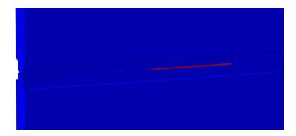
Figure 3.13: Damage band propagation inside the groove.
