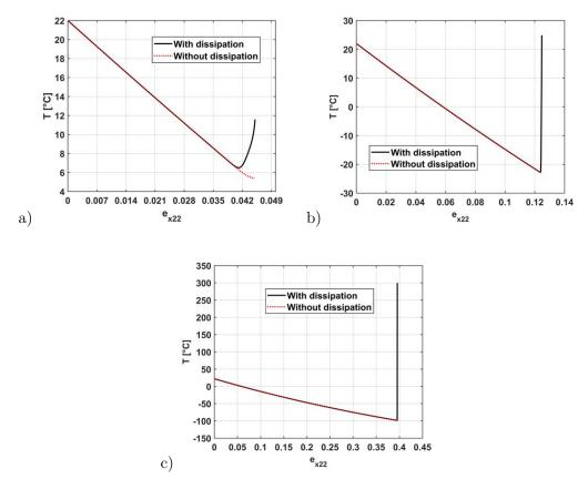
Figure 2.6: Temperature  $T^{(0)}$  versus the applied strain  $e_{x22}(u^{(0)})(t)$ , for three sizes of the microstructure: a)  $l_c = 10^{-4} m$ ; b)  $l_c = 10^{-5} m$ ; c)  $l_c = 10^{-6} m$ . Evolutions with (continuous line) or without (dotted line) crack tip heating.
