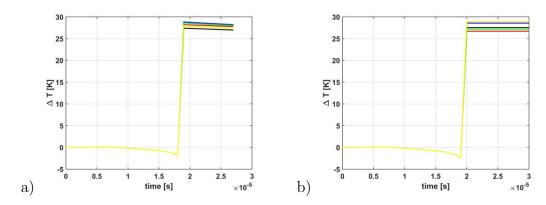
Figure 2.21: Evolutions of temperature in a point situated at a distance of  $0.6 \, mm$  from the initial notch tip.
