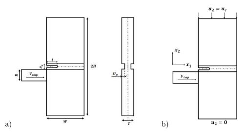
Figure 3.11: Geometry of the specimen and applied loadings: a) impact, b) impact and normal compression.
