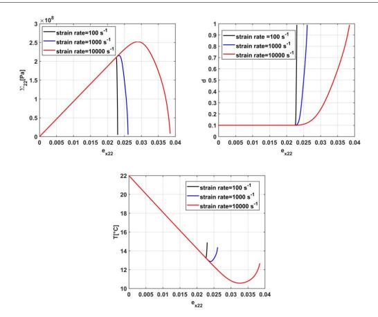
Figure 2.9: Effective stress, damage and temperature for different strain rates:  $\dot{e}_{x22} = 100 \ s^{-1}$ ,  $\dot{e}_{x22} = 1000 \ s^{-1}$  and  $\dot{e}_{x22} = 10000 \ s^{-1}$ .
