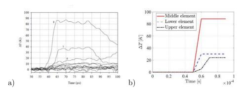
Figure 4.17: Temperature variation: measured values (a) from [19] and (b) computed values in 3 neighbor elements located in the region of IR detectors.
