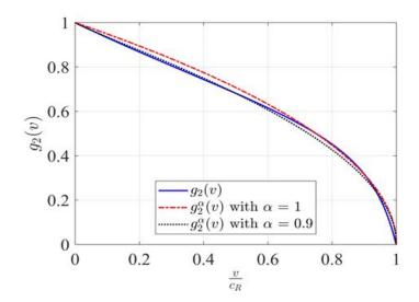
Figure 3.3: The function  $g_2(v)$  and its approximations  $g_2^{\alpha}(v)$  for  $\alpha = 1$  and  $\alpha = 0.9$ .
