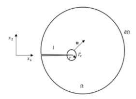
Figure 1.3: Solid with a moving crack
