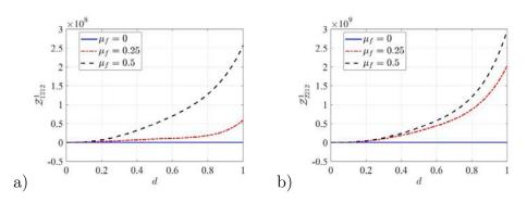
Figure 4.5: Coefficients  $\mathcal{Z}^1_{1212}$  (a),  $\mathcal{Z}^1_{2212}$  (b) vs damage variable d, for  $\mu_f = 0, 0.25, 0.5$ .
