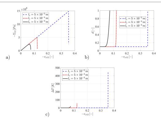
Figure 4.7: Effective stress  $\Sigma_{12}$ , damage variable d and temperature variation  $\Delta T$  vs. the strain  $e_{x12}$ , for different values of the microstructural length:  $l_c = 5 \times 10^{-5} \, m$ ,  $l_c = 5 \times 10^{-4} \, m$ ,  $l_c = 5 \times 10^{-3} \, m$ .
