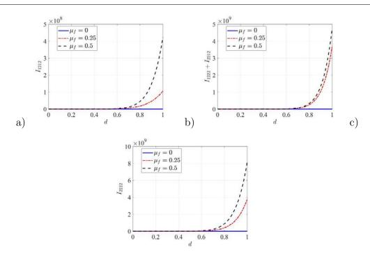
Figure 4.4: Homogenized coefficients  $I_{1212}$  (a),  $I_{1222} + I_{2212}$  (b) and  $I_{2222}$  (c) vs damage variable d, for  $\mu_f = 0, 0.25, 0.5$ .
