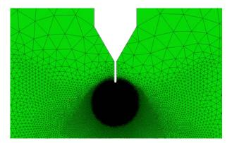
Figure 2.12: Local geometry near the notch tip and finite element mesh with refinement in the failure initiation zone.
