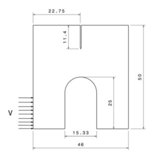
Figure 2.11: Geometry of the specimen, with dimensions in mm. The impact velocity V is applied over a region of  $16.5 \, mm$ .
