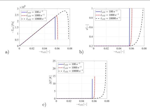
Figure 4.8: Effective stress  $\Sigma_{12}$ , damage variable d and temperature variation  $\Delta T$  vs. the strain  $e_{x12}$ , for different values of strain rate:  $\dot{e}_{x12} = -100 \, s^{-1}$ ,  $\dot{e}_{x12} = -10000 \, s^{-1}$ ,  $\dot{e}_{x12} = -10000 \, s^{-1}$ .
