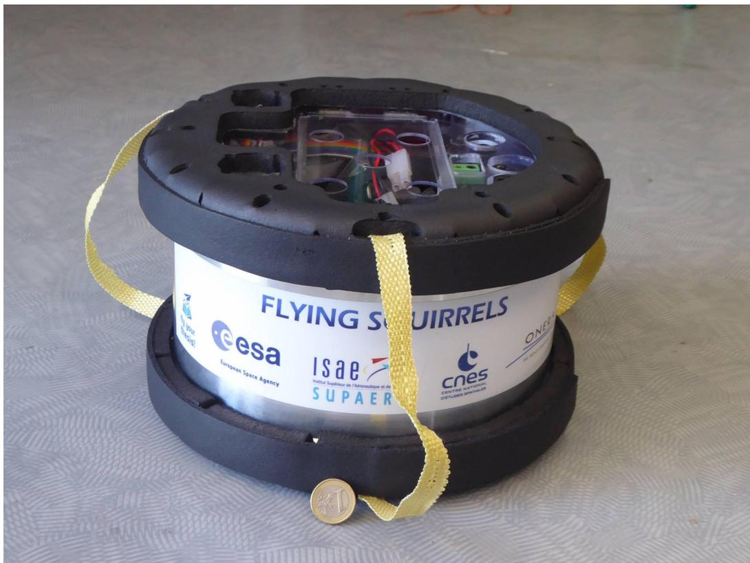
Figure 7.6: A picture of the SCRAT-0g platform tested on a parabolic flight (courtesy of ISAE SUPAERO and ONERA).
