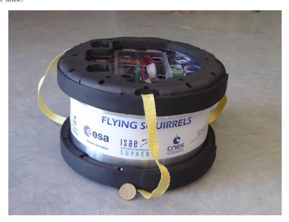
Figure 7.6: A picture of the SCRAT-0g platform tested on a parabolic flight (courtesy of ISAE SUPAERO and ONERA).
