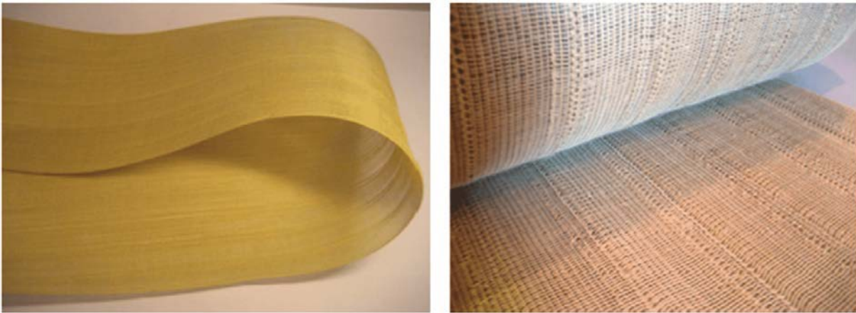
FIGURE 1.4 – Hybrid PPS/SMA/Kevlar fabric (Meo et al. [46])
