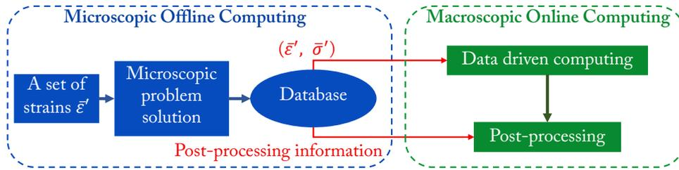
FIGURE 4.2 – The flowchart of the proposed data-driven FE<sup>2</sup> method.
