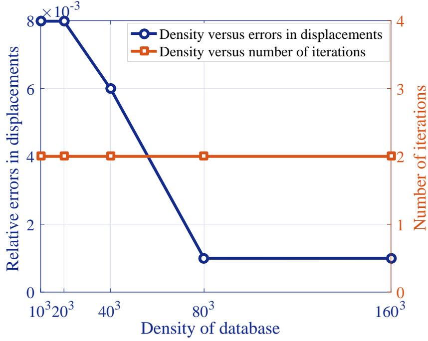
FIGURE 4.5 – The evolution of relative errors in displacements and iteration numbers along with the increasing of data density.
