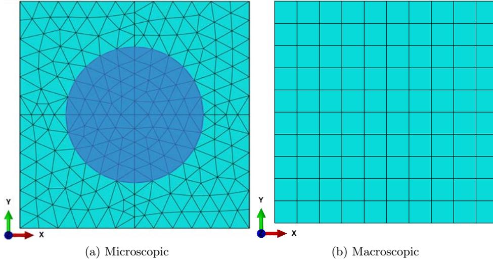
FIGURE 4.4 – Mesh of the RVE and the 1/4 composite plate.
