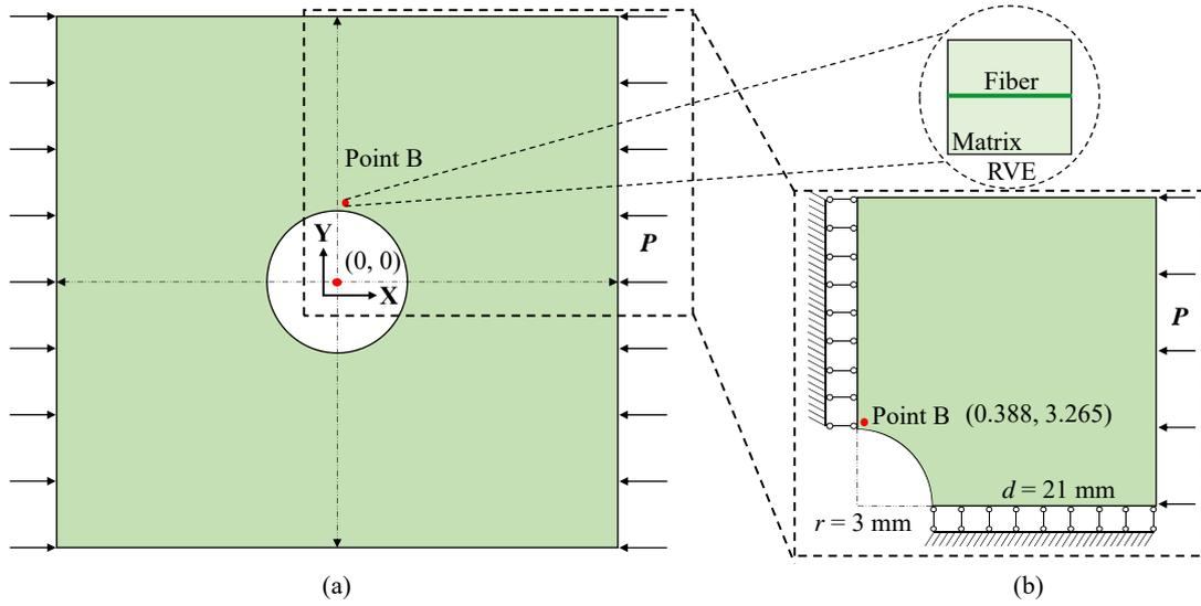
FIGURE 4.8 – Configuration of the composite plate with an hole in the center.
