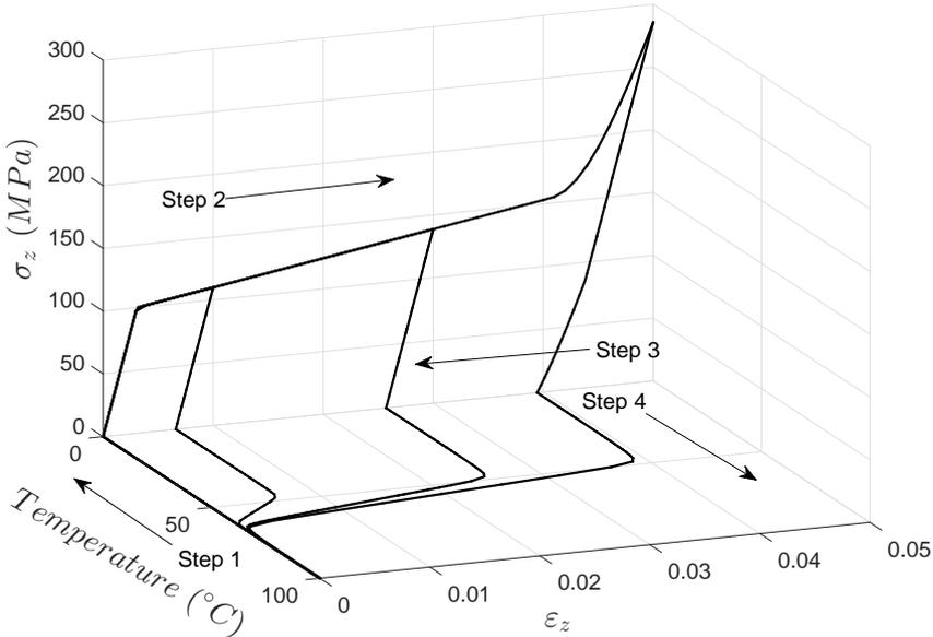
FIGURE 2.12 – The SME of pure SMA cube subjected to several strain levels.
