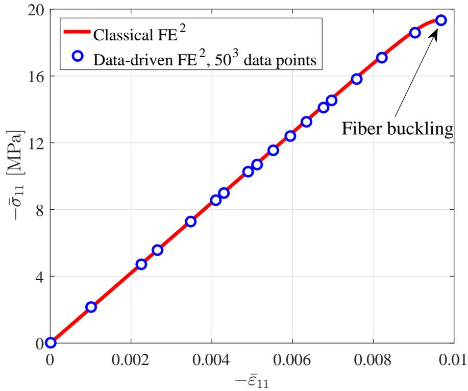
FIGURE 4.11 – Evolution of stress-strain relation at point B until the fiber buckles.
