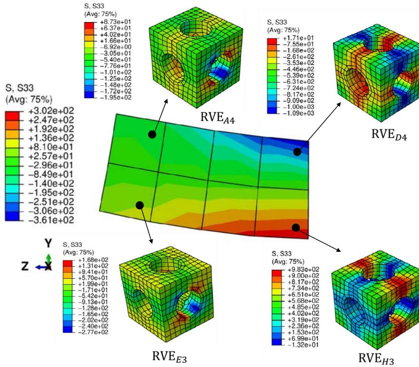
FIGURE 2.34 – The distribution of stress in Z direction (S33) for the macroscopic structure and microscopic structure with  $\xi = 40.7\%$ , where the deformations of both levels are magnified by three times.
