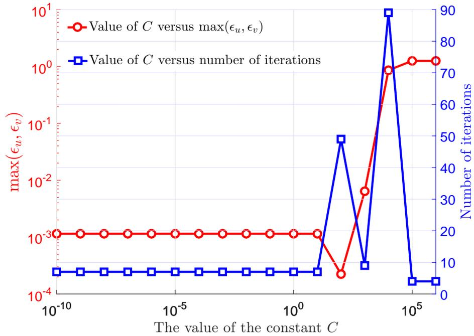
FIGURE 4.18 – Influence of the constant  $C$  in the penalty function  $\mathcal{F}$  on the accuracy of solution and the number of iterations required for the convergence, where the  $\max(\epsilon_u, \epsilon_v)$  represents the maximum relative error of displacements  $u$  and  $w$ .
