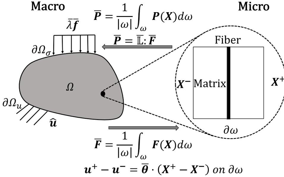
FIGURE 3.1 – Basic concept of multilevel finite element method.
