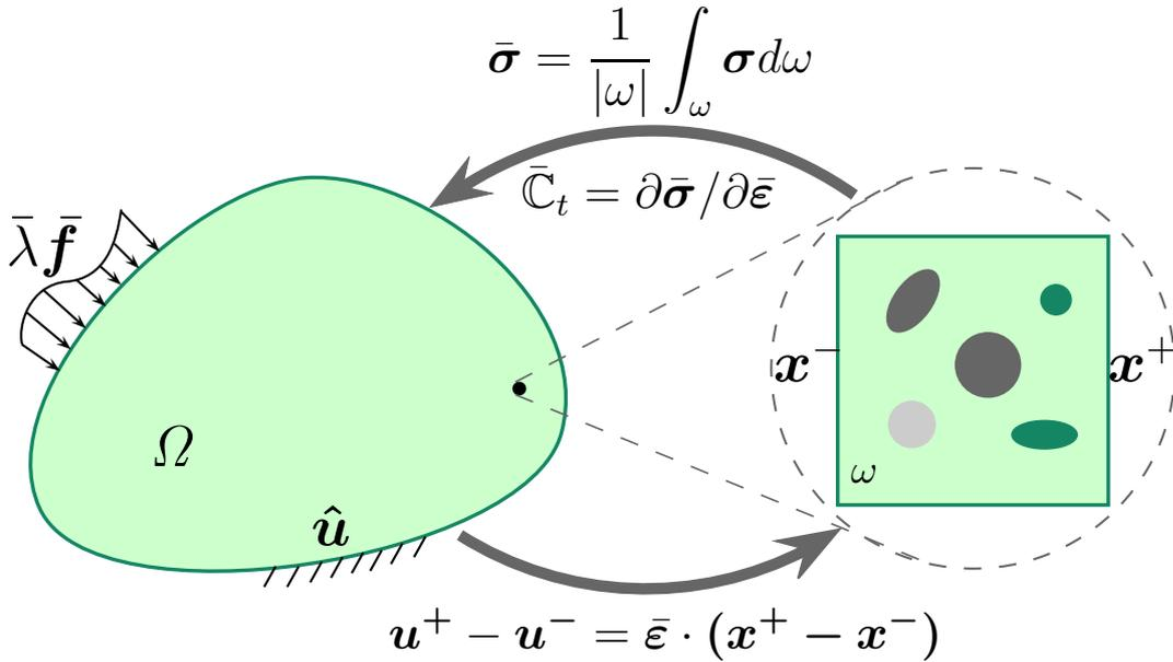
FIGURE 4.1 – Basic principle of the classical FE<sup>2</sup> method.
