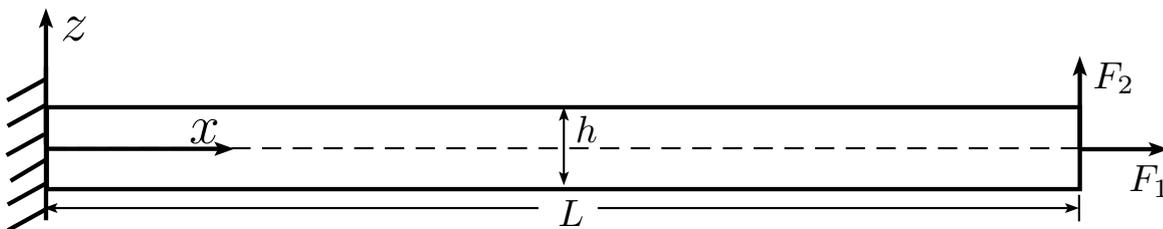
FIGURE 4.15 – A linear elastic homogeneous cantilever beam subjected to a point load at its free end.
