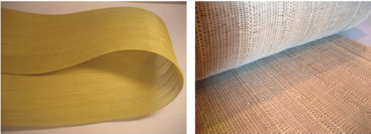
FIGURE 1.4 – Hybrid PPS/SMA/Kevlar fabric (Meo et al. [46])
