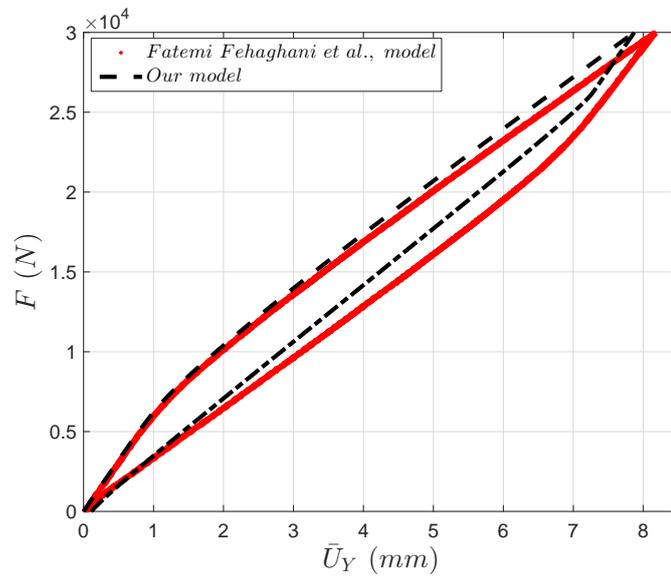
FIGURE 2.10 – Comparison of force versus averaged transverse displacement diagrams over face  $Z=100$  mm, simulated by the adopted FE<sup>2</sup> model and the reference Dehaghani et al. [58] model respectively.
