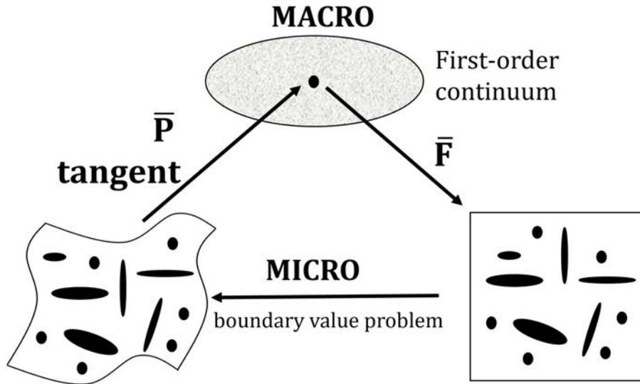
FIGURE 1.7 – Schematic diagram of the first-order  $FE^2$  model.
