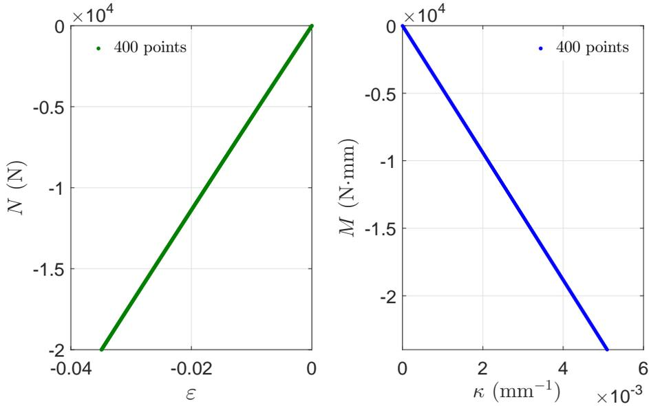
FIGURE 4.23 – Structural-genome database for the thin composite beam.
