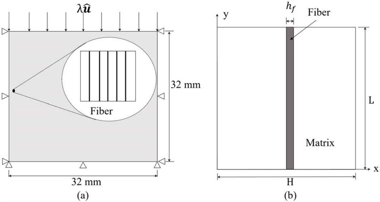
FIGURE 3.3 – (a) the fiber reinforced composite plate subjected to compressive displacement load; (b) Elementary cell of fiber reinforced material,  $H = L = 1$  mm,  $h_f/L = 1/20$ .
