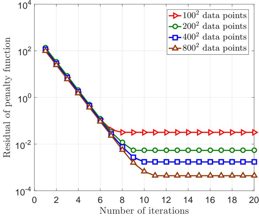
FIGURE 4.17 – Convergence of the penalty function  $\mathcal{F}$  with the number of iterations and with the number of structural-genome data points.
