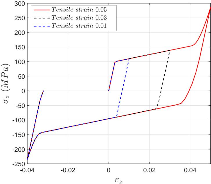
FIGURE 2.13 – Orientation of SMA subjected to several tensile-compression loadings at 0 °C.
