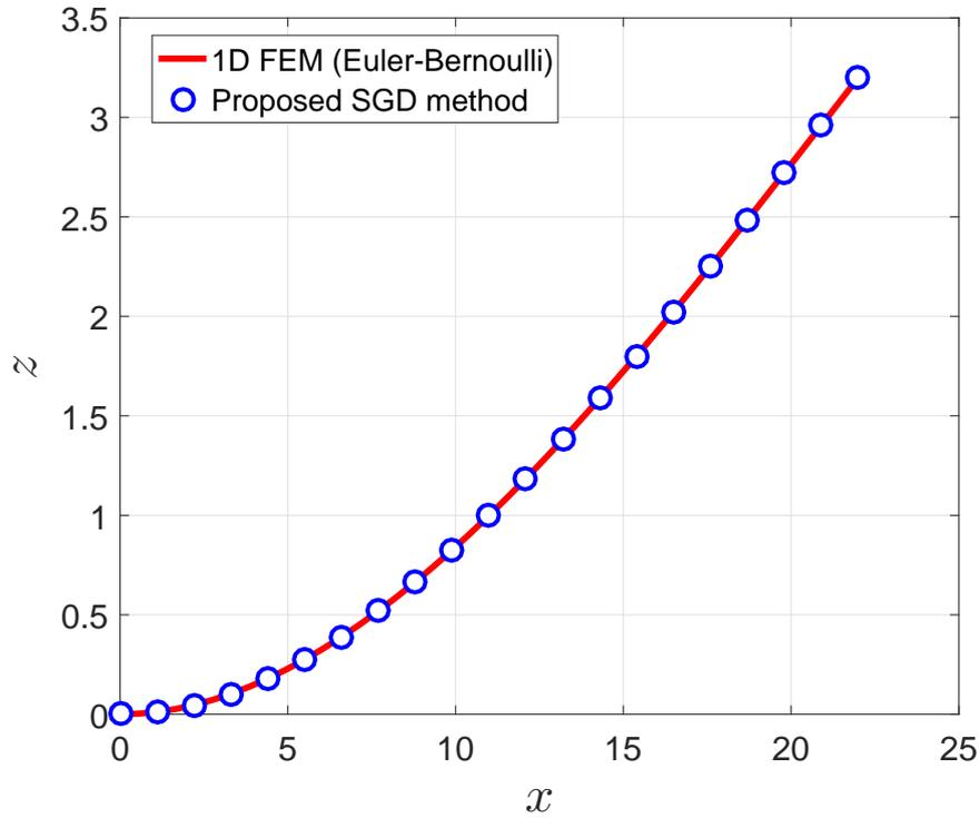
FIGURE 4.16 – Deformed shapes of the cantilever beam under tension and bending simulated by two methods.
