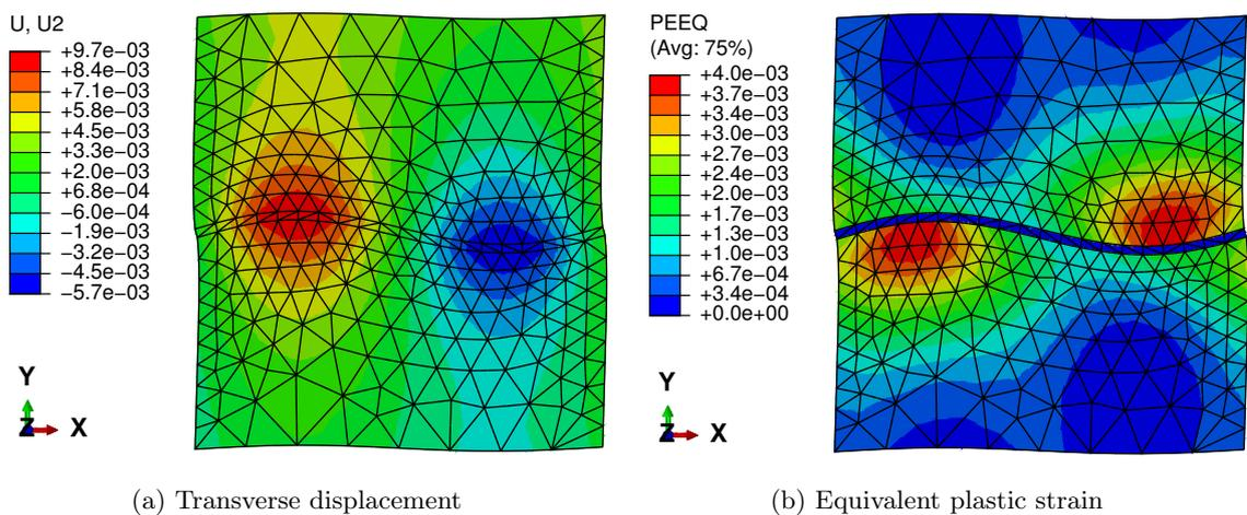
FIGURE 4.12 – Deformation and strain distribution over the RVE related to point B at state fiber buckling.
