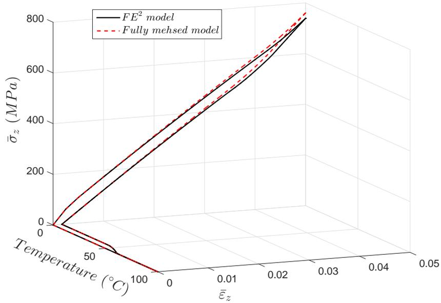
FIGURE 2.16 – Averaged stress, strain and temperature diagrams of face  $Z=10$  mm of composite modeled by the  $FE^2$  model and fully meshed model respectively.
