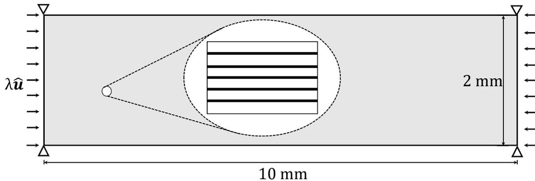
FIGURE 3.10 – The fiber reinforced beam subjected to compressive displacement load.
