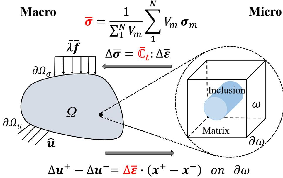
FIGURE 2.1 – Basic concept of finite element square method.
