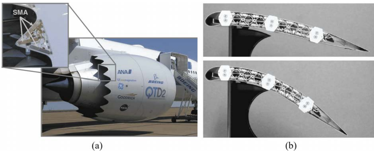
FIGURE 1.2 – (a) Boeing variable geometry chevron, flight testing (Hartl and Lagoudas [4]); (b) An artificial wing made by SMA (Sofla et al. [5]).
