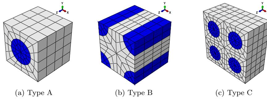
FIGURE 2.6 – Three types of fine meshed RVE.
