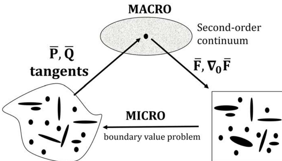
FIGURE 1.8 – Schematic diagram of the second-order  $FE^2$  model.
