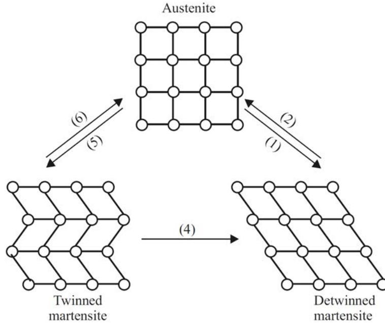
FIGURE 1.3 – Changes in the crystal structure : (1) loading/cooling; (2) unloading/heating; (4) loading; (5) cooling; (6) heating. (Sun and Huang [6]).
