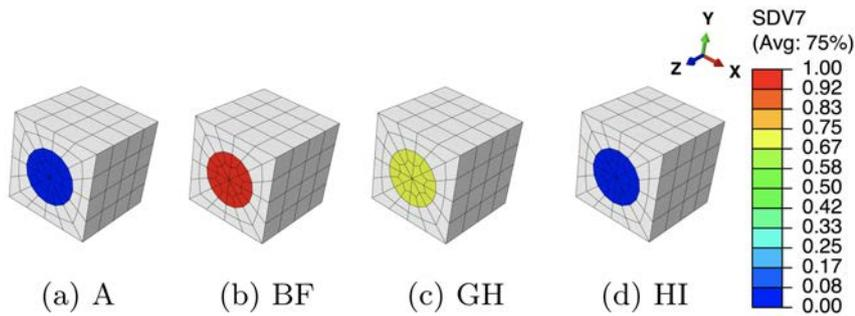
FIGURE 2.15 – Distribution of martensitic volume fraction in fiber.
