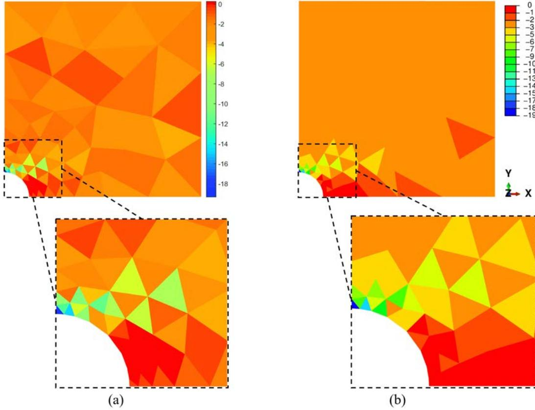
FIGURE 4.10 – The distribution of stress component  $\bar{\sigma}_{11}$  (MPa) over the local hole and the global plate when the fiber buckling at point B is triggered : (a) data-driven FE<sup>2</sup> method ; (b) classical FE<sup>2</sup> method.
