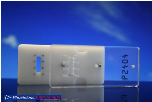
Figure 22: The intestine has to be mounted on pins of the serosal half of the Ussing chamber insert.
