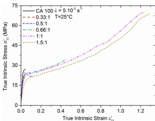
Fig. 11. True intrinsic mechanical behaviours of the different materials as function of the NH<sub>2</sub>:MAH molar ratio.
