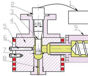
1.Ultrasonic generator 2.Piezoelectric transducer
