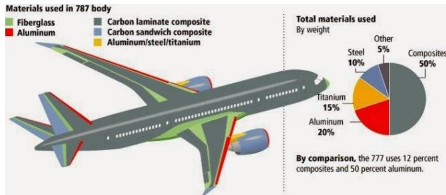
Figure 1 : Composition du Boeing 787 (source: tpeaviation.wordpress.com)
