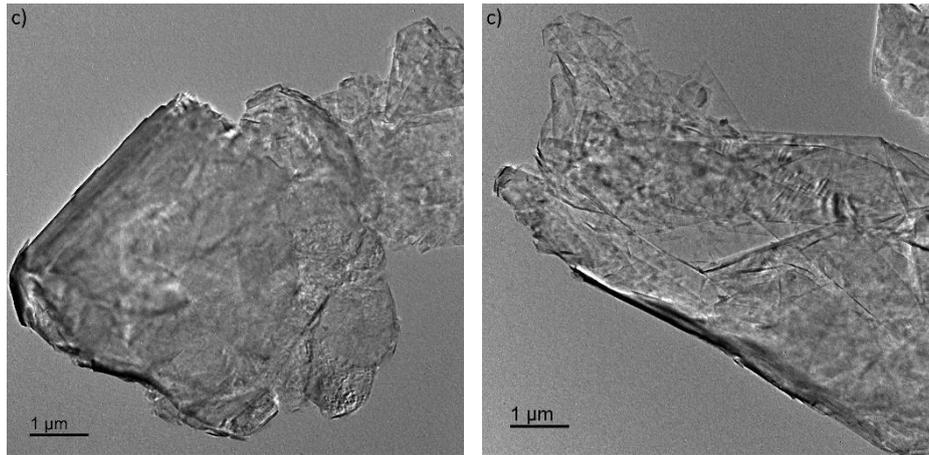
Figure III.13: Micrographies MET de la nano-charge KNG 180.
