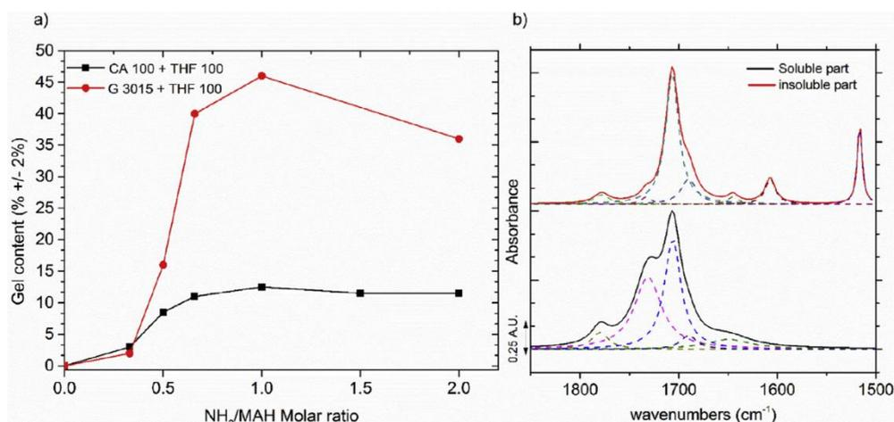
Fig. 2. a) Gel Content evolution of CA 100 and G 3015 based materials after reaction with Jeffamine THF 100 at various molar ratio NH<sub>2</sub>:MAH and b) FTIR spectra of the CA 100 1:1 soluble and insoluble parts.
