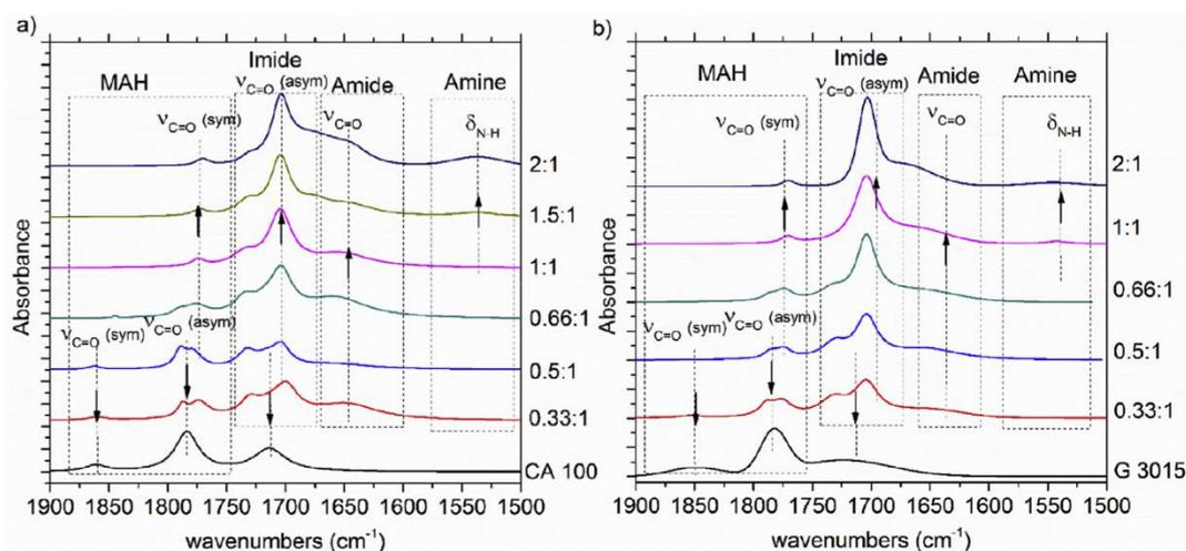
Fig. 3. FTIR spectra of a) the CA 100 based materials and b) the G 3015 based materials as a function of the NH<sub>2</sub>:MAH ratio.
