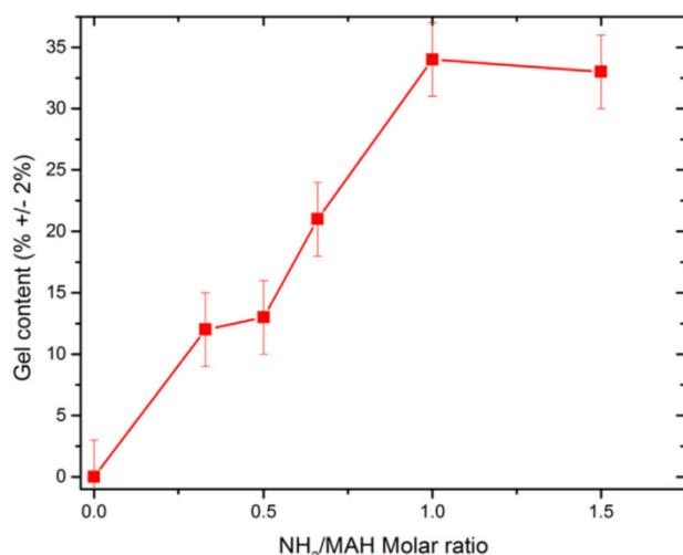
Fig. 3. Gel content measurements evolution as a function of the NH<sub>2</sub>:MAH molar ratio.
