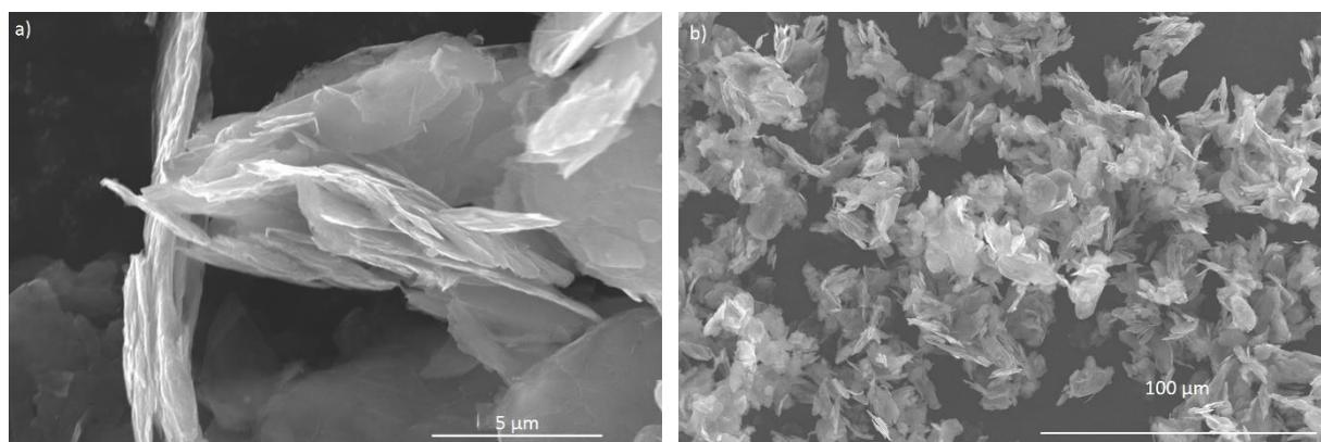
Figure III.12: Micrographies MEB des nano-charges KNG 180.
