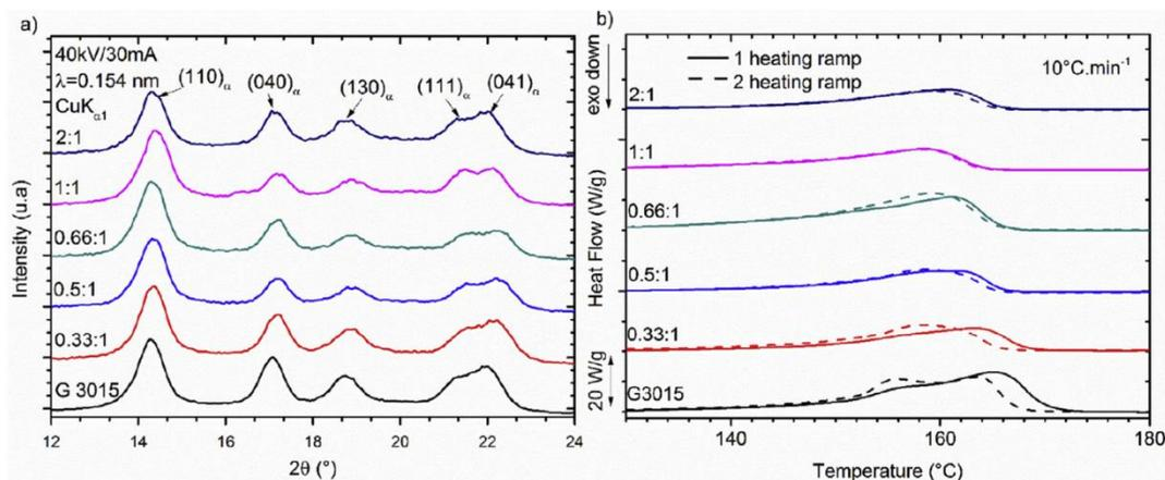
Fig. 5. a) 1D WAXS diffractograms and b) DSC thermograms of G 3015 and the modified materials prepared at variable  $\text{NH}_2$ :MAH molar ratios.
