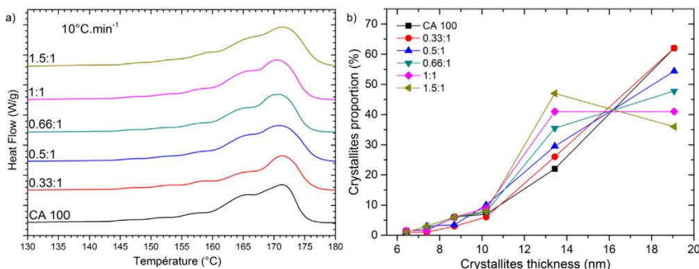
Fig. 6. a) SSA last thermograms for the different materials as a function of the NH<sub>2</sub>:MAH molar ratio, and b) distribution of the different lamellae populations between the different thickness according to their melting temperature.
