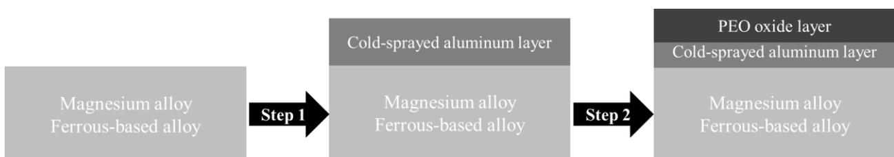
**Fig. VI-11:** Schematic view of a duplex treatment involving cold spray and PEO techniques.
