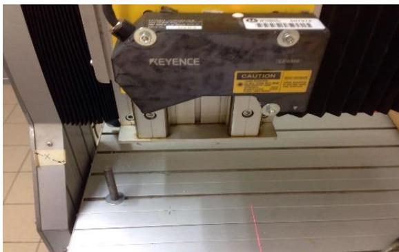
Figure 2.32: Scanner Laser [15]
