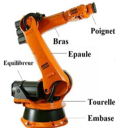
Figure 2.1(a): Robot Kuka Kr 210L180 [8]
