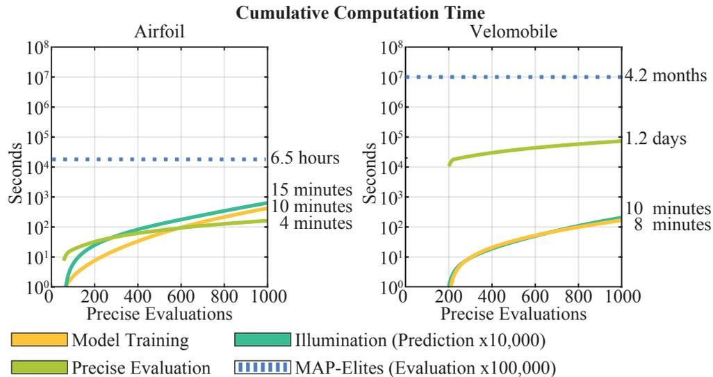
Figure 5.18: *Cumulative Computational Cost of SAIL Components.*
