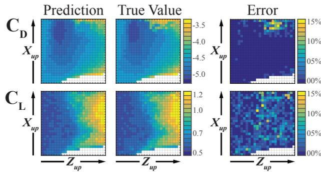
Figure 5.4: *Drag and Lift Predictions Per Bin*
