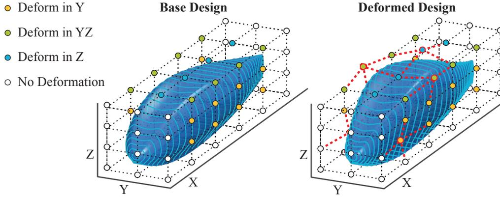
Figure 5.10: *Velomobile Design Created through Free-Form Deformation.*
