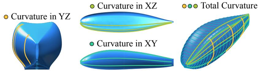
Figure 5.11: *Determination of Curvature from Selected Sections.*
