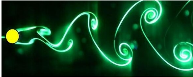
Figure 1.6: Swirling alley of Bénard-Von Karman, appearing in the wake of a cylinder transverse to the flow, beyond a minimum speed [23]
