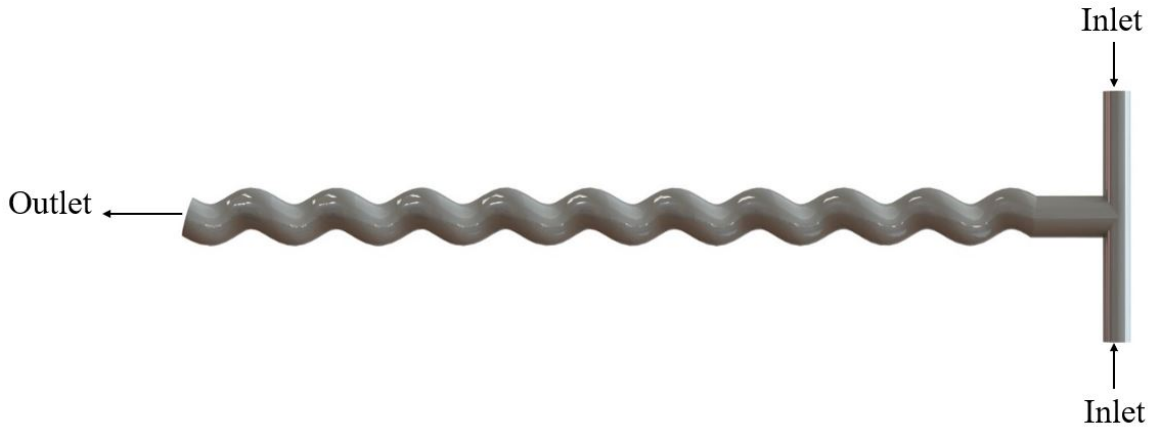
Figure 1: T-shaped micro-mixer with a HCHP design
