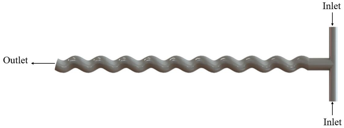
Figure 1: T-shaped micro-mixer with a HCHP design
