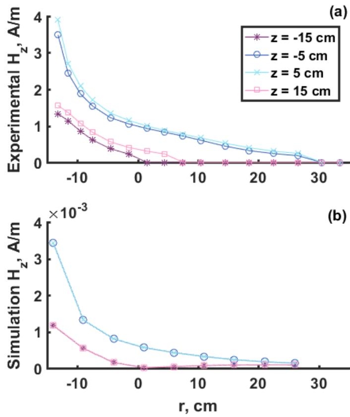
Fig. 4.31.  $H_z(r)$  in vacuum: (a) measured in experiment, (b) calculated in simulation.
