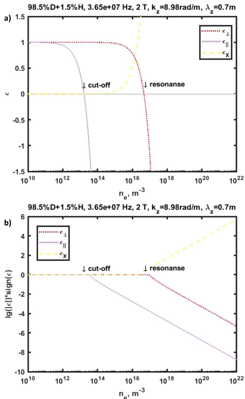
Fig. 2.3. Elements of dielectric tensor  $\epsilon_{\perp}$ ,  $\epsilon_{\parallel}$ ,  $\epsilon_X$  as a function of density: a) part of the range in linear scale to show the small values, b) same in logarithmic scale to show the big values.
