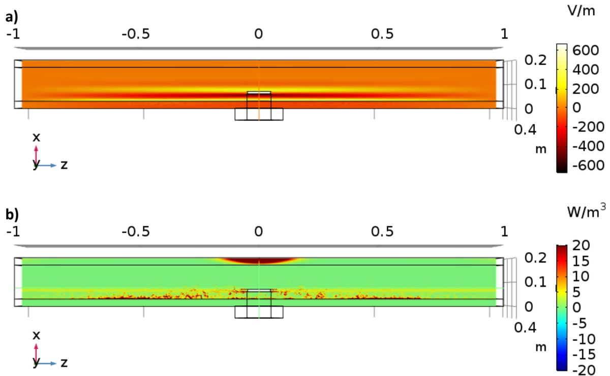
Fig. 4.43. Solution with the collisional losses and no side PMLs,  $n = 5 \cdot 10^{15} \text{ m}^{-3}$ : (a) electric field  $E_x$ , (b) total power dissipation density.
