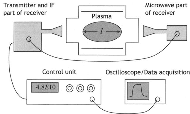
Fig. 2.8. Principle setup of MWI 2650
