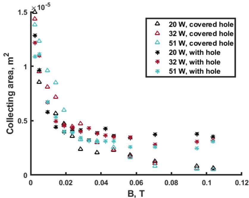
Fig. 3.5. Example of the collecting area for  $r_{pr} = 75 \mu\text{m}$  when a hole is present and when it is covered.
