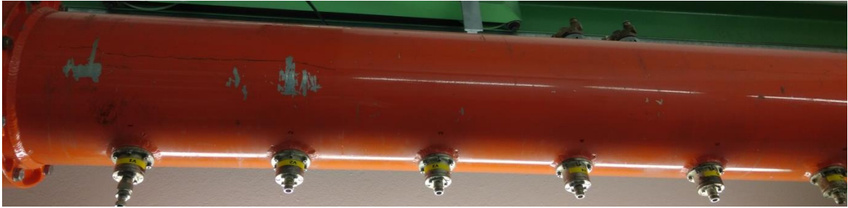
Fig. 4.55. Array of voltage probes in the unmatched IShTAR coaxial line.
