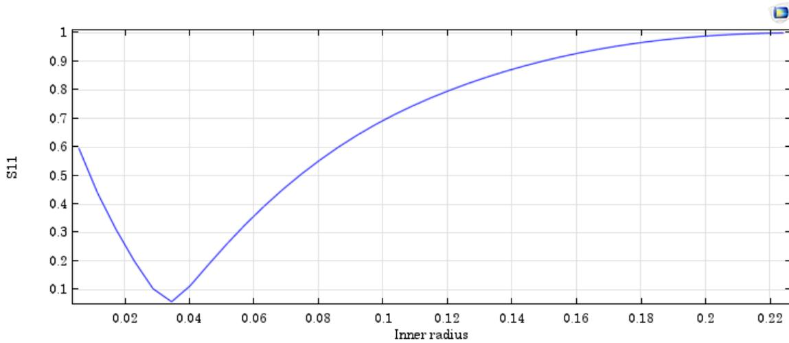
Fig. 4.54. Absolute value of  $S_{11}$  as a function of inner radius of the middle coaxial cable for  $Z_3 = 260.2 \Omega$ .
