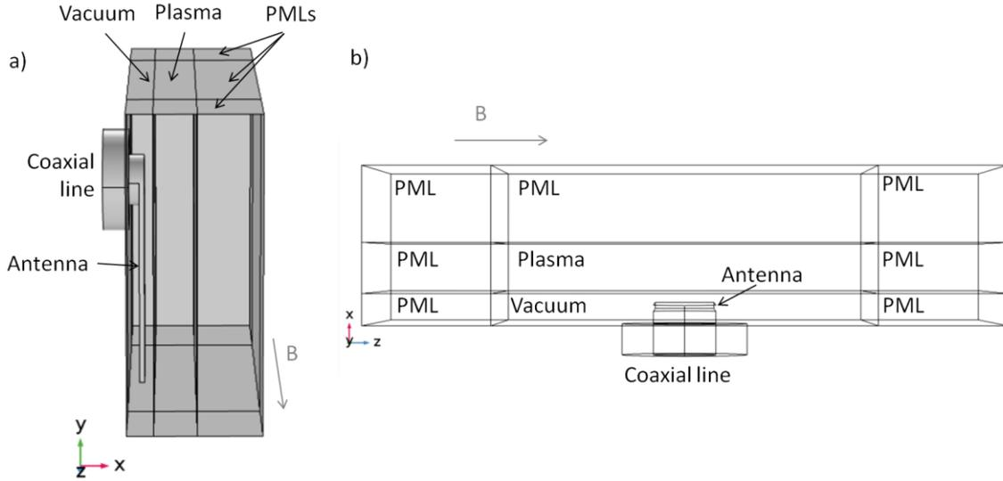
Fig. 4.35. COMSOL model geometry: (a) side view, (b) top view.
