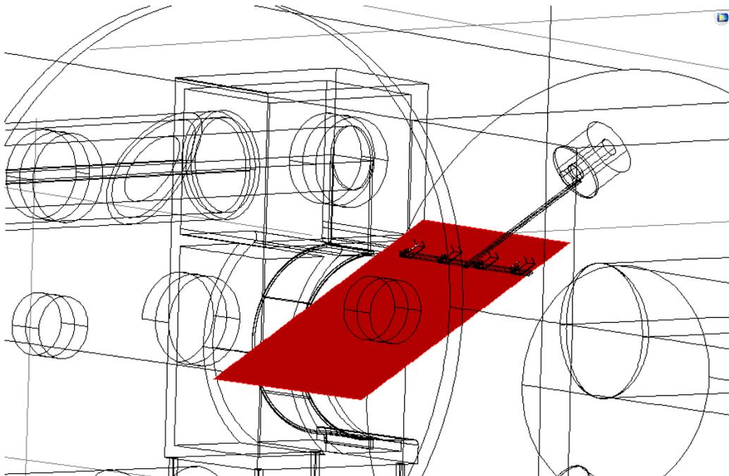
Fig. 4.32. The plane of the radial movement of the manipulator.
