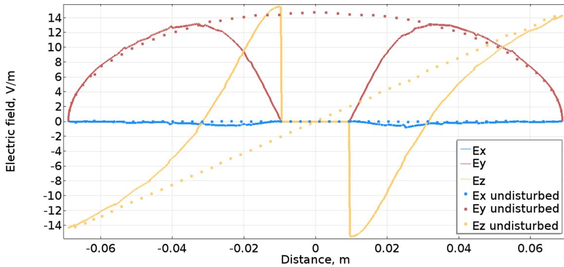
Fig. 4.23. Electric field disturbance along  $\varphi$ .
