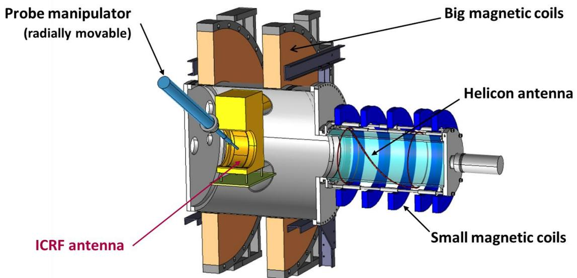
Fig. 1.7. IShTAR model with all main components.
