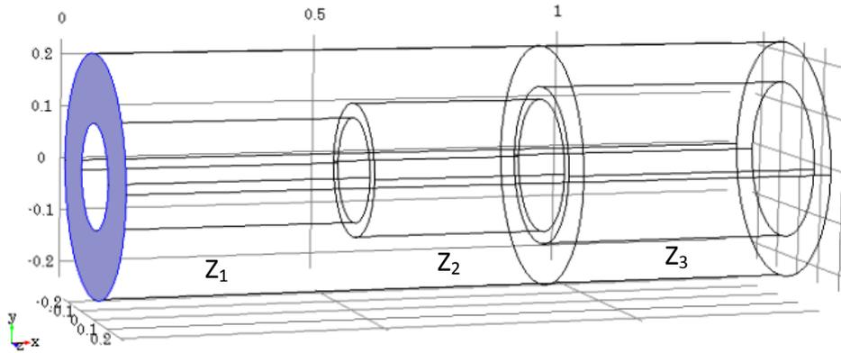
Fig. 4.51. Model with three adjacent coaxial cables.
