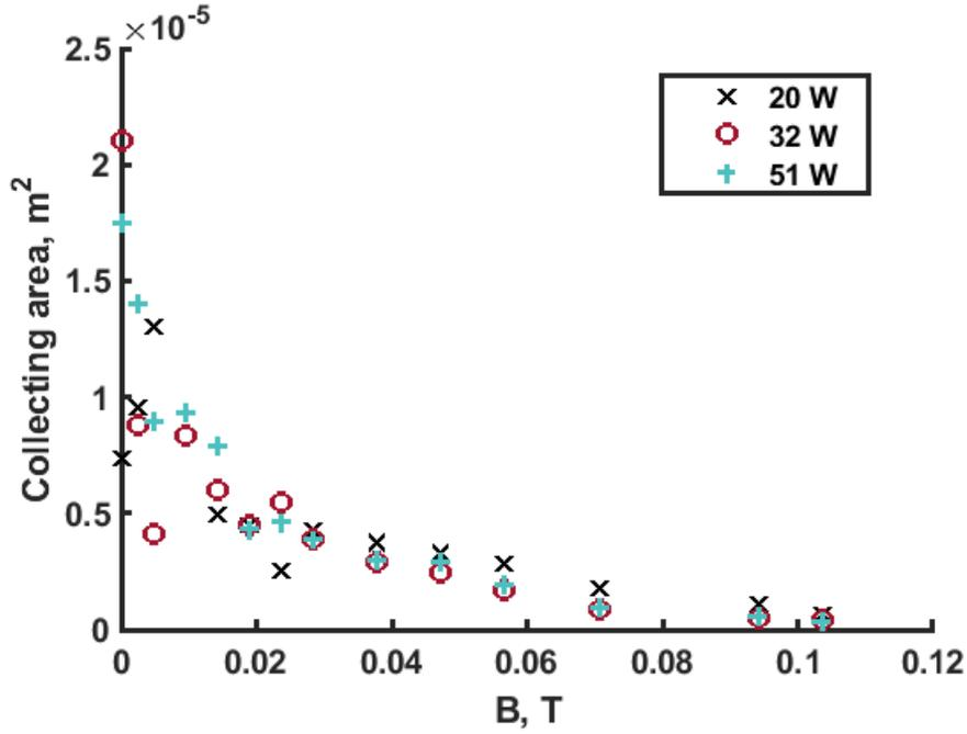
Fig. 3.1. Collecting area of the smaller cylindrical probe estimated using planar probe density measurements for 3 different forwarded RF power levels.
