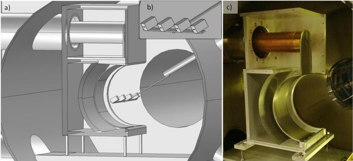
Fig. 4.28. (a) IShTAR model main components: ICRF antenna (side wall removed), manipulator and probes, (b) B-dot probe array on the manipulator (zoomed-in), (c) picture taken inside IShTAR.
