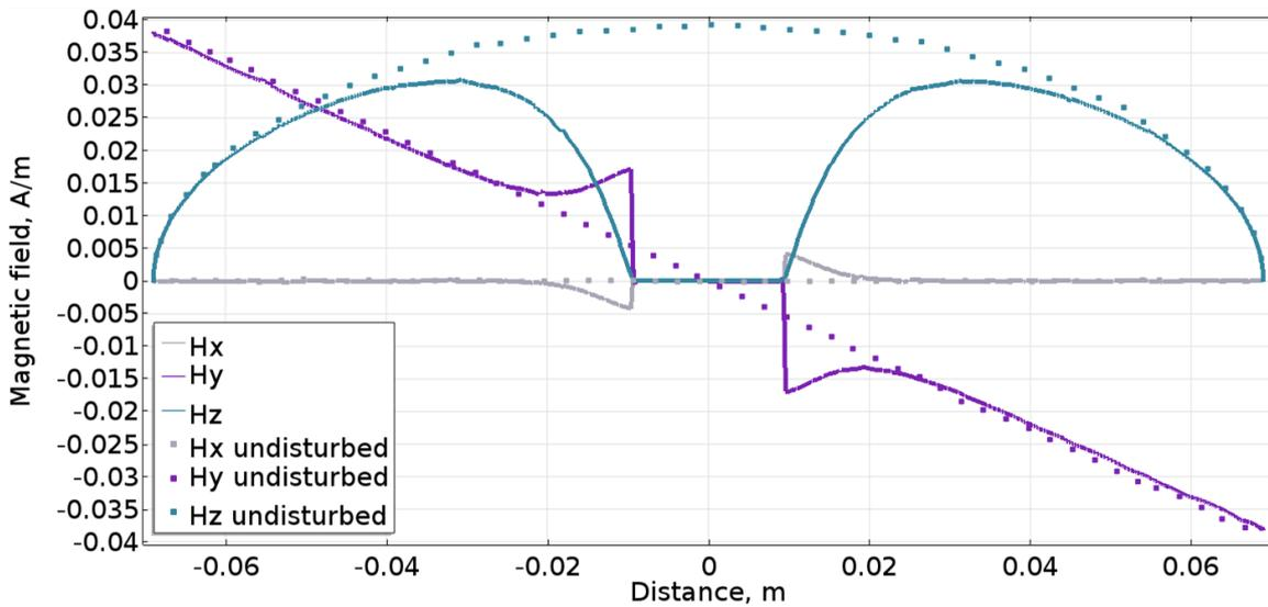
Fig. 4.24. Magnetic field disturbance along  $\varphi$ .
