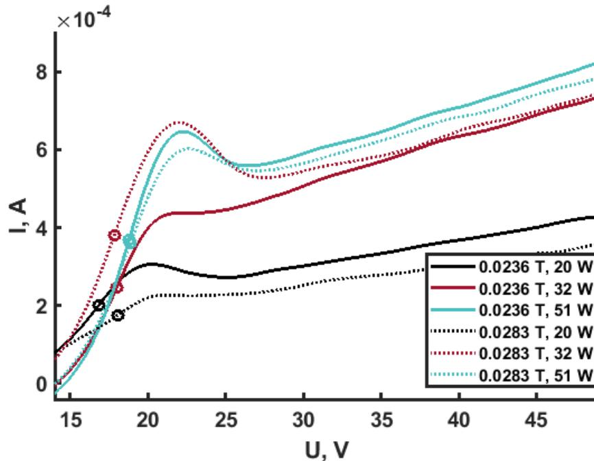
Fig. 3.20. Example of  $V_{pl}$  from the 1<sup>st</sup> derivative method (circle markers).
