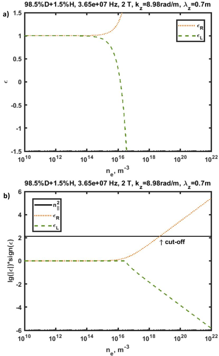
Fig. 2.4. Elements of dielectric tensor  $\epsilon_R$ ,  $\epsilon_L$  as a function of density: a) part of the range in linear scale to show the small values, b) same in logarithmic scale to show the big values.  $n_{\parallel}^2$  is also plotted to indicate the cut-off.
