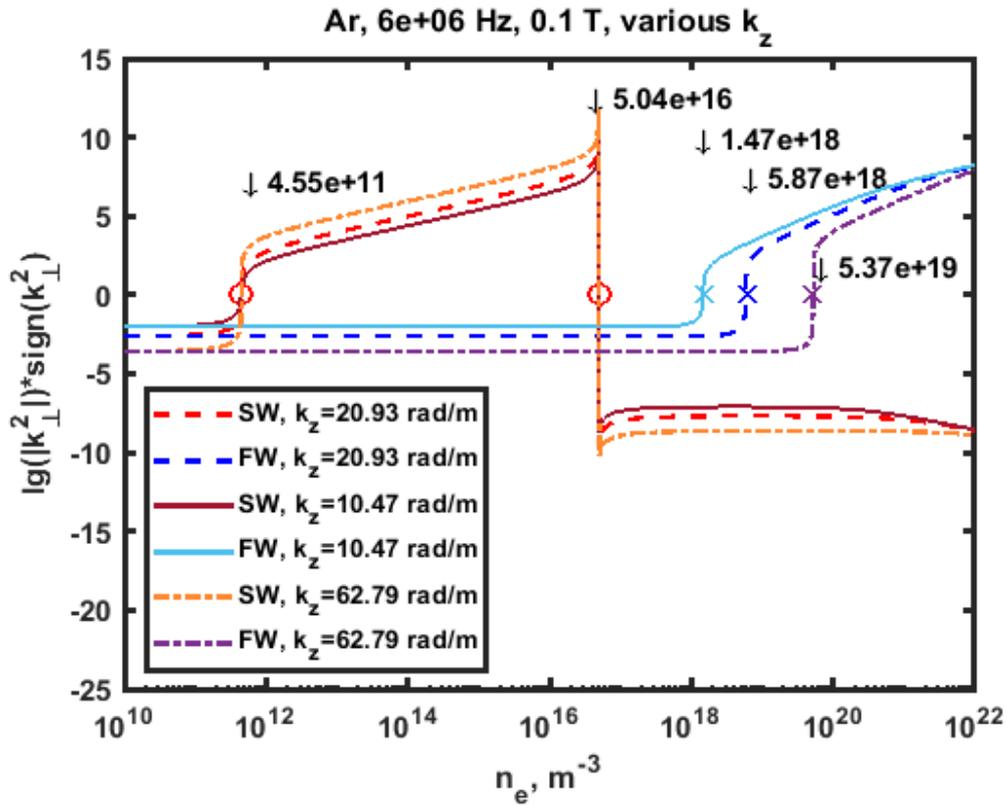
Fig. 4.5. SW and FW behaviour in IShTAR for various  $k_{\parallel}$ , in argon.
