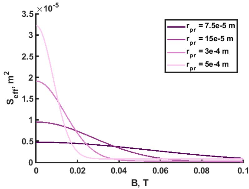
Fig. 3.2. Example of the effective collecting area for different probe radii at  $\theta = 0$ .
