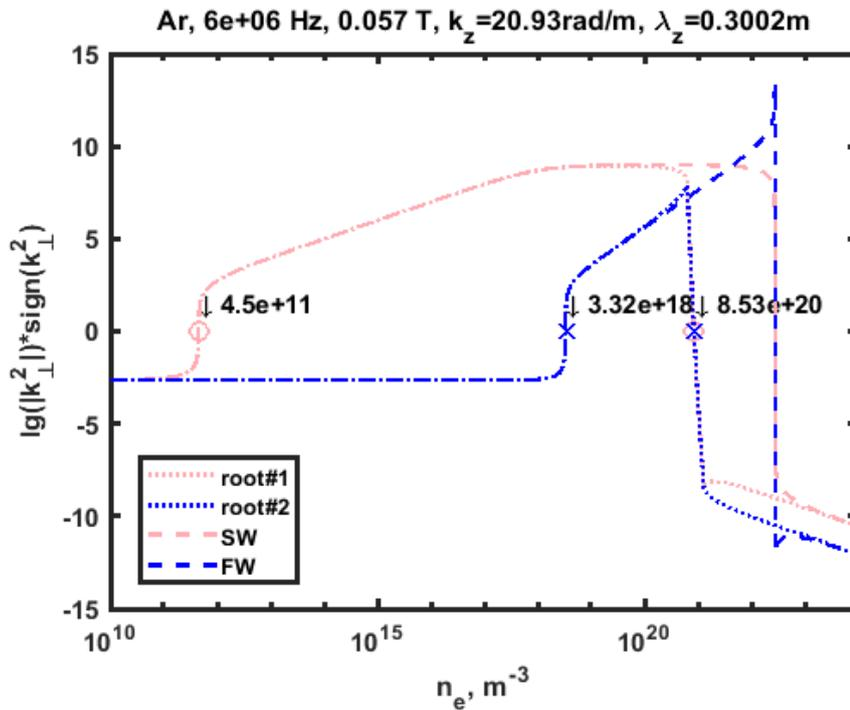
Fig. 4.7. SW and FW behaviour in IShTAR at the threshold  $B=0.057$  T, in argon.
