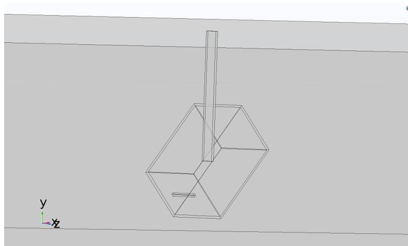
Fig. 4.15. B-dot probe geometry in COMSOL.
