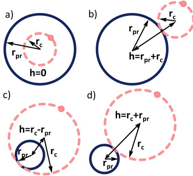
Fig. 3.12. Limiting cases for a particle to be collected, a)&b) for  $r_c < r_{pr}$ , c)&d) for  $r_c > r_{pr}$ . A dark circle represents the probe projection, a bright dashed circle – electron trajectory projection.
