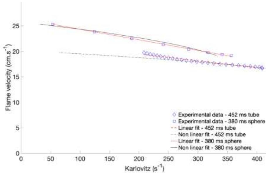
**Figure 6-9 Comparison of linear and nonlinear methods applied to a nanocellulose explosion:  $500 \text{ g.m}^{-3}$  concentration,  $t_v = 452 \text{ ms}$  – tube and  $t_v = 380 \text{ ms}$  – vented sphere**
