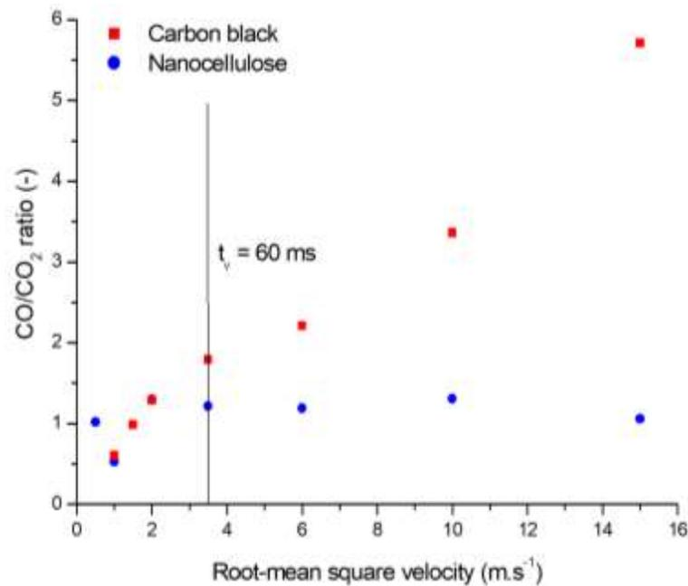
**Figure 5-31 Evolution of the CO/CO<sub>2</sub> ratio of the combustion gases of nanocellulose and carbon black with the root-mean square velocities**
