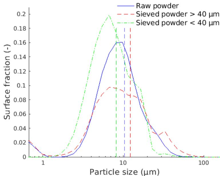
*Figure 5-2 Particle size distribution of raw and sieved nanocellulose after injection in the 20L at the moment of ignition (at 60 ms)*
