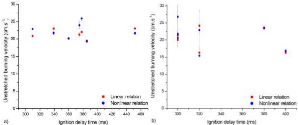
**Figure 6-8 Evolution of the laminar burning velocity of 500 g.m<sup>-3</sup> of nanocellulose with ignition delay time calculated by the linear and nonlinear relations in a) the propagation tube b) the vented 20L sphere**
