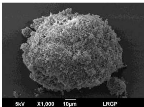
*Figure 3-1 SEM image of aluminum 100 nm*
