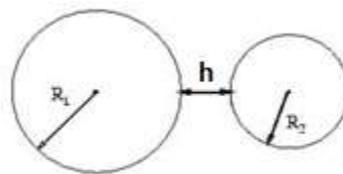
**Figure 2-5 Useful geometric considerations to present van der Waals forces between two spherical particles**
