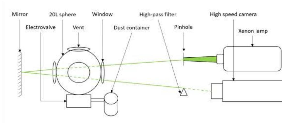
**Figure 6-2 Schematic of the Schlieren setup and the modified 20L sphere**
