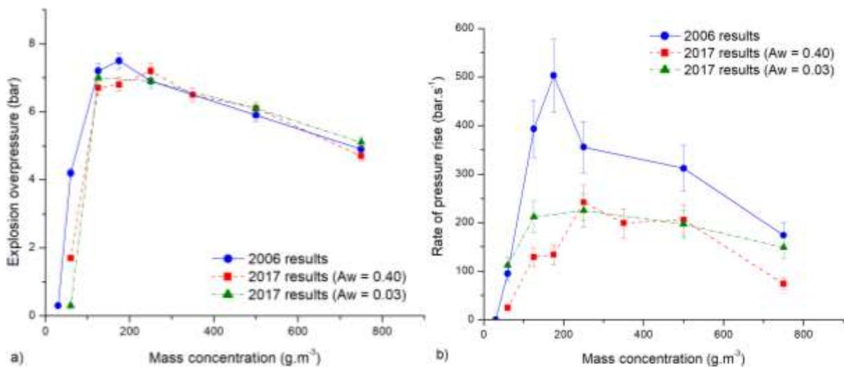
**Figure 5-14 Evolution of the explosion a) overpressure and b) rate of pressure rise with the concentration for carbon black powder in 2006 and 2017 (raw and dry)**
