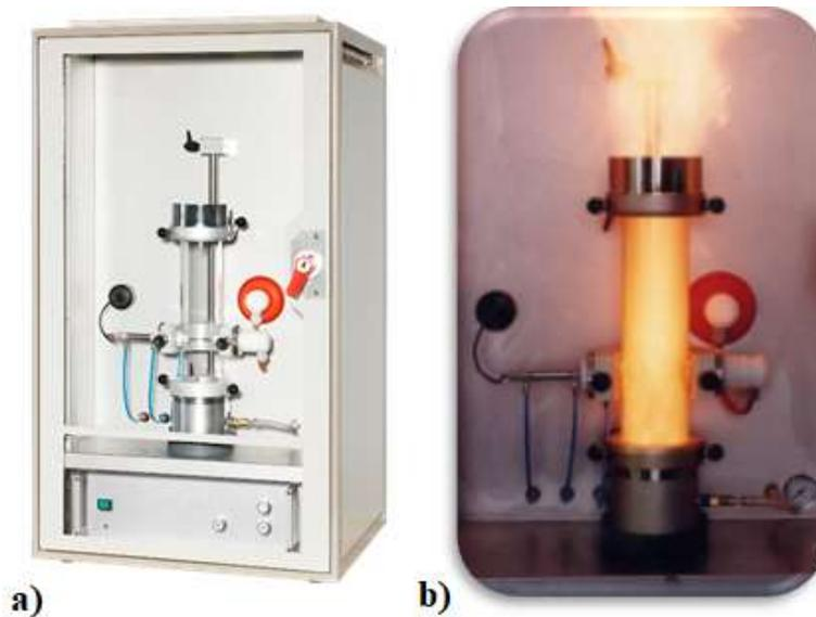
**Figure 4-1 a) Modified Hartmann tube (TÜV SÜD Schweiz AG, 2020) b) Modified Hartmann tube during an ignition**
