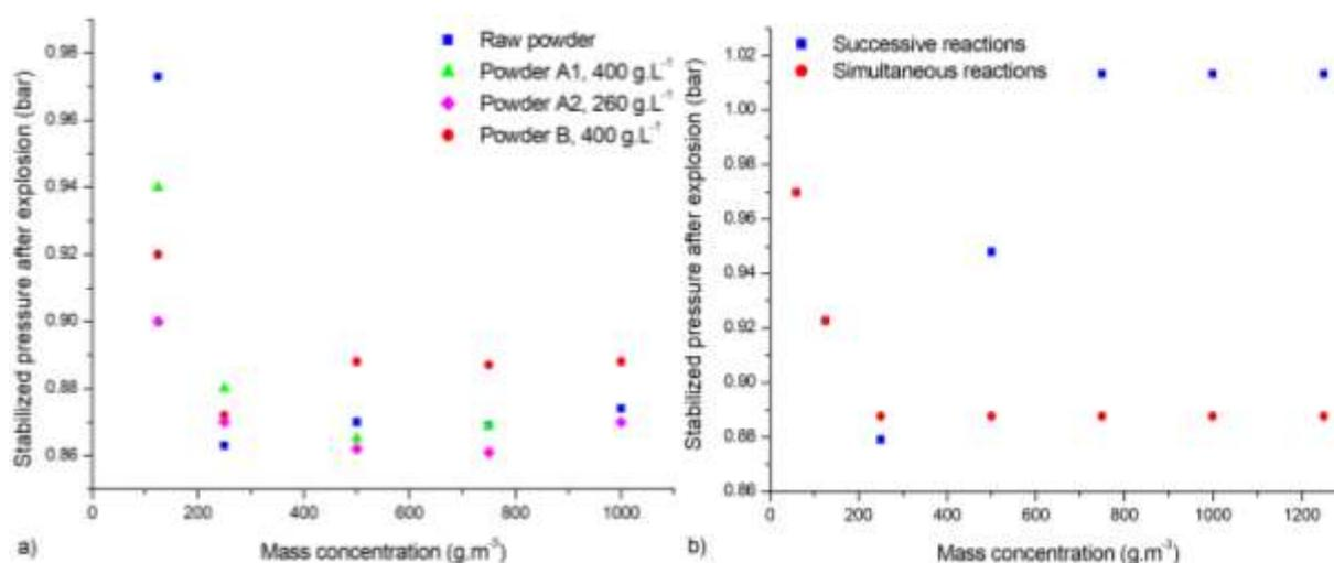
**Figure 5-12 Evolution of the stabilized pressure after explosion in the 20L sphere with the mass concentration a) experimentally measured for the different samples of carbon-coated silicon b) calculated for the raw powder**
