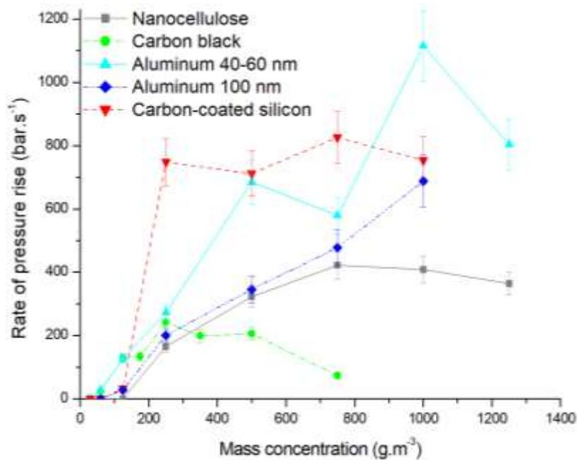
**Figure 4-8 Evolution of the rate of pressure rise with the concentration for the studied powders in standard conditions**
