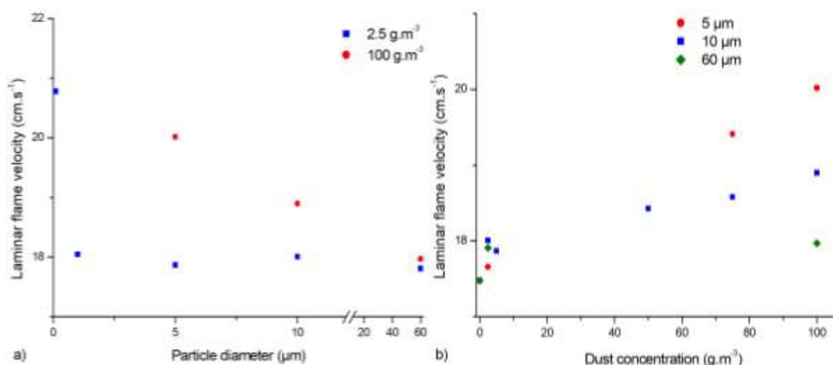
**Figure 6-19 Influence of the a) primary diameter and b) dust concentration considered for the radiative heat transfer during the combustion of the pyrolysis gases of 500 g.m<sup>-3</sup> of nanocellulose**
