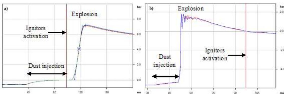
**Figure 5-19** Pressure-time evolution of an aluminum explosion at 750 g.m<sup>-3</sup> with a) air injection b) nitrogen injection.
