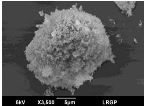
**Figure 3-4 SEM image of silicon coated by carbon**
