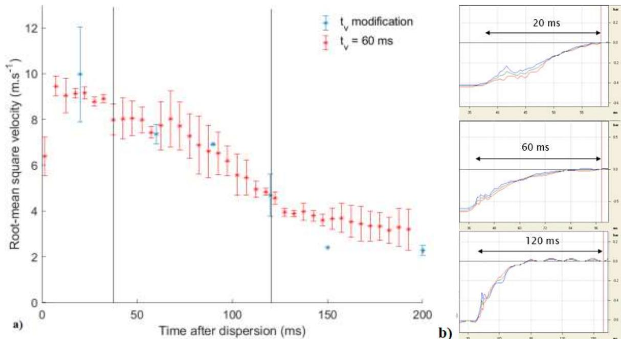
**Figure 5-28 a) Time evolution of the root-mean-square velocity within the 20L sphere during a standard injection for various ignition delay times b) Modifications of the injection dynamic for various ignition delay times**
