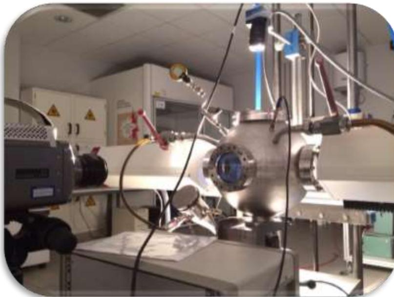
***Figure 3-9 Experimental set-up for the particle size distribution measurement in the visualization 20L sphere using the laser diffraction sensor (D'Amico, 2016)***
