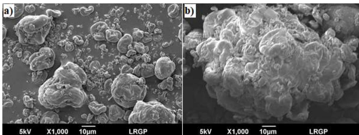
**Figure 5-4 Nanocellulose observed by Scanning Electron Microscopy a) Raw powder b) Agglomerated powder**
