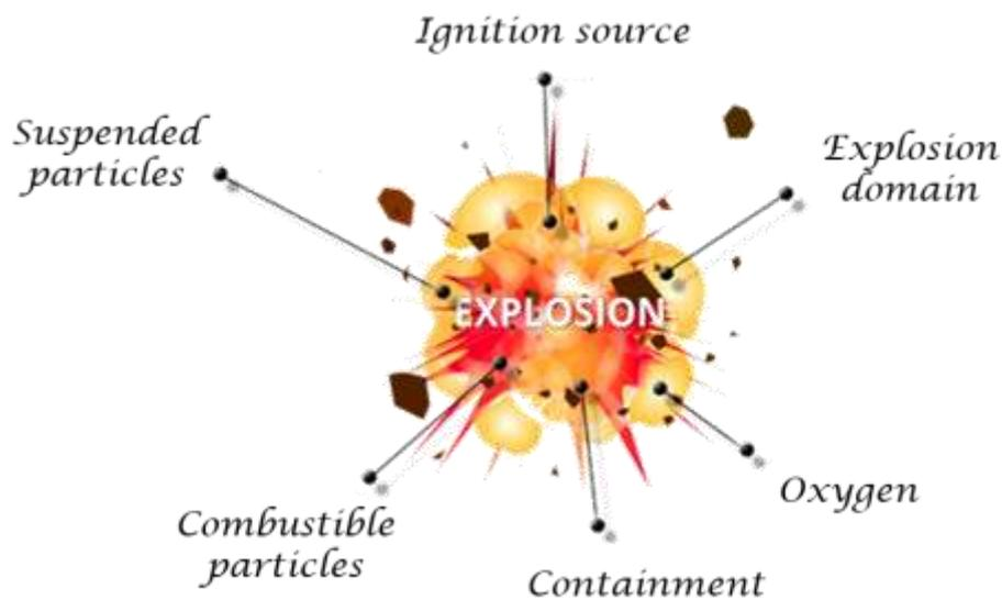
*Figure 2-1 Requirements to generate a dust explosion*
