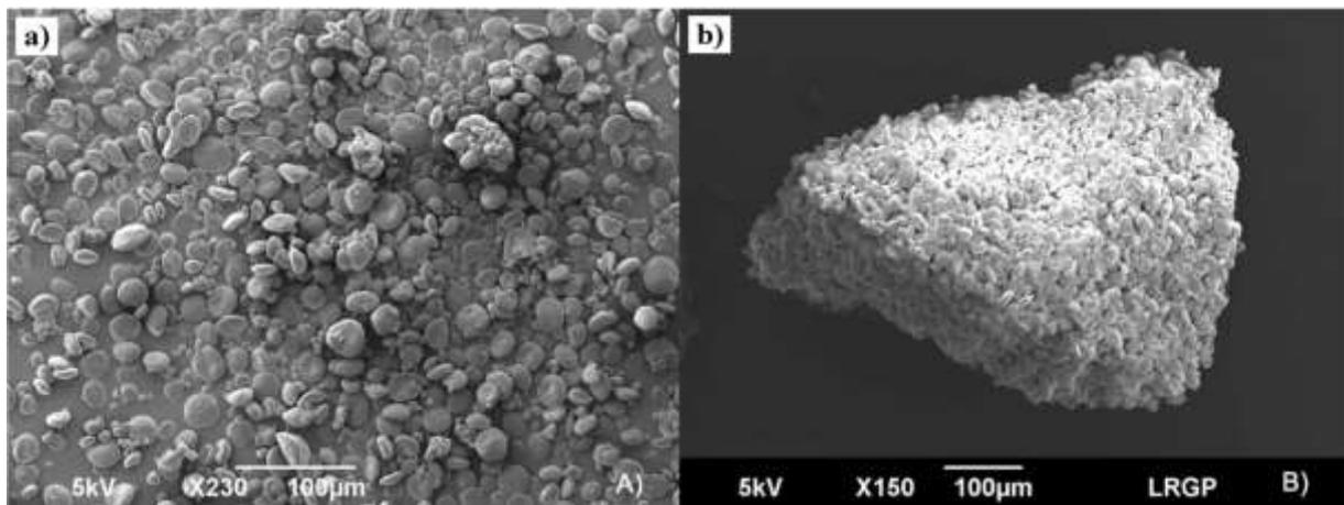
**Figure 5-6 SEM images of a) raw starch powder and b) a starch agglomerate generated by dry granulation**
