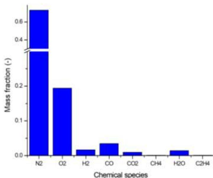
**Figure 6-15 Initial composition of the nanocellulose pyrolysis gases/air mixture considered in the flame propagation model**
