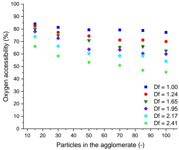
*Figure A-7 Evolution of the oxygen accessibility with the number of particles in agglomerates of different fractal dimensions*
