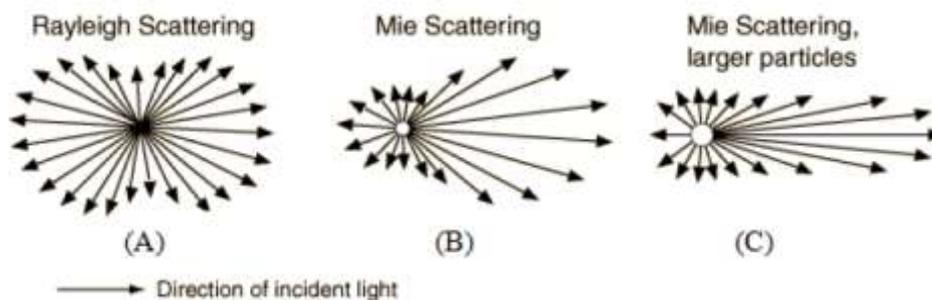
**Figure 2-12** Spatial distribution of light scattering for particles of different sizes (Ben Moussa, 2017)
