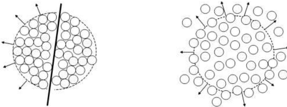
**Figure 2-9 Theoretical models of agglomerate fracture according to Rumpf (left) and Weiler (right) (Weiler et al., 2010)**
