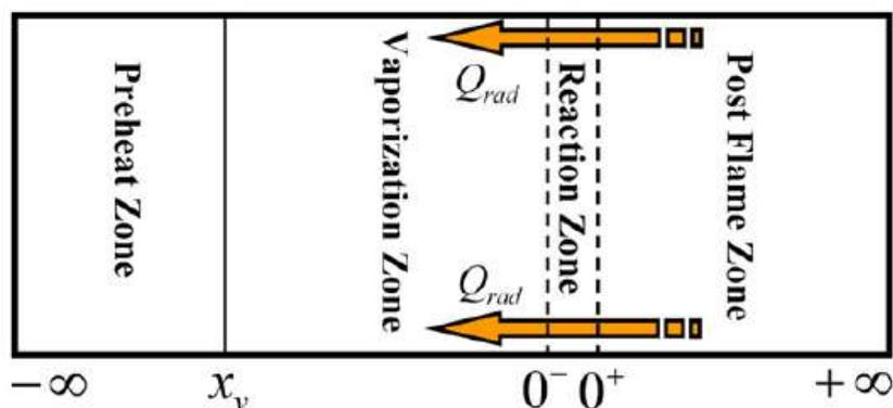
Figure 2-2 Schematic of the front flame propagation divided into four zones for organic particles in air (Haghiri and Bidabadi, 2010)
