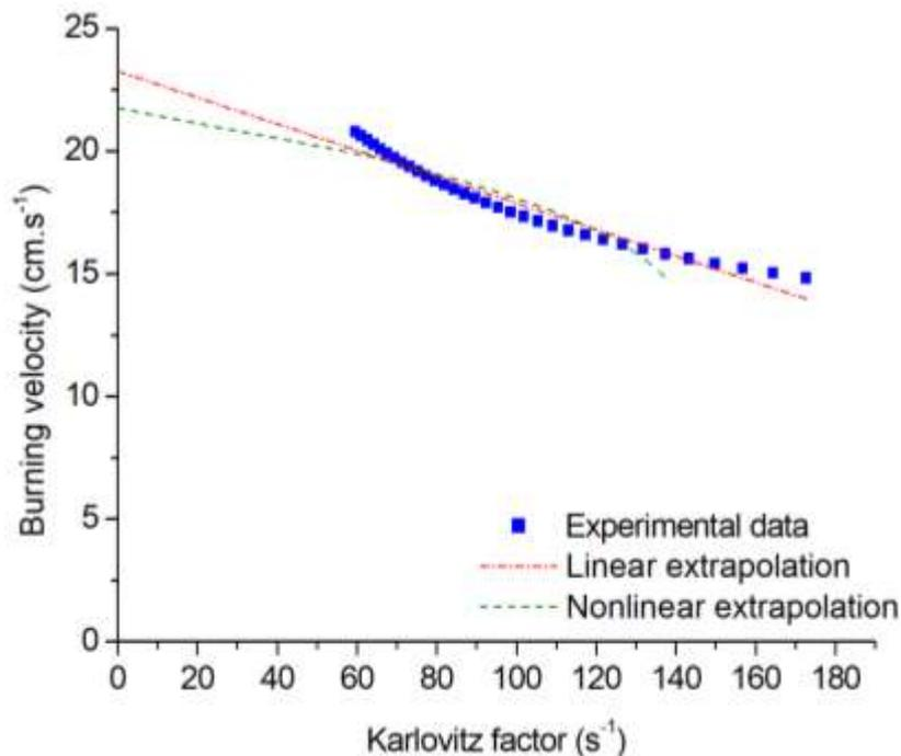
**Figure 6-6 Illustration of the burning velocity – stretching factor relation after smoothing for a  $500 \text{ g.m}^{-3}$  nanocellulose-air mixture for  $t_v = 340 \text{ ms}$**
