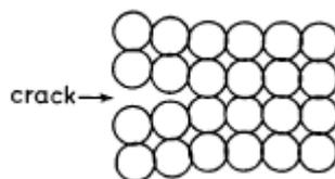
***Figure 2-8 Agglomerate fracture model according to Kendall (1988)***
