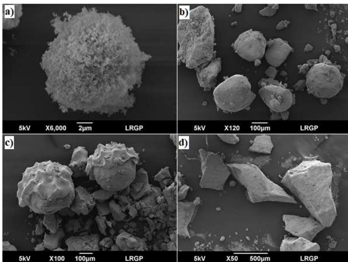
**Figure 5-8 Carbon-coated silicon observed by Scanning Electron Microscopy a) Raw powder b) Sample A1 ( $260 \text{ g.L}^{-1}$ ) c) Sample A2 ( $400 \text{ g.L}^{-1}$ ) d) Sample B ( $400 \text{ g.L}^{-1}$ )**
