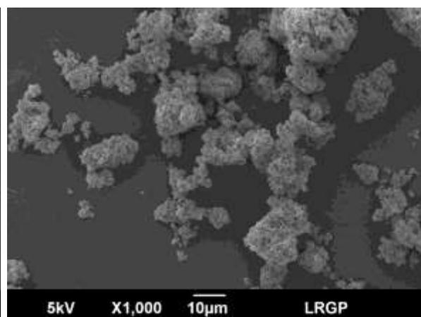
*Figure 3-2 SEM image of aluminum 40-60 nm*
