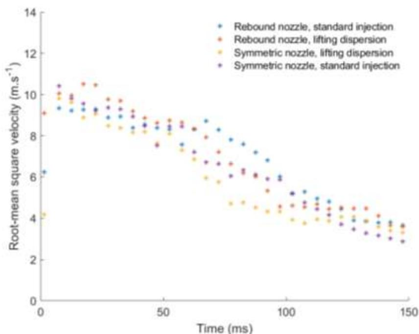
*Figure 5-26 Evolution of the root-mean square velocity with time after dispersion for different dispersion procedures*
