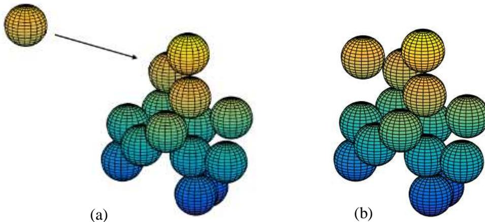
**Figure A-1 a) Particle propagating toward an agglomerate and b) particle added to the agglomerate**
