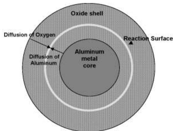
**Figure 2-10 Scheme of an aluminum particle with the oxide layer, surface reaction and oxygen diffusion (Rai et al., 2006)**
