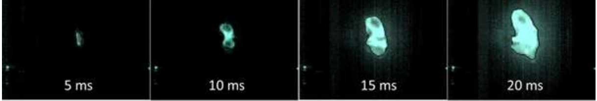
Figure 6-3 Time evolution of the flame profile in the semi-open tube for a dispersion of 500 g.m^{-3} of nanocellulose at 340 ms ignition delay time
