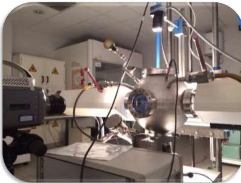
Figure 3-9 Experimental set-up for the particle size distribution measurement in the visualization 20L sphere using the laser diffraction sensor (D'Amico, 2016)
