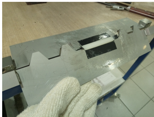
Figure 3.30 – Compression molding of polystyrene impact specimens.
