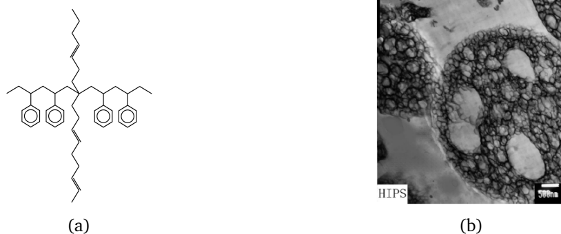
Figure 1.10 – HIPS: a) chemical structure and b) micrograph of the salami micro structure of commercial HIPS. Transmission electron micrograph, Gao et al., (2006), [54]
