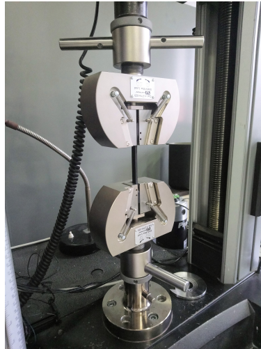
Figure 3.27 – Tensile strength testing
