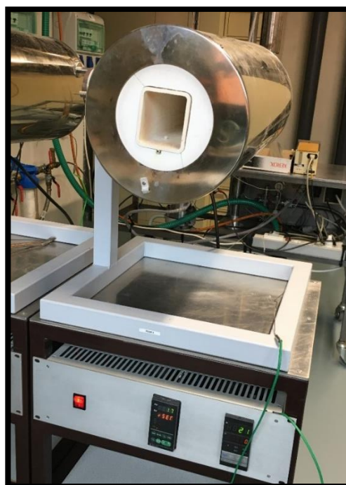
Figure 4.33: Horizontal heating furnace used for the process of saturation annealing.
