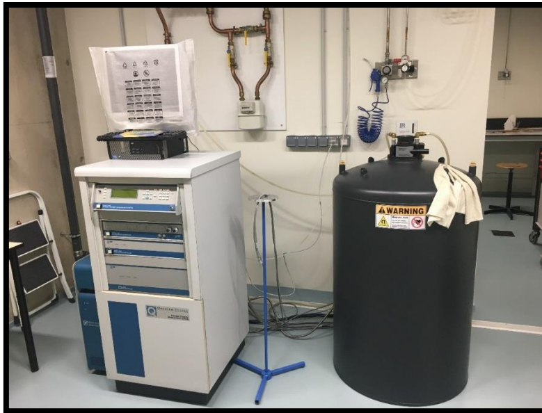
Figure C.1: Experimental setup of Quantum Design PPMS installed at IJL, Nancy.
