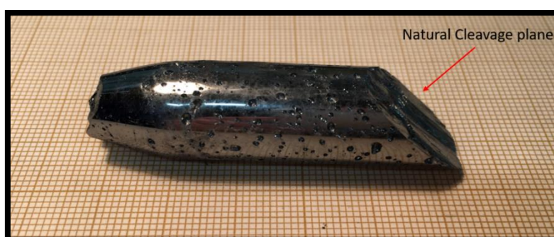
Figure 4.14: Grown InTe single crystal using the vertical Bridgman technique. The mirror-like cleavage plane is indicated. Note that the other side of the crystal was broken and does not correspond to a natural cleavage plane.
