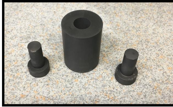
Figure 3.14: Graphite die and the pistons used for SPS process.
