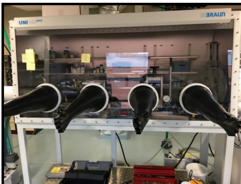
Figure 3.8: MBraun made Argon Glove box.
