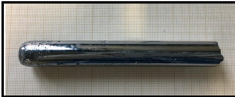
Figure 4.11: Prepared polycrystalline InTe ingot before introduction in the carefully-designed V-shaped-end silica tube for Bridgman-Stockbarger process.
