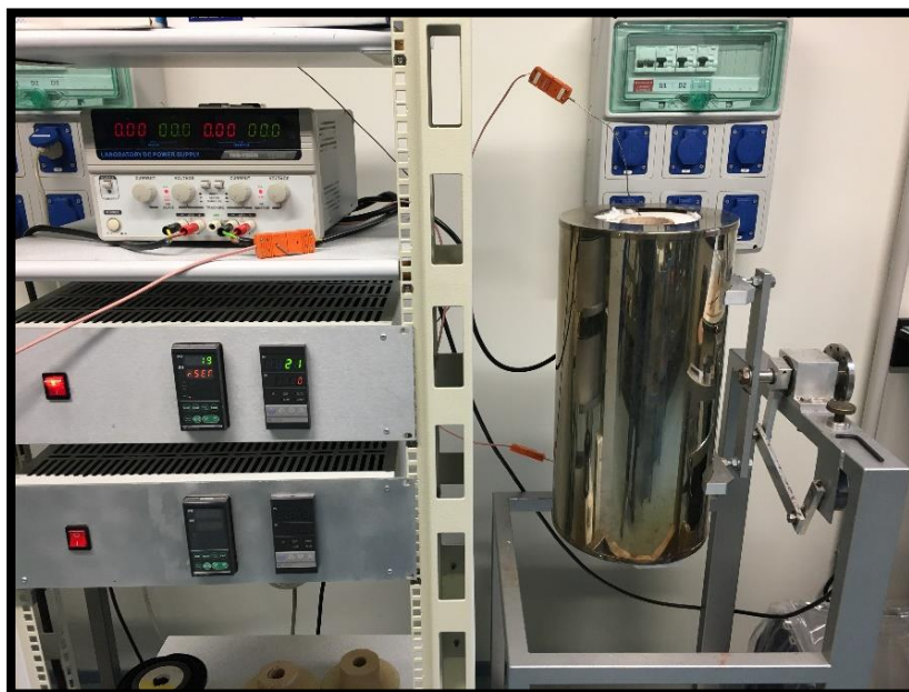
Figure 3.11: High-temperature vertical rocking furnace.
