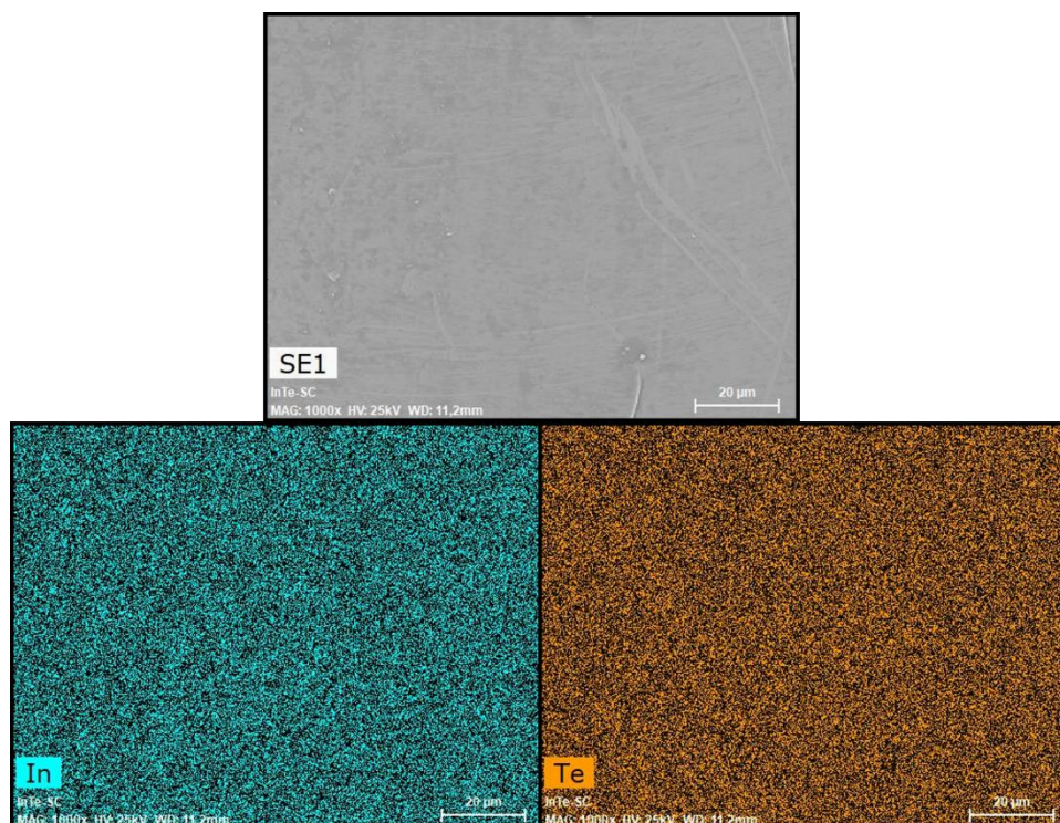
Figure 4.17: Elemental mapping for single crystalline InTe performed by SEM-EDXS analysis.
