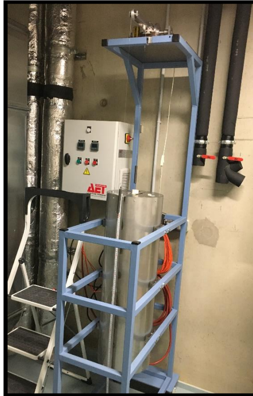
Figure 4.12: Two-zone vertical Bridgman furnace.
