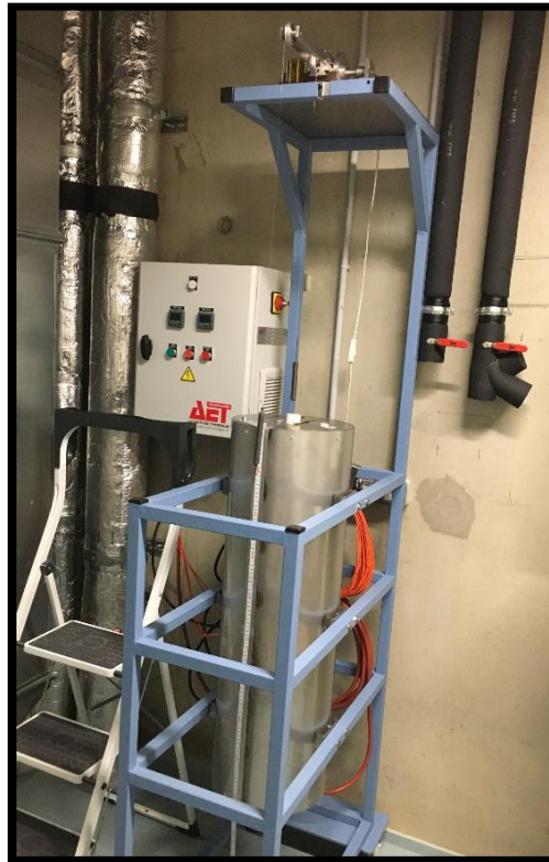
Figure 4.12: Two-zone vertical Bridgman furnace.
