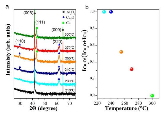
**Figure 3.8.** X-ray diffractograms  $Cu_2O$  and Cu films on sapphire substrates, showing the temperaturedependent selectivity (a). Evolution of the Cu and  $Cu_2O$  XRD intensity with deposition temperature (b).
