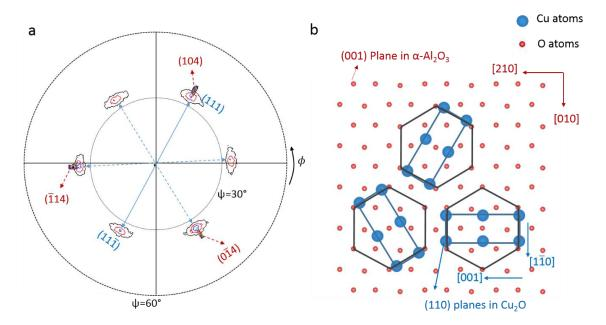
**Figure 3.9.** Pole figure of a Cu<sub>2</sub>O film deposited on  $\alpha$ -Al<sub>2</sub>O<sub>3</sub> at 2 $\theta$ =36.42°, the {111} and {104} family of planes for Cu<sub>2</sub>O and  $\alpha$ -Al<sub>2</sub>O<sub>3</sub>, respectively, are indicated (a). Schematic of the epitaxial relationship between the Cu<sub>2</sub>O films and the  $\alpha$ -Al<sub>2</sub>O<sub>3</sub> substrate, the different configuration, associated with the three Cu<sub>2</sub>O domains are indicated (b).
