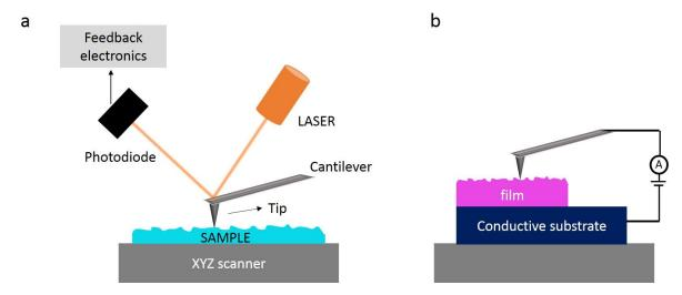
**Figure 2.26.** Schematic of the AFM system in contact mode (a). Schematic of one of the standard geometries for the C-AFM measurements.
