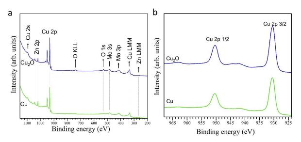
Figure 3.15. XPS survey scan (a) and Cu 2p spectra (b) for a Cu<sub>2</sub>O (blue) and a Cu (green) film.
