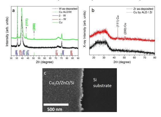
**Figure 3.18.** X-ray diffractometer of a Cu film deposited by ALD on a 200 nm W film (a) and on a 500 nm Zr film (b). Top view SEM micrograph for a Cu<sub>2</sub>O/ZnO/Si sample showing the area-selectivity of Cu<sub>2</sub>O on ZnO vs. Si substrates (c).
