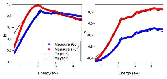
**Figure IV.** Measured and simulated ellipsometric spectra for the Cu/ZnO (10 000 ALD cycles) film at  $60^{\circ}$  (blue) and  $70^{\circ}$  (red).
