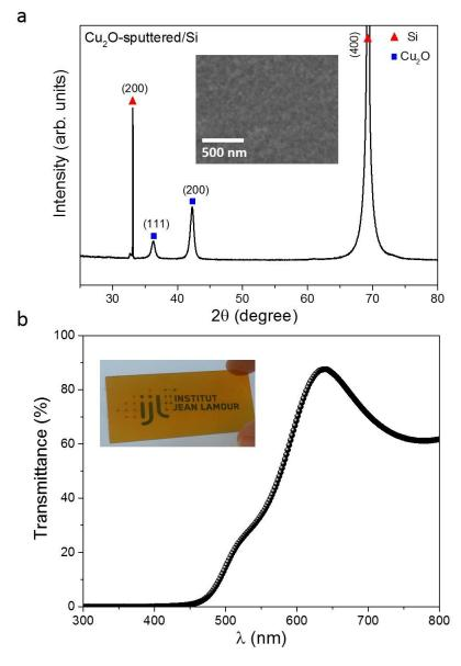
**Figure 5.11.** X-ray diffractogram of the  $Cu_2O$  film deposited on Si substrate (a), a top-view SEM micrograph is shown as inset. Transmittance spectrum of the  $Cu_2O$  film deposited on a glass substrate (b), a picture of the sample is shown as inset.
