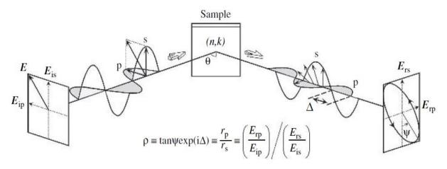
Figure 2.14. Configuration for spectroscopic ellipsometry measurements [143].
