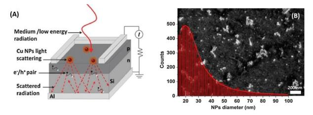
**Figure 1.14.** Schematic illustrating the light scattering in a Si solar cell due to the Cu nanoparticles at the surface (A). Top-view SEM micrograph of the devices showing the Cu nanoparticles at the surface (B) (modified from **[114]**).
