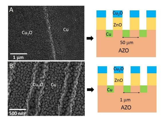
**Figure 3.21.**  $Cu_2O$  and Cu area-selective deposition on features of different sizes: 50 µm (a) and 1 µm (b).
