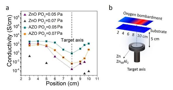
Figure 3.2. Conductivity of the ZnO and AZO films as a function of the position in the sputtering chamber and O<sub>2</sub> partial pressure (a). Schematic of the configuration used for the deposition and of the flux of high energetic O atoms and O<sup>-</sup> ions (b). Remark: the conductivity of sample deposited using  $P_{0_2} = 0.07$  Pa was too high to be measured near the target axis, explaining why symbols were selected instead of connecting lines in (a) for this condition.
