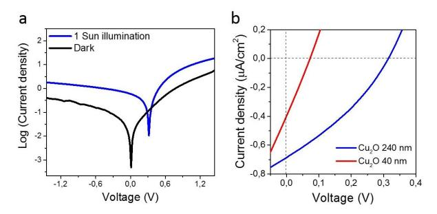
**Figure 5.13.** Current density characteristics of the heterojunction (in semi logarithmic scale) in dark (black line) and under 1 Sun illumination (blue line) (a). Current density characteristics amplified around the short-circuit current and open-circuit voltage points for the heterojunction with (blue line) and without (red line) the 240-nm-Cu<sub>2</sub>O sputtered layer (b).
