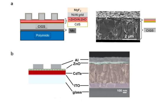
**Figure 1.7.** Schematic and cross-section SEM micrograph of a thin film CIGS solar cell on a flexible polyimide substrates, from **[74]** (a). Schematic and colored cross-section SEM micrograph of a CdTe solar cell, from **[75]** (b).
