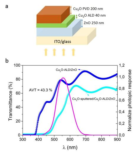
**Figure 5.12.** Schematic of the heterojunction with the addition of an uppermost  $Cu_2O$  layer growth by sputtering (a). Transmittance of the  $Cu_2O$ -ALD/ZnO (blue),  $Cu_2O$ -sputtered/ $Cu_2O$ -ALD/ZnO film (cyan) and the normalize photopic response of the human eye (violet) (b).
