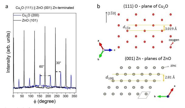
**Figure 3.13.**  $\phi$ -scan of the Cu<sub>2</sub>O (200) and the ZnO (101) crystallographic planes of the Cu<sub>2</sub>O-(111)/ZnO-(001)-Zn terminated sample, in logarithmic scale (a). Schematic of the oxygen atoms at the (111) planes of Cu<sub>2</sub>O (top) and the zinc atoms at the (001) plane in ZnO (bottom) (b).
