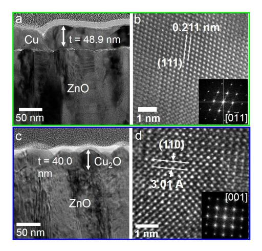
**Figure 3.4.** Cross-section TEM micrographs of the Cu (a) and the Cu<sub>2</sub>O (c) films. HRTEM micrographs of the Cu (b) and the Cu<sub>2</sub>O (d) films; the corresponding FFT patterns are shown at the inset.
