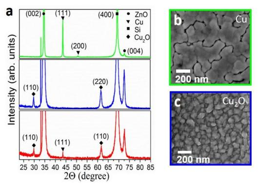
**Figure 3.3.** X - ray diffractograms of the samples after the ALD deposition at  $280^{\circ}$ C (a). Top-view SEM micrographs of the Cu film (b) and the Cu<sub>2</sub>O film (c).
