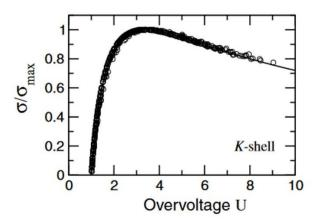
**Figure 2.19.** Normalized ionization cross-section of the K shell vs. overvoltage from **[146]**. The circle represent the DWBA calculation from several elements and the continuous line an analytical expression proposed by Campos *et al.*
