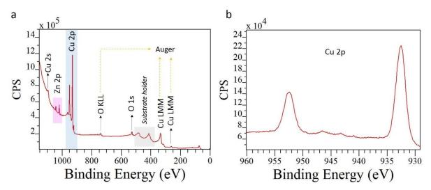
Figure 2.24. XPS survey spectrum (a) and Cu 2p spectra (b) from a Cu<sub>2</sub>O film.
