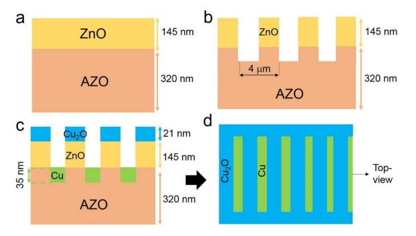
**Figure 3.19.** Schematic of the bilayer structure (a) as-deposited, (b) after etching, and after ALD deposition in (c) cross-section and (d) top-view.
