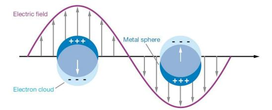
Figure 1.9. Schematic of localized surface plasmon resonance at the metallic nanoparticles [98].
