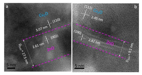
**Figure 5.17.** HR-TEM micrograph showing the orientation relationship between the  $Cu_2O$  and the ZnO nanowires.
