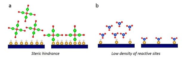
**Figure 2.3.** Simplified representation of the mechanism that lead to less than one monolayer deposition: steric hindrance (a) and low density of reactive sites (b).
