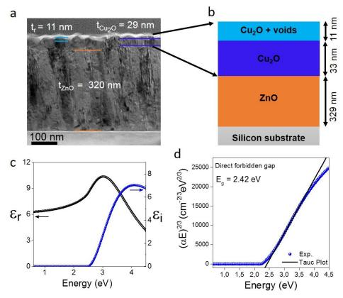
**Figure 5.5.** TEM micrograph of the  $Cu_2O/ZnO$  heterojunction (a). Schematic of the physical model used for fitting the ellipsometric data (b). Real and imaginary parts of the dielectric function of the  $Cu_2O$  film determined by ellipsometry (c). Tauc Plot for the  $Cu_2O$  film (d).
