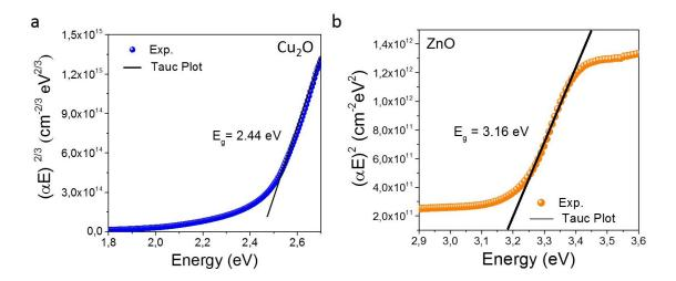
**Figure 5.7.** Tauc Plot for the Cu<sub>2</sub>O (a) and ZnO (b) films deposited on  $\alpha$ -Al<sub>2</sub>O<sub>3</sub>, and glass substrates, respectively.
