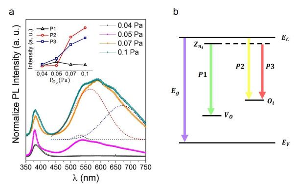
Figure 3.16. Normalized photoluminescence spectra of ZnO films deposited at different  $P_{0_2}$ , the evolution of the areal intensity of the defect bands with the oxygen partial pressure is presented at the inset (a). Energy level diagram illustrating the defect levels in ZnO and the transition observed in the photoluminescence spectra (b).
