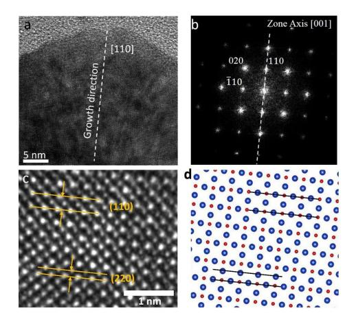
**Figure 5.3.** Cross-section HR-TEM micrograph of the  $Cu_2O$  film (a) with the corresponding FFT pattern (b). Amplified HR-TEM micrograph, the (110), and (220) planes are indicated (c). Schematic of the  $Cu_2O$  crystal structure (d).
