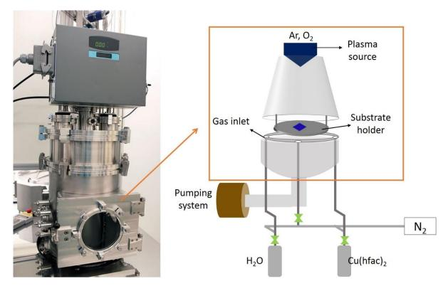
**Figure 2.6.** Picture of the ALD PICOSUN<sup>TM</sup> R-200 Advanced reactor (a). Simplified schematic of the ALD reactor, showing the reaction chamber, the plasma source at the top, and the precursor bottle and connections with the camber at the bottom (b).
