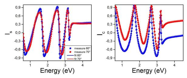
**Figure I.** Measured and simulated ellipsometric spectra for a typical ZnO substrate at  $60^{\circ}$  (blue) and  $70^{\circ}$  (red).
