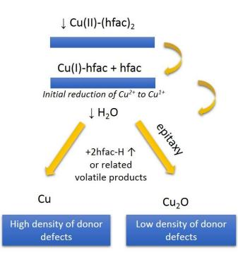
Figure 3.17. Schema illustrating the mechanism behind the selective deposition of Cu and Cu<sub>2</sub>O.
