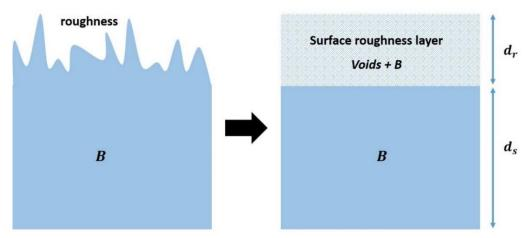
Figure 2.15. Schematic of the optical model employed to simulate the surface roughness (b).
