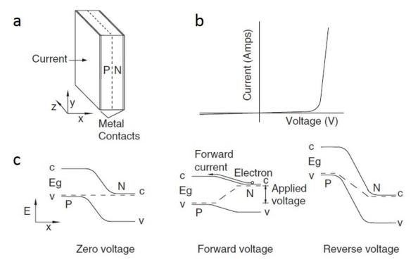
**Figure 2.27.** Schematic of a p-n junction (a). I-V characteristics of the junction (b). Energy diagrams diagrams for the different operation modes of the p-n junction: zero voltage (left), forward bias (center), reverse bias (right) (c) **[161]**.
