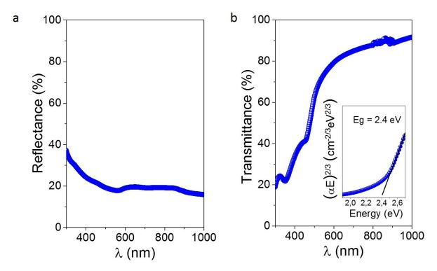
**Figure 2.13.** Reflectance (a) and transmittance (b) spectra of a Cu<sub>2</sub>O film deposited on  $\alpha$ -Al<sub>2</sub>O<sub>3</sub>. The Tauc Plot for this sample is presented as inset.
