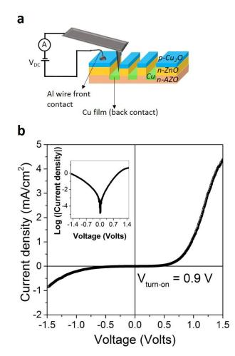
**Figure 3.23.** Schema of the sample configuration for the C-AFM measurements and the electrical contacts (a). Current density - voltage characteristics of the device in the dark at room temperature (b), the curve is also reported in semi-logarithmic scale as inset.
