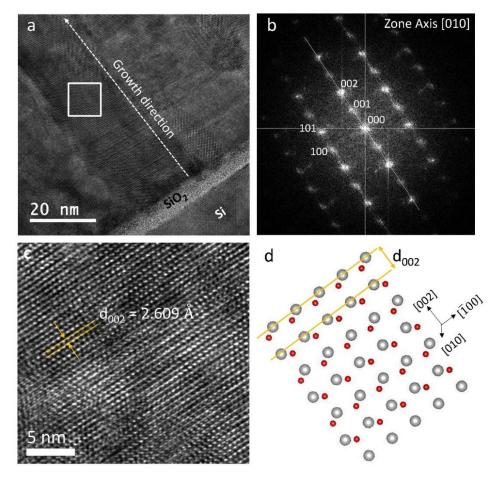
**Figure 5.2.** Cross-section HR-TEM micrograph of the ZnO film (a) with the corresponding FFT pattern (b). Amplified HR-TEM micrograph, the (002) planes are indicated (c). Schematic of the ZnO crystal structure, where the (002) planes are indicated (d).
