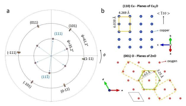
**Figure 3.12.** Pole figure of the Cu<sub>2</sub>O film deposited on ZnO at  $2\theta$ =36.42°, the {111} and {101} family of planes for Cu<sub>2</sub>O and ZnO, respectively, are observed (a). Schematic of the Cu atoms at the (110) planes of Cu<sub>2</sub>O (top), and the oxygen atoms at the (001) planes of ZnO (bottom). The different configuration in which the Cu<sub>2</sub>O domains can grow on top of the ZnO substrate (b).
