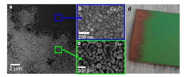
**Figure 3.6.** Top-view SEM micrographs of the sample composed of a mixture between Cu and Cu<sub>2</sub>O (a). Amplified micrograph at the Cu<sub>2</sub>O (b) and Cu (c) regions. Picture of the sample, where the interface between the Cu (orange) and the Cu<sub>2</sub>O (green) can be observed (d).
