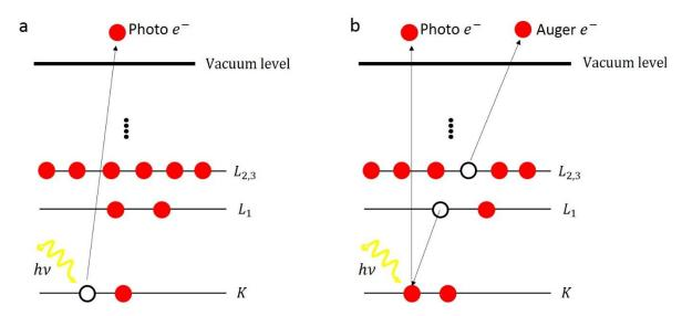
**Figure 2.23.** Schematic representation of photoelectron emission in XPS process (a) and Auger electron emission at result of relaxation process (b).
