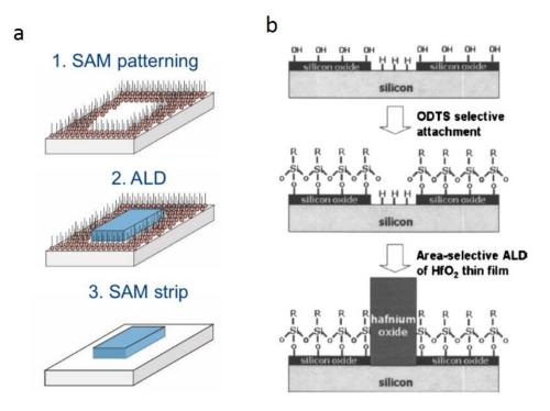
**Figure 3.1.** Schematic of the AS-ALD process by deactivation of the surface using SAMs [1] (a). Schematic of the AS-ALD process for the fabrication of HfO<sub>2</sub> using octadecyltrichlorosilanes (ODTS) SAMs to modify the surface [165].
