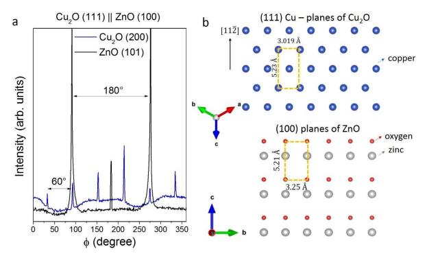
**Figure 3.14.**  $\phi$ -scan of the Cu<sub>2</sub>O (200) and the ZnO (101) crystallographic planes of the Cu<sub>2</sub>O-(111)/ZnO-(100) sample, in logarithmic scale (a). Schematic of the Cu atoms at the (111) planes of Cu<sub>2</sub>O (top) and the Zn atoms at the (100) plane in ZnO (bottom) (b).
