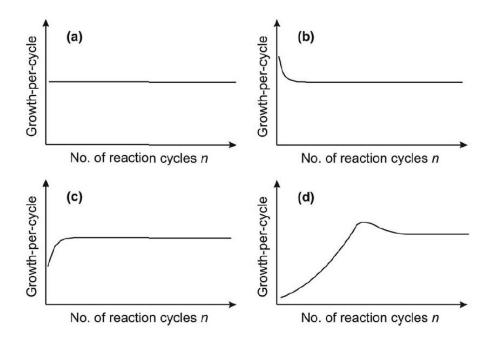
Figure 2.5. Evolution of the GPC with the number of ALD cycles. Linear growth (a), substrateenhanced growth (b), substrate-inhibited growth type I, and substrate-inhibited growth type II (d) [121].
