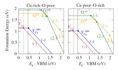
**Figure 1.3.** Theoretical calculations of the formation energy for the different acceptor levels in  $Cu_2O$ , under Cu-rich (left) and Cu-poor (right) conditions (color lines). The vertical dashed lines represent experimental values obtained from deep-level transient spectroscopy measurements [19].
