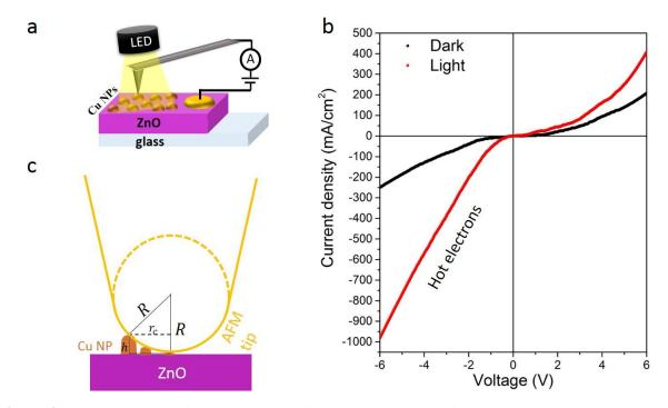
**Figure 4.7.** Photoresponse of Cu NP under visible light. Schematic of the C-AFM measurements (a). Current density characteristics of the Cu NP/ZnO device in the dark and under visible-light illumination, with an estimated contact area of  $4.3 \times 10^3$  nm<sup>2</sup> (b). Schematic of the contact area between the AFM tip and the sample surface (c).
