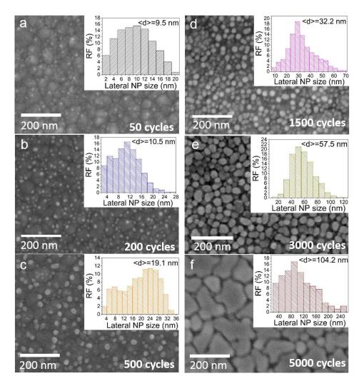
**Figure 4.1.** Top-view SEM micrographs of Cu NP at 50 (a), 200 (b), 500 (c), 1500 (d), 3000 (e), and 5000 (f) ALD cycles with the corresponding lateral NP size distributions in the inset (RF meaning relative frequency).
