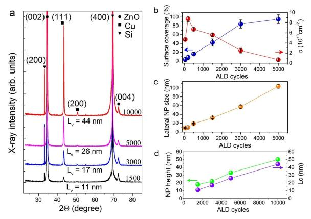
**Figure 4.2.** X-ray diffactrograms of the Cu NP after 1500 (black), 3000 (blue) and 5000 (magenta) ALD cycles and the Cu film (red) deposited at 10000 ALD cycles (a). Surface coverage, density (b) and average lateral NP size (c), versus the number of ALD cycles. Average NP height (green), and coherence length (violet), versus the number of ALD cycles (d).
