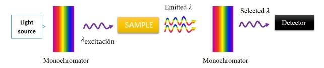
Figure 2.16. Schematic principle of the photoluminescence spectroscopy set-up.
