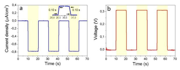
**Figure 5.14.** Current density (a) and voltage (b) versus time during multiples dark/light cycles of 20 seconds.
