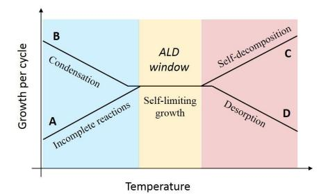
Figure 2.4. Schematic of ALD process, showing the GPC evolution versus substrate temperature.
