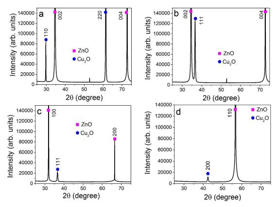
**Figure 3.10.** X-ray diffractograms of the Cu<sub>2</sub>O films deposited on c-plane oriented O-terminated ZnO (a), c-plane oriented Zn-terminated ZnO (b), a-plane ZnO (c), and m-plane ZnO (d) substrates.
