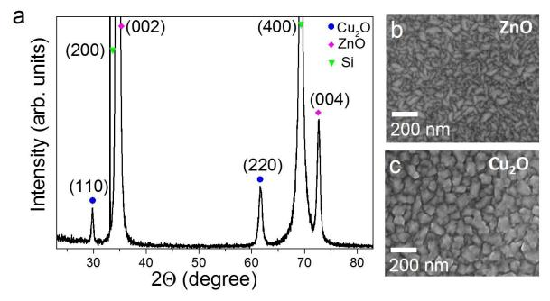
**Figure 5.1.** X-ray diffrcatogram of the  $Cu_2O/ZnO$  heterostructure (a). Top-view SEM micrograph of the as-grown ZnO film (b) and of the  $Cu_2O$  film deposited on top (c).
