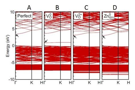
**Figure 1.5.** Band structure of a ZnO perfect crystal (A), and considering different types of defects: oxygen vacancies in the neutral state (B) and 2+ charge states (C), and Zn interstitial at the octahedral site in the neutral state [52].
