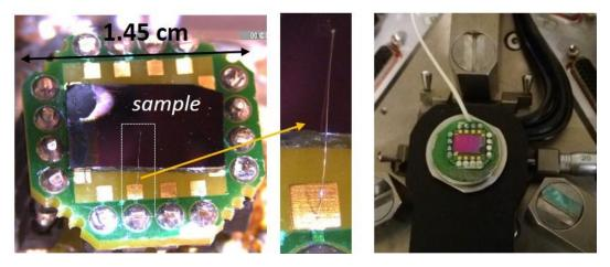
**Figure 3.22.** Picture of the chip used as substrate holder for the C-AFM measurements and the Al wire used as electrical contact on the  $Cu_2O$  film.
