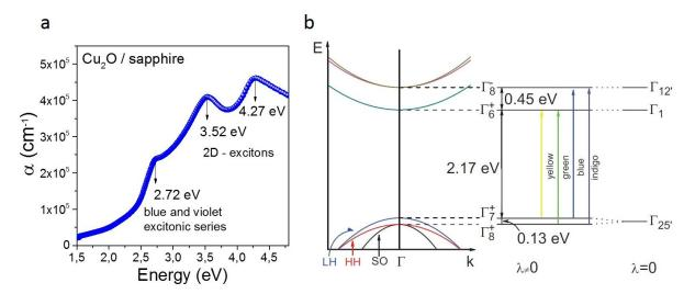
**Figure 5.6.** Absorption coefficient for the Cu<sub>2</sub>O film deposited on  $\alpha$ -Al<sub>2</sub>O<sub>3</sub> (a). Schematic of the Cu<sub>2</sub>O electronic band structure around the center of the Brillion zone ( $\Gamma$ -point), without ( $\lambda$ =0) and with ( $\lambda$ ≠0) spin-orbit interaction. Transition from the  $E_C$  to the  $E_V$  leads to the four excitonic series represented in color lines (b).
