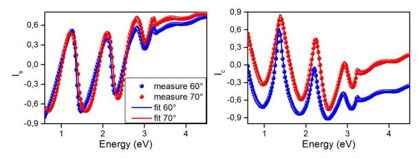
**Figure V.** Measured and simulated ellipsometric spectra for the Cu<sub>2</sub>O/ZnO films at  $60^{\circ}$  (blue) and  $70^{\circ}$  (red).
