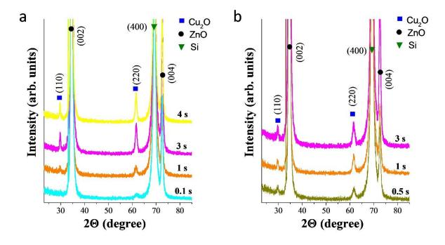
**Figure 2.7.** Optimization of the precursors pulse length:  $H_2O(a)$  and  $Cu(hfac)_2(b)$  for the deposition of  $Cu_2O$  on ZnO substrates. The substrate temperature and the number of cycles were fixed at 280 °C and 5000, respectively.
