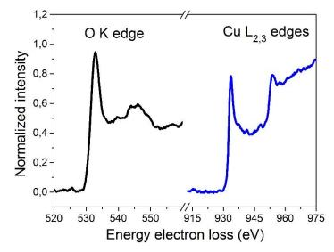
Figure 2.22. Typical EELS spectrum from a Cu<sub>2</sub>O film, at the high energy loss region.
