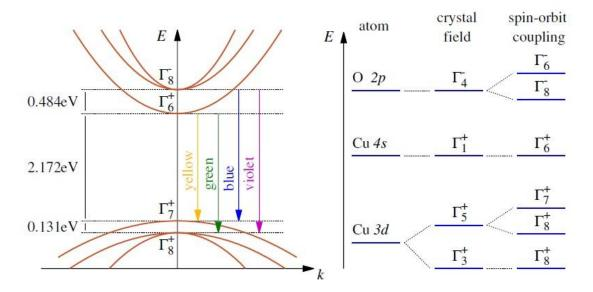
Figure 1.2. Schematic of the  $Cu_2O$  band structure at the  $\Gamma$ -point of the Brillouin zone, the different electronic transitions leading to the four excitonic series are indicated. Origin of conduction and valence bands from the atomic orbitals and the band splitting considering crystal-field and spin-orbit interaction are depicted on the right [17].
