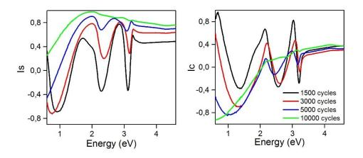
**Figure II.** Comparison of the ellipsometry measurements of the Cu nanoparticles/ZnO (1500, 3000 and 5000) and Cu film/ZnO (10000) at 70°.
