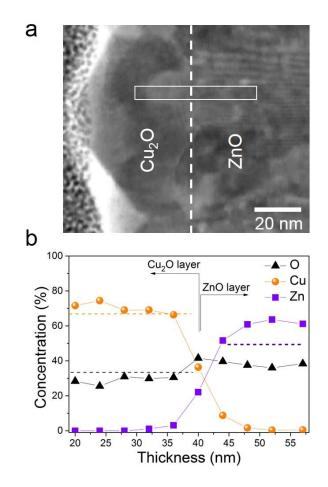
**Figure 5.4.** Bright field STEM micrograph taken at the interface between  $Cu_2O$  and ZnO films (a). Composition profiles obtained by EDS in the region enclosed by a rectangle in a (dashed lines indicate the expected Cu, Zn and O concentrations for the stoichiometric Cu<sub>2</sub>O and ZnO) (b).
