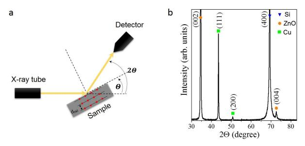
**Figure 2.12.** Schematic of the Bragg-Brentano geometry used in XRD (a). X-ray diffractogram of Cu/ZnO/Si sample (b).
