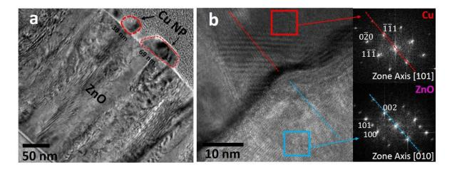
**Figure 4.3.** Bright-field-TEM micrograph of the CuNP/ZnO sample (a). High resolution TEM micrograph at the interface between the Cu NP and the ZnO film. FFT patterns taken at the Cu and ZnO regions are shown in the inset.
