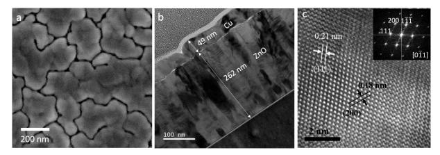
**Figure 4.4.** Top-view SEM micrographs of the Cu film after 10000 ALD cycles (a). TEM bright field micrograph taken from a cross-section of the Cu film (b). HRTEM micrograph taken to the Cu film (c) and the corresponding FFT pattern (inset).
