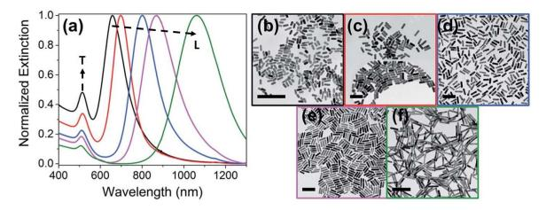
**Figure 1.12.** Evolution of the extinction spectra of Au nanorods by changing the aspect ratio. The longitudinal (L) and transverse (T) plasmon modes are indicated (modified from **[109]**).
