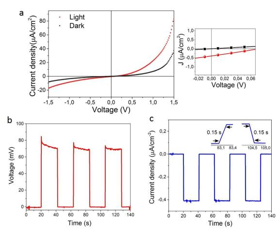
**Figure 5.9.** Current density characteristics of the Cu<sub>2</sub>O/ZnO heterojunction in the dark and under 1 Sun illumination (a). Voltage (b) and current density (c) versus time during multiples dark/light cycles of 20 seconds.
