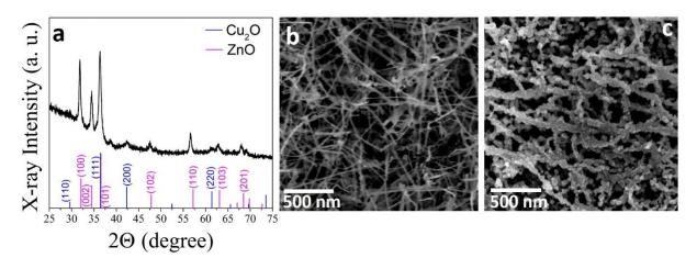
**Figure 5.15.** X-ray diffractogram of the Cu<sub>2</sub>O/ZnO nanowires (a). SEM micrograph of the ZnO before (b) and after the Cu<sub>2</sub>O deposition by ALD (c).
