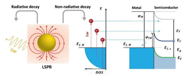
**Figure 1.13.** Schematic of the LSPR decay (left), and the hot-electron generation at the metallic nanoparticle and injection into the semiconductor (modified from **[3]**).
