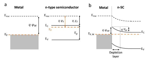
**Figure 1.16.** Band energy diagram of a metal and a n-type semiconductor, isolated (a) and when both materials are brought together, forming a Schottky junction (b).
