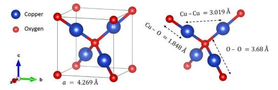
Figure 1.1. Crystal structure of cuprite Cu<sub>2</sub>O (space group Pn-3m). The bond lengths are indicated.
