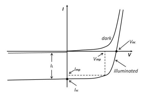
Figure 2.28. I-V characteristics of a p-Cu<sub>2</sub>O/n-ZnO heterojunction on dark and under 1 Sun illumination [162].
