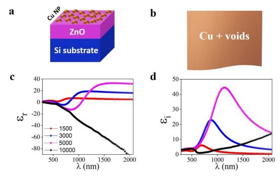
**Figure 4.5.** Schematic of the physical model used for fitting the ellipsometry data for the Cu NP (a) and the Cu film (b). Real (c) and imaginary (d) part of the dielectric function of the Cu NP and the Cu film (black line).
