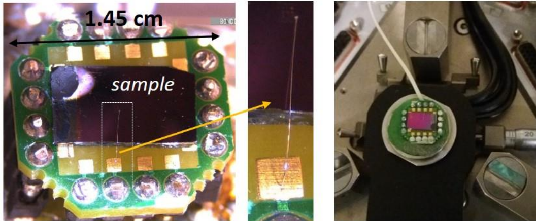
Figure 3.22. Picture of the chip used as substrate holder for the C-AFM measurements and the Al wire used as electrical contact on the \text{Cu}_2\text{O} film.
