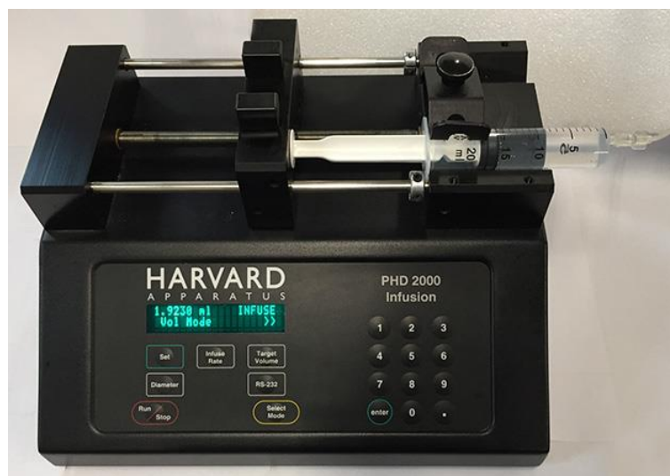
Fig. 2-3 Photograph of the syringe pump PHD 2000.
