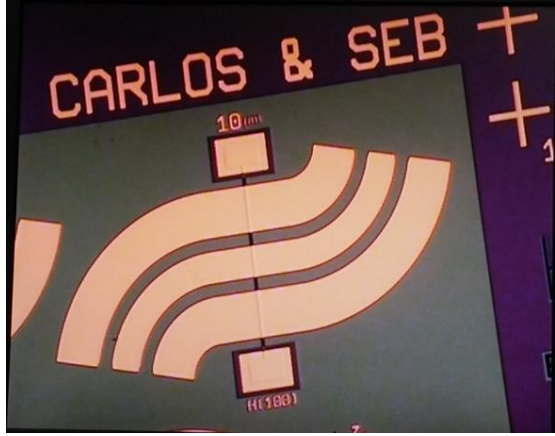
Figure II.12. (a) Picture of a SPFMR device which consists of a slab of the systems under study with an insulator cap and an antenna was deposited on top. (b) The same device with rf (GSG) and dc connections. The dc is to detect the spin pumping voltage, and rf to inject the rf current in the antenna. The dc field is applied along x-axis and perpendicular to the slab which is along y-axis as depicted in the figure.
