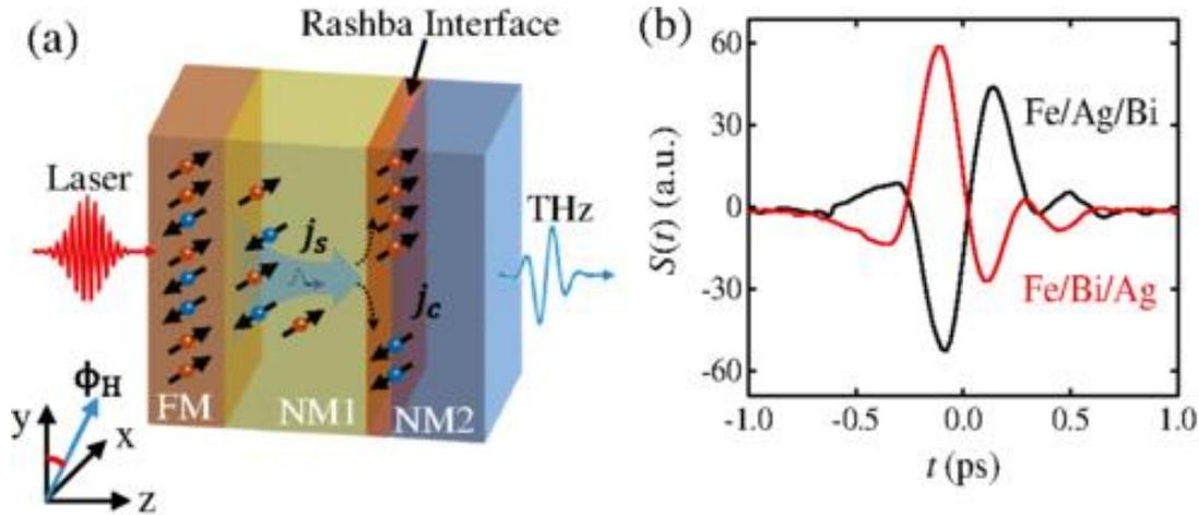
**Figure III.3** (a) Schematic of the THz emission experiment. An fs laser shines the sample on the FM side generating a spin current  $j_s$  which is converted in a transversal charge current  $j_c$  of THz range. (b) The THz emission on epitaxial Fe(2nm)/Ag(2nm)/Bi(3nm) and Fe(2nm)/Bi(3nm)/Ag(2nm) has opposite sign. Taken from [29]. In my opinion this is nice new evidence that supports the IEE scenario.
