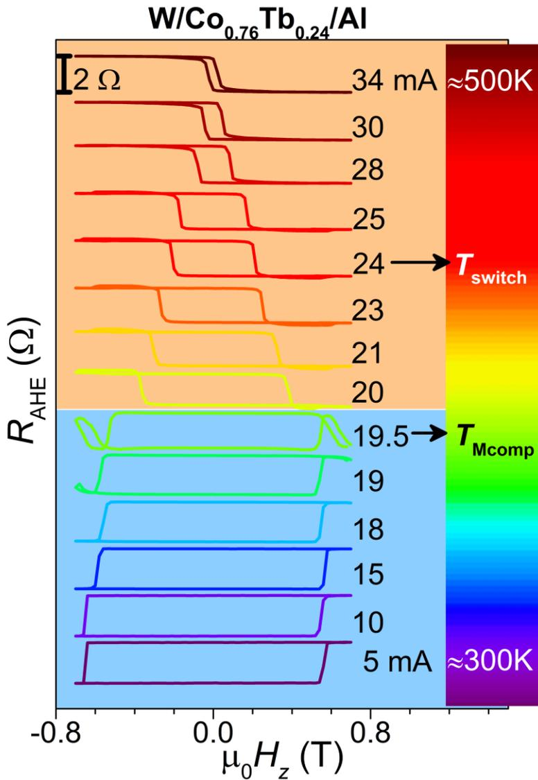
Figure V.7  $R_{\text{AHE}}(H_z)$  cycles with different pulse current intensities, instead of a small direct current of 0.4 mA. We can see that around 19.5 mA the cycle starts to change its sign. And already at 20 mA the cycle changed sign or polarity, that is, the device is above  $T_{\text{MC}}$ . In this sample, the switching current determined from the  $R(i)$  cycles is about 24 mA.
