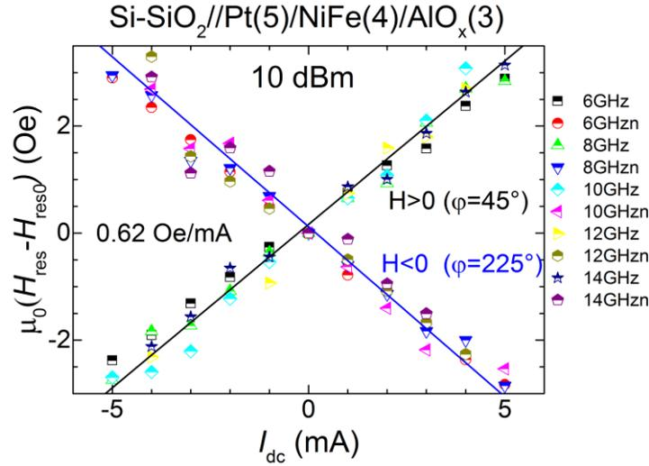
**Figure IV.6** Resonance field variation or shift of  $H_{res}$  as function of the total  $I_{dc}$  current added in the STFMR based experiment. The variation has a positive slop for positive filed, or  $\varphi=45^\circ$ , and negative slop upon reversal of in-plane magnetic field. All the frequencies has the same slope. The linear fit yield 0.62 Oe/mA. Considering  $h_{Oe}=\pm$ , then  $h_{FL}=\pm$  following the eq. (4.11). *Unpublished.*
