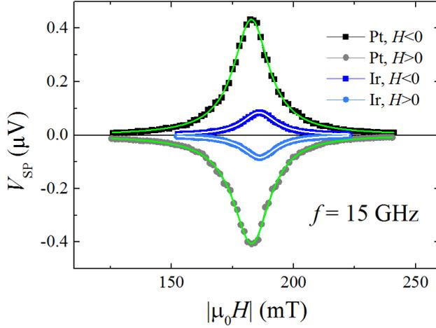
Figure II.13. Raw data SPFMR voltage in  $\text{SiO}_2//\text{CoFeB}/\text{Ir}$  and  $\text{SiO}_2//\text{CoFeB}/\text{Pt}$ . We can observe that the signal is symmetric around resonance field, and both systems exhibit the same sign, that is Pt and Ir have the same sign of spin hall angle.
