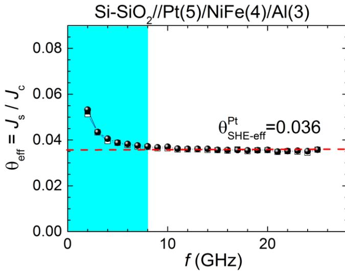
**Figure IV.3** Estimation of effective spin Hall angle of Pt in Pt/NiFe sample using the lineshape analysis given by the eq. (4.2). We can see that for frequencies  $f < 8\text{GHz}$  (light blue shaded area), the value is not constant and consequently not reliable. *Unpublished.*
