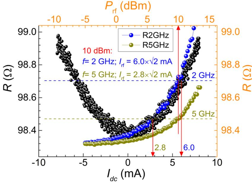
Figure IV.4 Example of the calibration of the  $I_{rf}$  current at a certain frequency and power by taking advantage of the variation of the resistance with the  $I_{dc}$  current due to the Joule heating effect. In the example we see that for an injected rf power of 10 dBm the current  $I_{rf} = 6.0\sqrt{2} = 8.5$  mA for 2 GHz and  $I_{rf} = 2.8\sqrt{2} = 3.9$  mA for  $f=5$  GHz.
