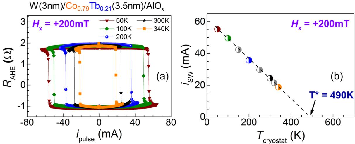
**Figure V.8** SOT-switching temperature dependency. (a) Switching cycles with current at different cryostat temperatures. (b) Extraction of switching current as a function of  $T_{\text{cryostat}}$ . We see a linear dependence that extrapolated to  $i_{\text{sw}}=0$  produces  $T^*=490\text{K}$ .
