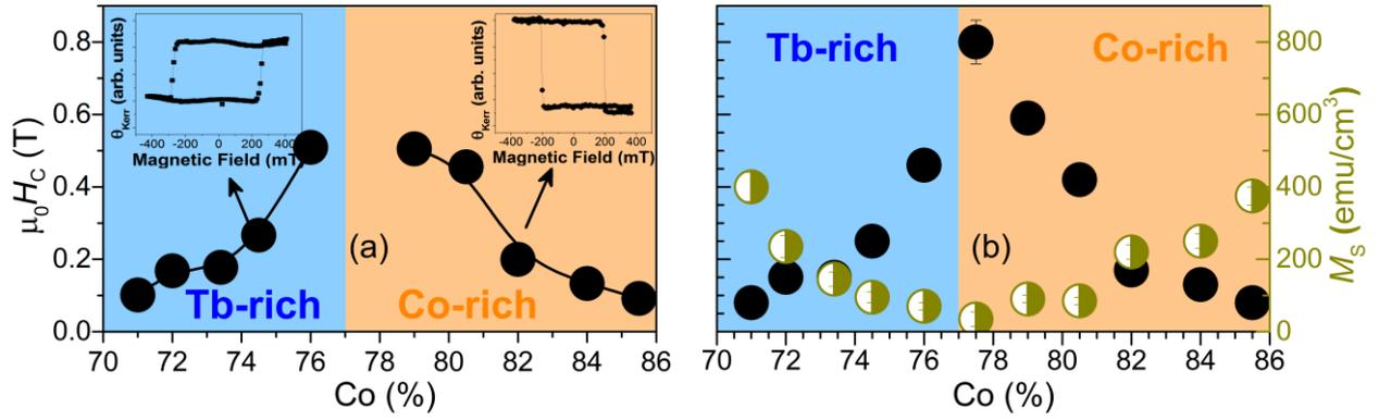
**Figure V.3** Magnetic characterization of W/CoTb/Al systems at 300 K. Coercitive field (a-b) and net magnetic saturation (b) as function of Co concentration.  $H_c$  from Kerr cycles (a), and  $M(H)$  cycles in SQUID-VSM (b). The insets in (a) are Kerr cycles for the indicated concentration. We see that  $H_c$  diverges and net  $M$  tends to zero at the magnetic compensation point. Adapted from [228].
