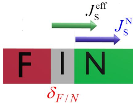
**Figure II.9.** Overview of the model used to describe that the interfaces are not transparent to spin injection. Within an FM/NM bilayer it is considered an I interface, and is analyzed as a fictitious FM/I/NM three-layer (FIN in the scheme). So the current that actually reaches the NM layer is an effective current after "losing" something in the interface and that also takes into account the back flow.
