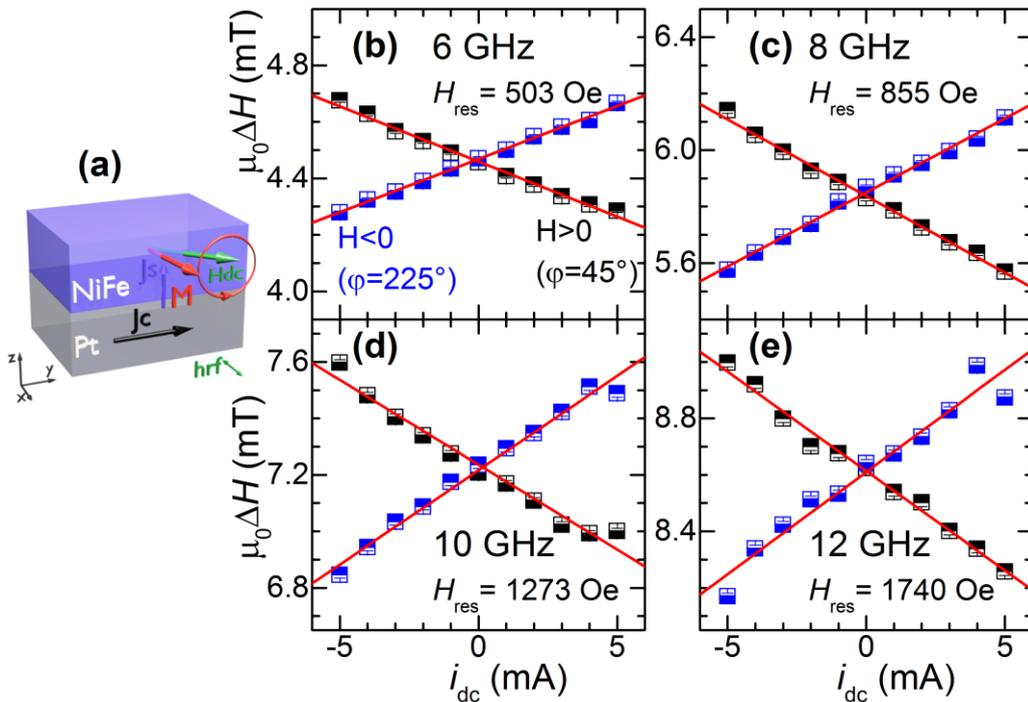
**Figure IV.5** Variation of NiFe linewidth vs. total current  $I_{\text{dc}}$  added in the STFM experiment at different frequencies between 6 and 12 GHz. The analysis, eq. (4.10), yield an average
