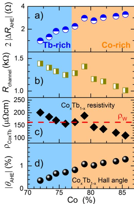
Figure V.5  $\text{W}(3)/\text{Co}_x\text{Tb}_{1-x}(3.5)/\text{AlOx}(3)$  composition dependence of AHE amplitude (a), longitudinal channel resistance in the Hall bar (b), CoTb resistivity (c), and Hall angle (d). Note that according to our convention,  $\Delta R_{\text{AHE}} > 0$  ( $< 0$ ) for Tb-rich (Co-rich). The dashed red line in (c) stands for the W resistivity.
