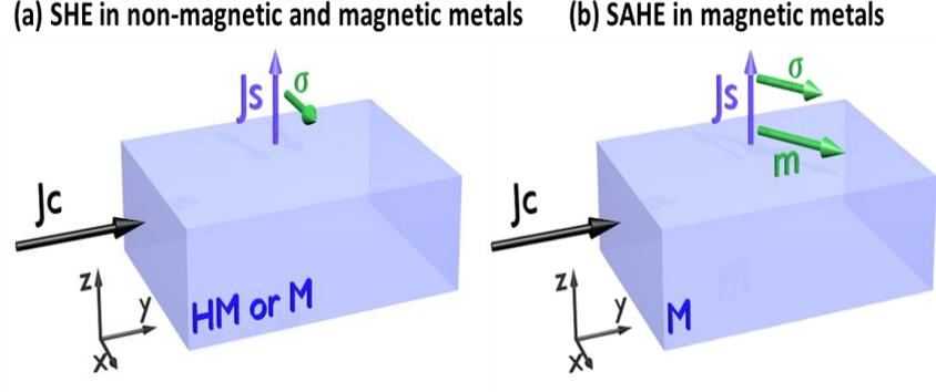
**Figure VI.1 Schematic of SHE and SAHE.** (a) In the SHE symmetry the spin current  $J_s$  along  $z$  has a spin polarization  $\sigma$  perpendicular to both,  $J_s$  and  $J_c$ ,  $J_s \propto \theta_{\text{SHE}} (\mathbf{J}_c \times \sigma)$ . (b) In the SAHE symmetry the spin current  $J_s$  along  $z$  has a spin polarization  $\sigma$  parallel (or antiparallel) to magnetization  $m$ ,  $J_s \propto \theta_{\text{SAHE}} (\mathbf{J}_c \times \mathbf{m})$ .
