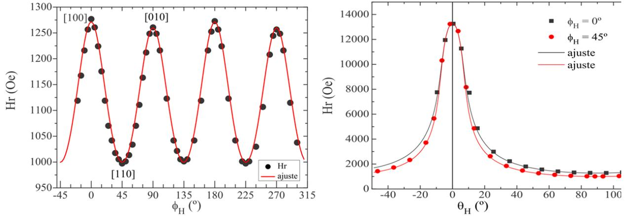
**Figure II.6.** IP (a) and OOP (b) angular dependence of resonance field at 150 K on a LSMO(60 nm) film performed using a X-band resonance cavity ( $f \sim 9.6$  GHz). Data points are experimental values and lines are numerical fits using eq. (2.3) and (2.5). In square brackets are shown the corresponding crystalline axes in (a). Two perpendicular plane to the film were carried out to get the data points in (b).
