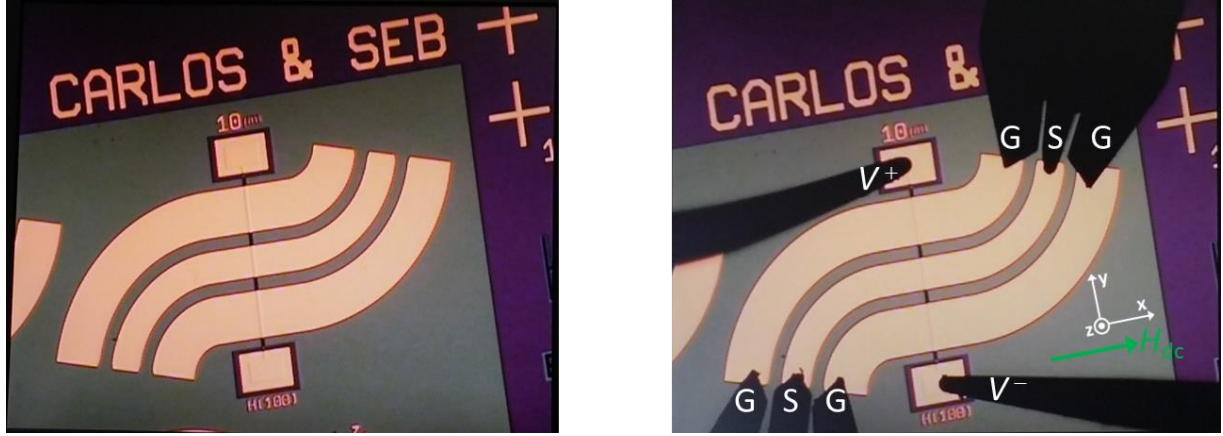
Figure II.12. (a) Picture of a SPFMR device which consists of a slab of the systems under study with an insulator cap and an antenna was deposited on top. (b) The same device with rf (GSG) and dc connections. The dc is to detect the spin pumping voltage, and rf to inject the rf current in the antenna. The dc field is applied along x-axis and perpendicular to the slab which is along y-axis as depicted in the figure.
