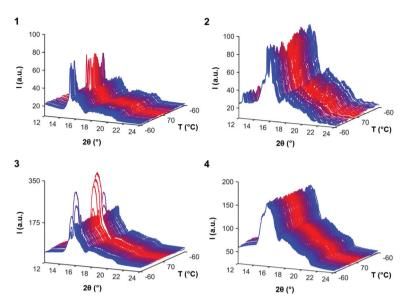
Fig. 5 Variable temperature WAXS analysis of SPUs 1-4. The samples were heated at 5 °C min<sup>-1</sup> between -60 °C and 70 °C over three cycles.
