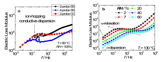
**Figure 2.** Electric loss modulus of Nafion using three different electrodes setup: 2-probe SS; 4-probe SS; and 2-probe CC (**a**). Electric loss modulus of Nafion with decreasing relative humidity using 2-probe CC (**b**).
