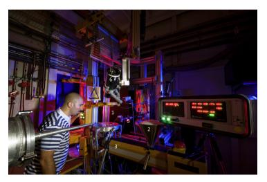
**Fig. 6.** Film blowing unit installed on beamline BM26A at the ESRF [56]. 1-blown film, 2-fedding hopper, 3-extruder, 4-film blow die, 5-X-ray beam, 6-WAXS detector, 7-SAXS detector. This set-up was used to collect data on the structural evolution of LLDPE [55,57]. With the appropriate infrastructure in place this type of sample environment can be installed in a couple of hours.
