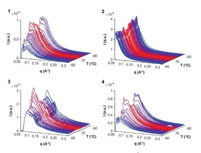
Fig. 3 Variable temperature SAXS analysis of 1–4. The samples were heated at 5 °C min<sup>-1</sup> between -60 °C (nearest) and 70 °C before cooling to -60 °C (furthest).
