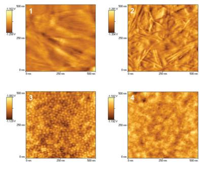
Fig. 6 AFM phase micrographs of DBDI based SPUs 1–4.
