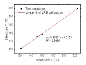
Figure 3.4. Calibration curve obtained under the simultaneous influence of both X-ray beam and Raman laser (785 nm) measured by the Linkam DSC-stage.
