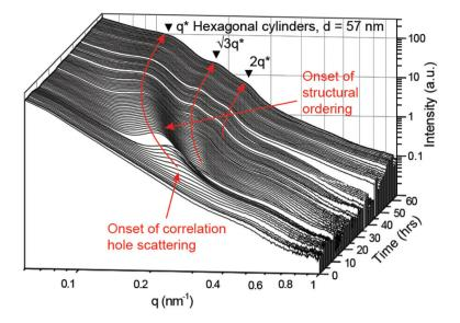
Fig. 1 Time-resolved *in situ* SAXS data collected during the chain extension of PMMA(31) to form PMMA(31)-PS(25) (experiment 5) *via* dispersion polymerisation in scCO<sub>2</sub>. The time between the individual profiles included is approximately 30 minutes.
