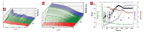
**Fig. 8.** In situ GIWAXS (a) and GISAXS (b) of pDPP and PC<sub>71</sub>BM blends processed from a DCB:CF solvent mixture. (c) Summary of the in-situ GIWAXS and GISAXS results during solvent evaporation. Adapted with permission from [90].
