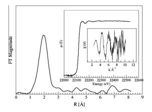
**Fig. 11.** An X-ray Absorption Spectroscopy scan from a Ruthenium containing soft condensed matter sample. This kind of data can be used to shine light on the coordination of metallic complexes with the surrounding organic medium. The graph shows the data and the inset the derived data. These experiments using reasonable time scales and X-ray doses were hardly feasible 10 years ago but have moved into the realm of reality in the last number of years.
