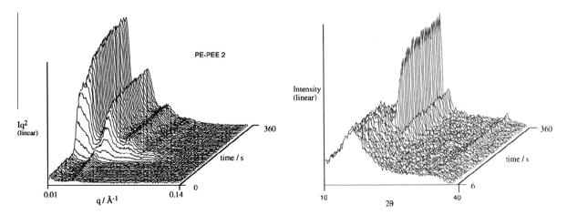
**Fig. 1.** Time-resolved SAXS (left panel) and WAXS (right panel) patterns obtained in a combined experiment where the PE-PEE diblock copolymers were cooled from the melt [14]. Even though the detectors and X-ray intensity in this experiment from 1995 were not of the same quality/intensity as is available at present high data quality could be achieved in time frames of 1–5 s/frame (reproduced with permission).
