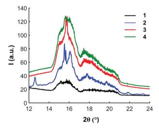
Fig. 4 Comparison of WAXS profiles for DBDI-based SPUs (1-4).
