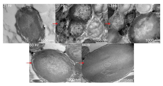
Fig. 4 TEM images of representative cross-sectioned PMMA-*b*-PS particles taken from the kinetic aliquots of the offline chain extension of PMMA(25) with PS(50) at time points of 21, 37, 53, 60 and 84 hours.
