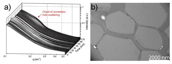
**Fig. 5** (a) Time-resolved *in situ* SAXS data recorded during the chain extension of PMMA(58) to form PMMA(58)-PS(12) *via* dispersion polymerisation in scCO<sub>2</sub>. The time between the individual profiles included is approximately 30 minutes. (b) TEM images taken of the final product.
