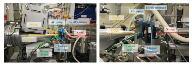
Figure 3.1. Simultaneous SAXS/WAXS combined to both Linkam DSC and Raman spectroscopy setup at DUBBLE (BM26b, ESRF) (A) and a magnification of the sample environment (B).
