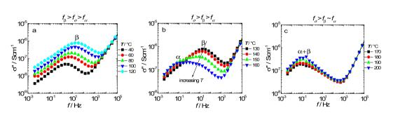
**Figure 3.** Imaginary component of the proton conductivity as a function of frequency in three temperature ranges: (**a**) from 40 to 120 °C; (**b**) from 130 to 160 °C; and (**c**) from 170 to 200 °C.
