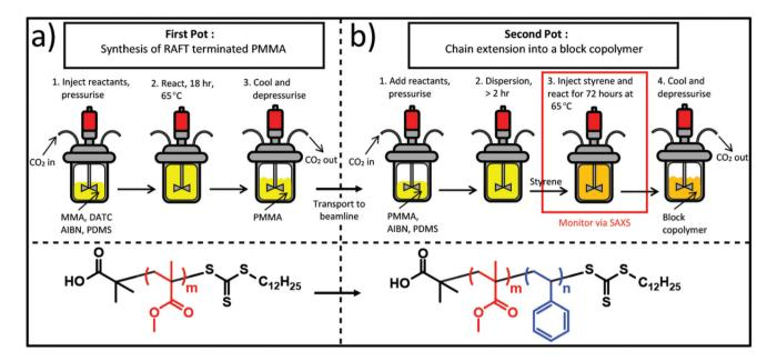
Scheme 1 The "two pot" synthesis method used to prepare the block copolymers monitored *via* time resolved SAXS. (a) Preparation of PMMA particles *via* dispersion polymerisation and (b) PMMA particle redispersion with additional PDMS-MA stabiliser and subsequent chain extension with styrene at the beamline.
