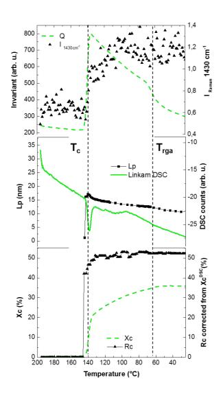
Figure 3.7. Porod's invariant, crystallinity (Xc) and long period evolution as a function of temperature during crystallization from the melt (200 °C) of PVDF sample. The dash line ( $\approx$  145 °C) indicates the crystallization transition (T<sub>c</sub>) and the dash line ( $\approx$  70 °C) the transition of the rigid amorphous compaction (T<sub>rga</sub>).
