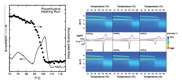
**Fig. 4.** Combined X-ray scattering and thermal analysis data. The left hand panel shows the slow cooling and crystallization from a polyethylene sample [16] obtained around 1985. The right hand panel shows a similar experiment [20] using a flash DSC, well collimated beamline and efficient photon counting detectors performed in 2015. The differences in data quality are clearly visible.
