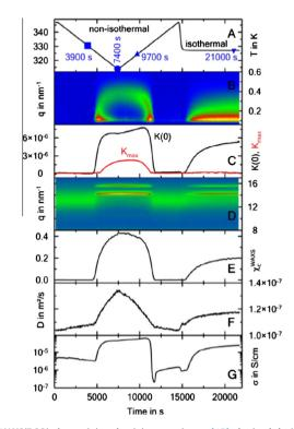
**Fig. 3.** Derived parameters from a SAXS/WAXS/DSC/calometric/conductivity experiment [15] obtained during thermal treatments of a polymer sample doped with Multi Walled Carbon Nano Tubes. (A) Thermal profile, (B) raw data, (C) derived electron density data (SAXS), (D) Raw WAXS data, (E) degree of crystallinity derived from WAXS data, (F) thermal diffusivity, (G) electrical conductivity. Data obtained with modern detectors and sample environments.
