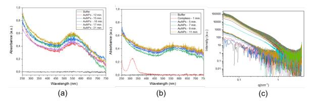
Figure 6.4 a) Uv-Vis absorption spectra of a solution mixture of HAuCl<sub>4</sub> and HEPES with different times ([AuP = 0.45 mM, H2O]/ ([B1 HEPES = 2.5 mM, D2O]). b) UV-vis absorption spectra of a solution mixture of HAuCl<sub>4</sub> and HEPES with different times ([AuP = 0.45 mM, D2O])/ (B2 [HEPES = 2.5 mM, D2O]). c) SAXS experimental data of the nucleation and growth mechanisms of a solution mixture of HAuCl<sub>4</sub> and HEPES ([AuP = 0.45 mM, D2O])/ ([B1 HEPES = 2.5 mM, H2O])/
