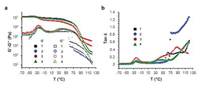
Fig. 7 (a) Thermal dependence of dynamic shear moduli for DBDI derived polymers 1–4. (b) Plot of tan  $\delta$  versus temperature for DBDI based SPUs 1–4.
