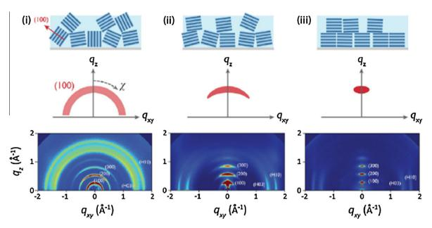
**Fig. 7.** Overview of the structural information that can be extracted from GIWAXS images. (i) Random crystallites orientation; (ii) crystallites with partial orientation; (iii) crystallites highly oriented with the (0 0 1) plane parallel to the substrate. Reprint with permission from [88].
