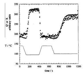
**Fig. 2.** The derived data obtained from the SAXS and WAXS raw data shown in Fig. 1. The scattering invariant  $Q = \int_0^{\infty} q^2 I(q) dq$  (open symbols) and the integrated intensity of the WAXS (1 1 0) peak (closed symbols) are given as function of time and temperature. The data quality is remarkably good even though the WAXS data is intrinsically more noisy than the SAXS data.
