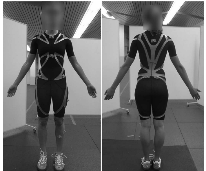
Figure 1 — Participant wearing the customized full-body compression suit (FBCS) with 2x thermoplastic polyurethane layers (TPU). The FBCS design provides support for the trunk over the pelvis segment through the 2x TPU layers that link the upper body with lower limbs across the pelvis in the back (right). The customized apparel production ensures a perfect fitting for each participant.
