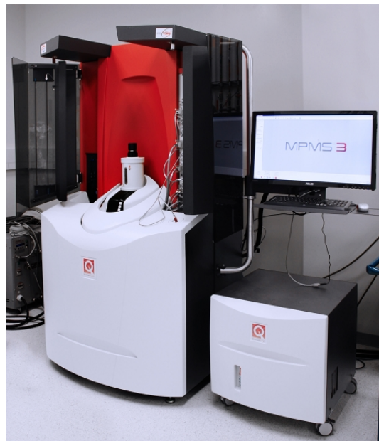
Figure 2.2: MPMS SQUID VSM from Quantum Design
