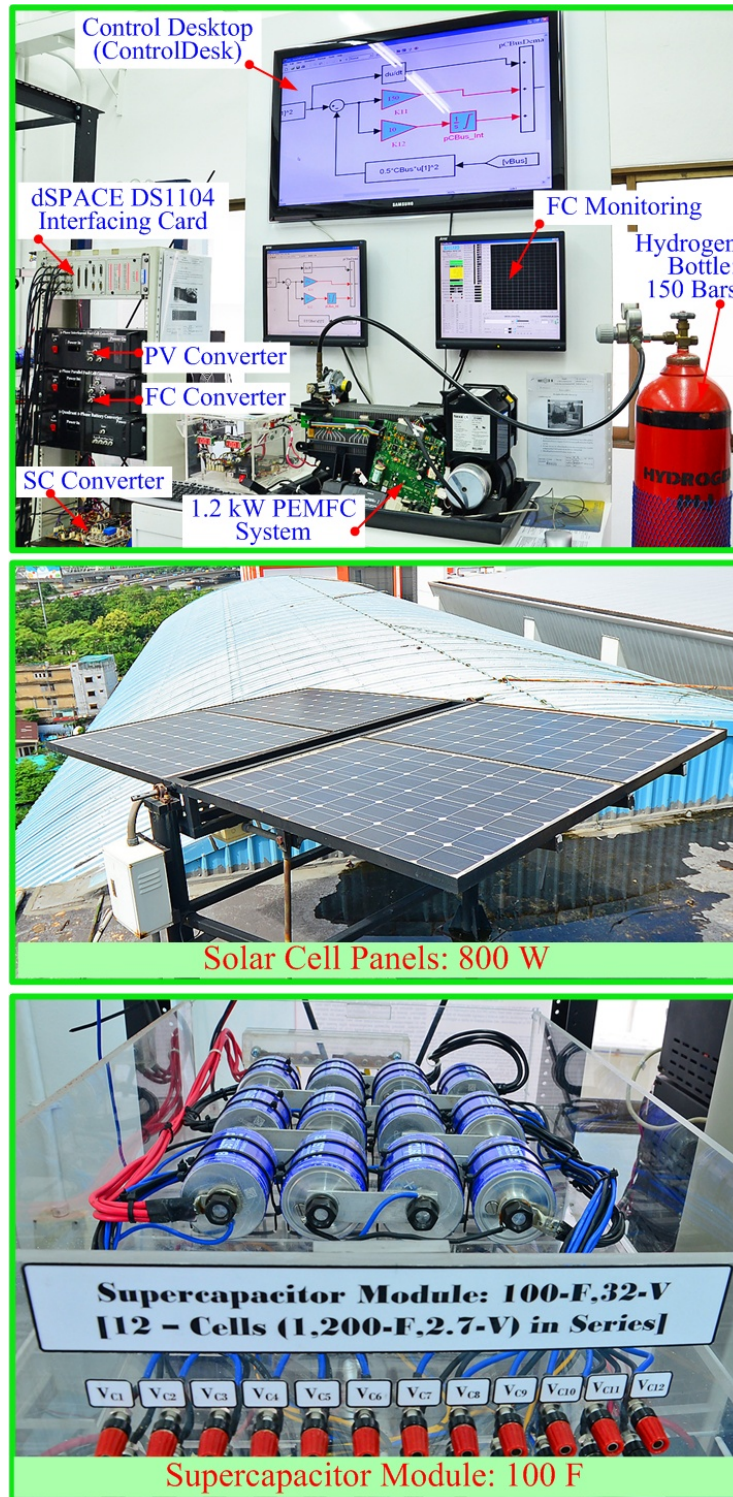
Fig. II.3.63. Photograph of the experimental setup at the Renewable Energy Research Centre (RERC), Bangkok.
