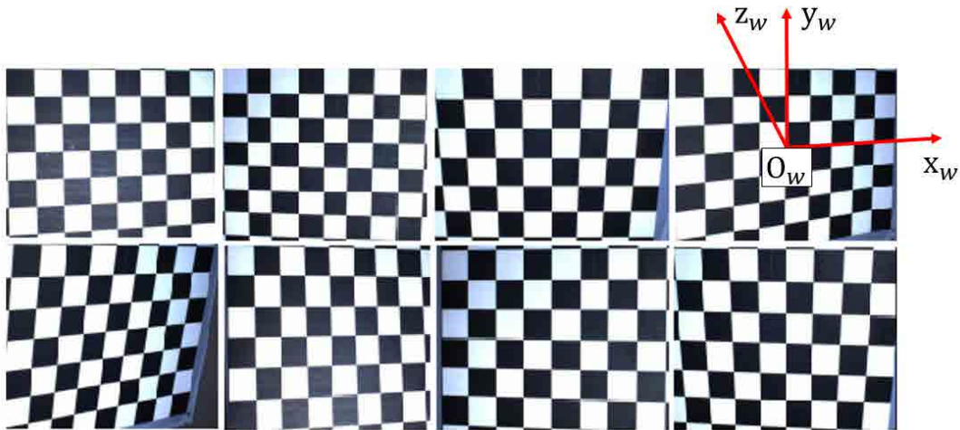
Figure 2.4: Calibration pattern acquired from various viewpoints. For the state-of-the-art method of Zhang, it is recommended to take numerous (at least 10-15) images from very different camera distances and orientations. Tests performed in the frame of this thesis have shown that a significant variation of the camera orientation is of particular importance to ensure an accurate calibration with Zhang’s approach.
